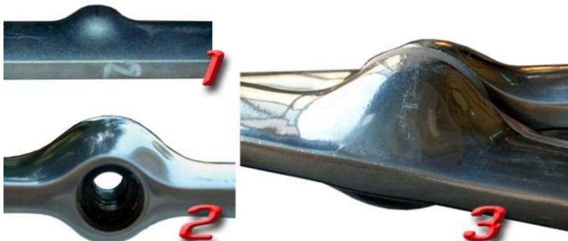
[image 1] Chronological sequence of cap's transformation; prototype 1 was made using bleu plastic chair's drawings; prototype 2 was rejected because it did not respect designer's guidelines; prototype 3 is the one that took us to the chair's realization.
