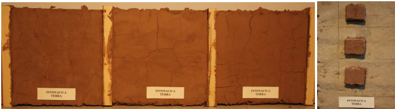
Fig. 1 – Type of specimens: size 25x25 cm and 5 x 4 cm on the wall; thick of specimens about 2 cm.
