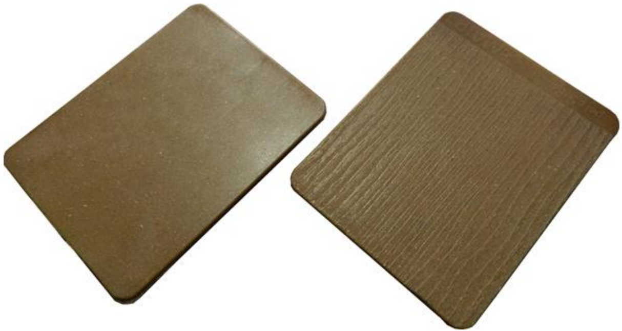
Aesthetic samples PP / 35% bamboo fibers (Francesca Griotti, 04/09/2013)
