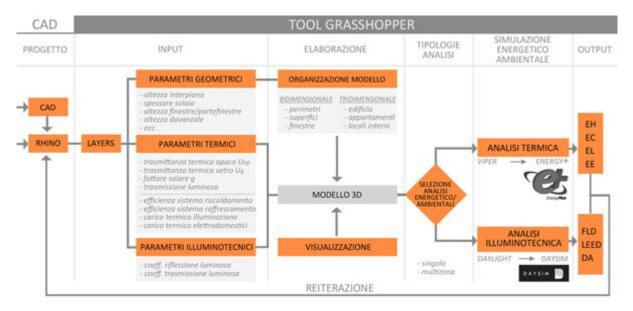
Flowchart visualizing the use of the Tool and its connection with Rhinoceros and with the energy simulation process (Energy Plus and Daysim)
