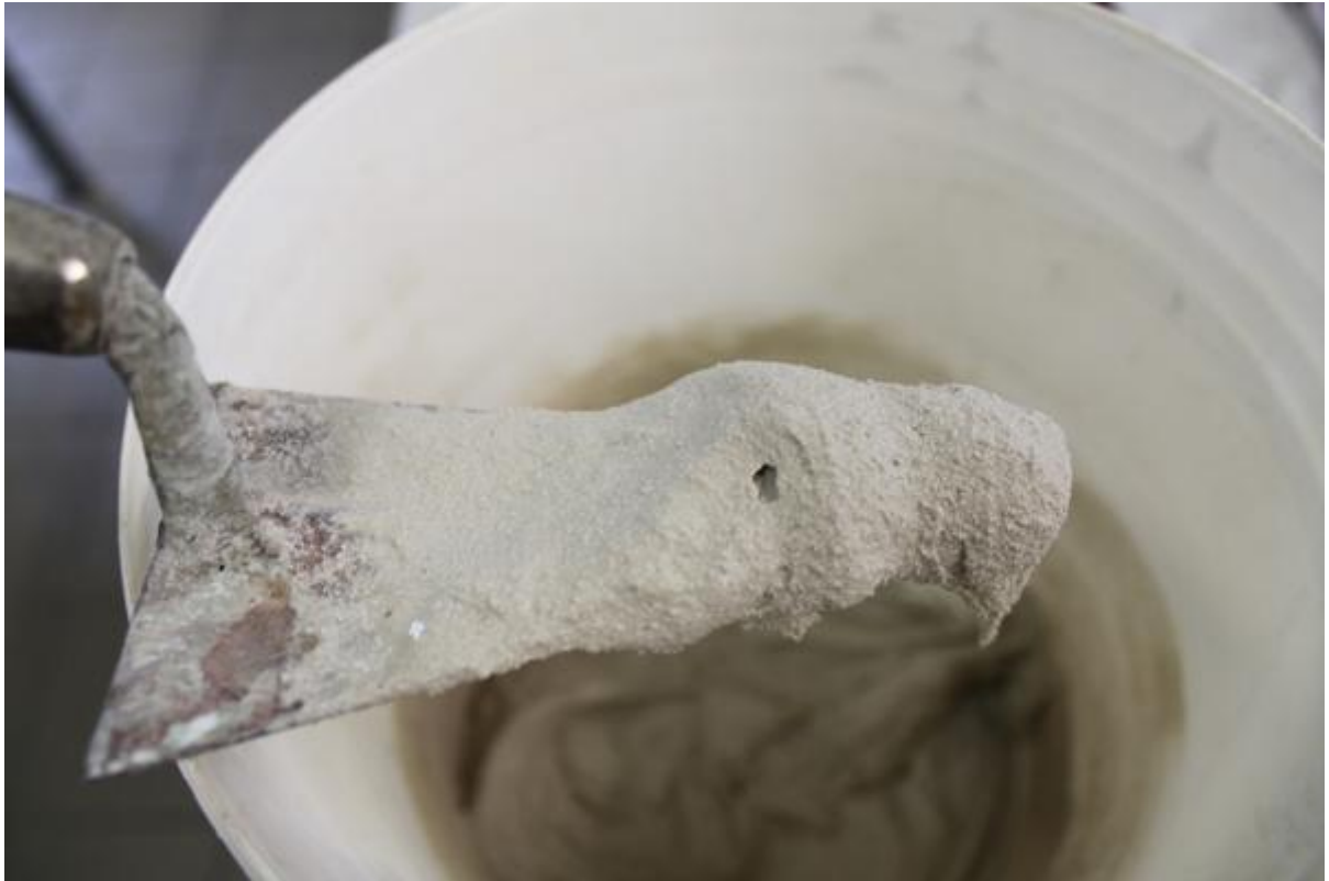
Finishing based on PCM: mixing tests in laboratory
