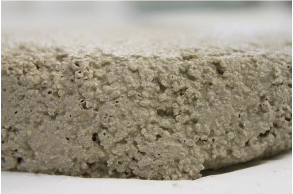
Plaster based on granular Aerogel: samples preparation in laboratory
