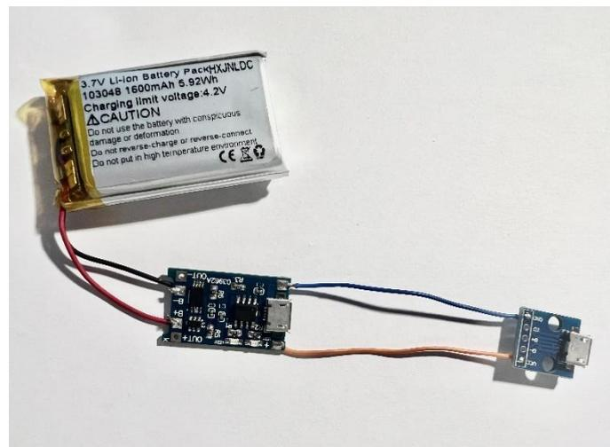
Figure 12: Connection between the USB port and charging board
