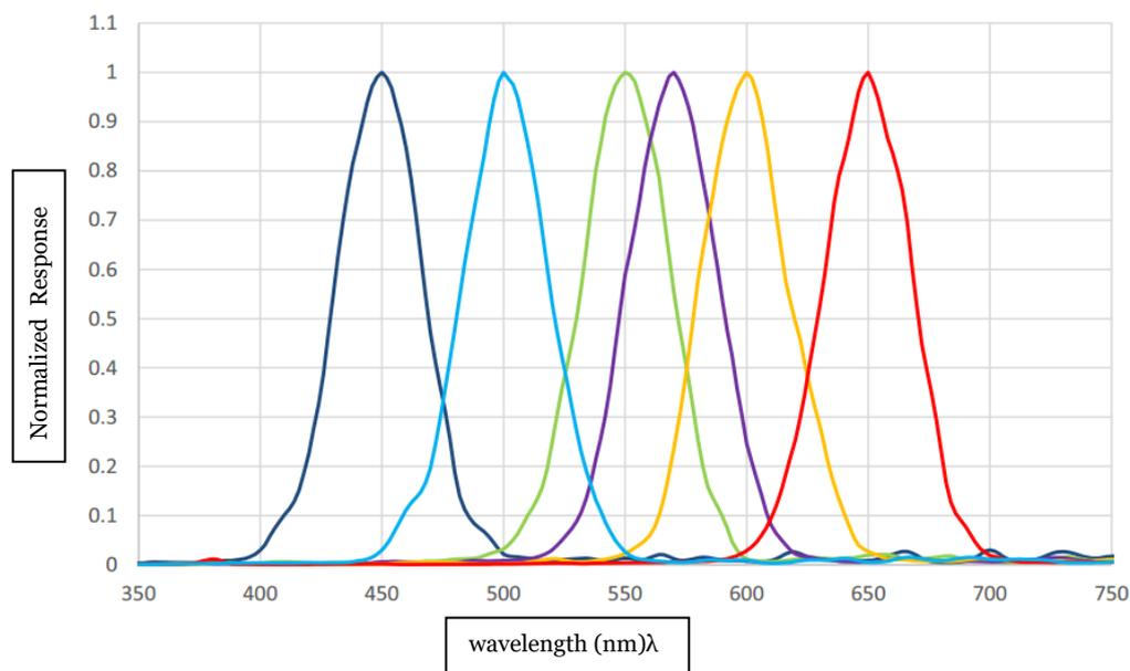
Figure 2: AS7262 output spectral responsivity [15]
