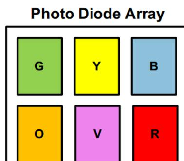
Figure 4: photodiodes array of AS7262 sensor [15]
