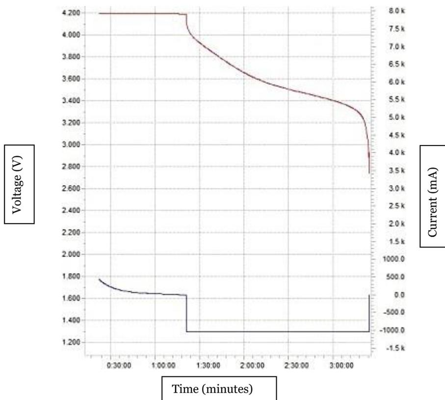
Figure 8: discharging diagram of Li-Ion battery
