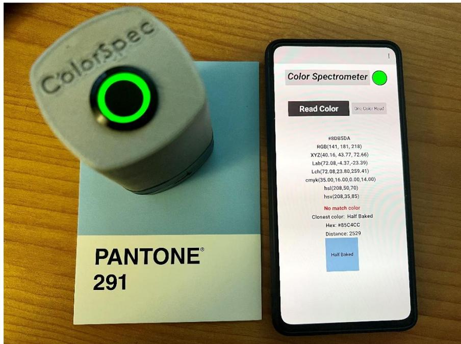
Figure 22: reading a color sample and showing the result
