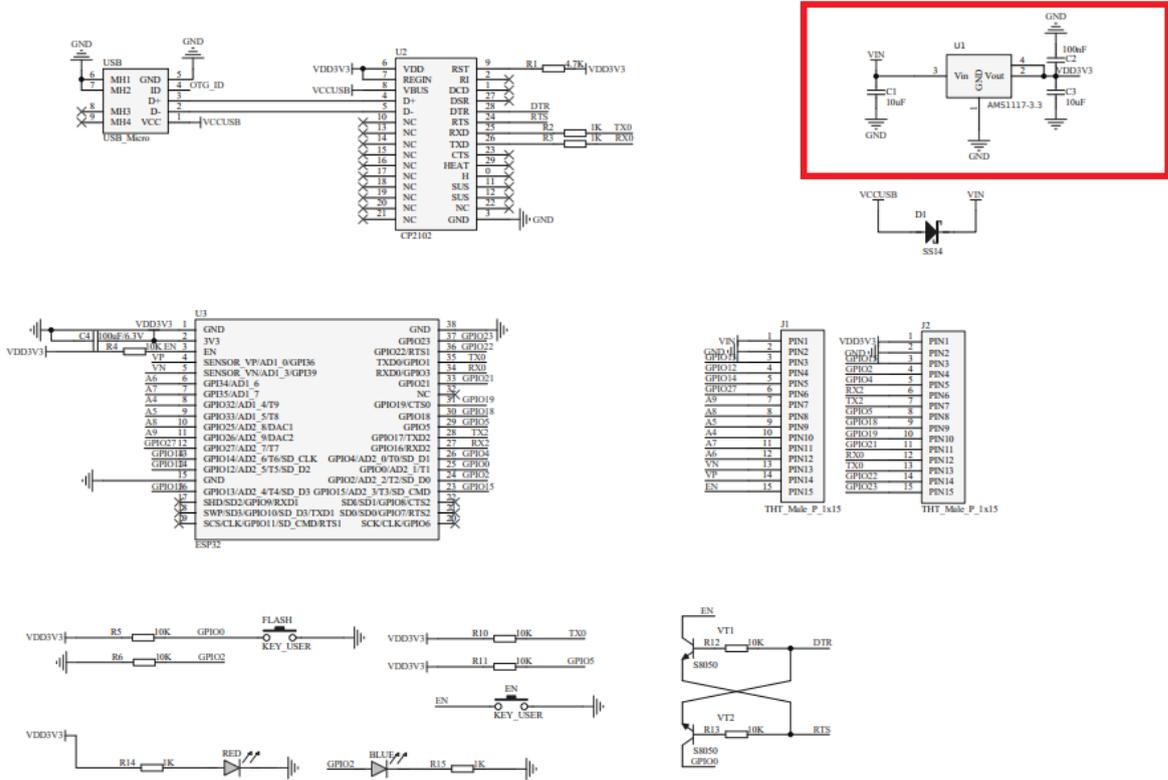
Figure 15: ESP32 devkit v1 schematic [5]
