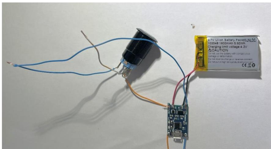
Figure 14: the power connection circuit of the system
