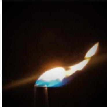
Figure 3.3. Detail of flame affected by turbulent air jet.
