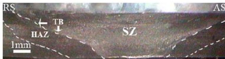
Figure 2.38 Macroscopic view of the joint cross section in condition 4III[32].
