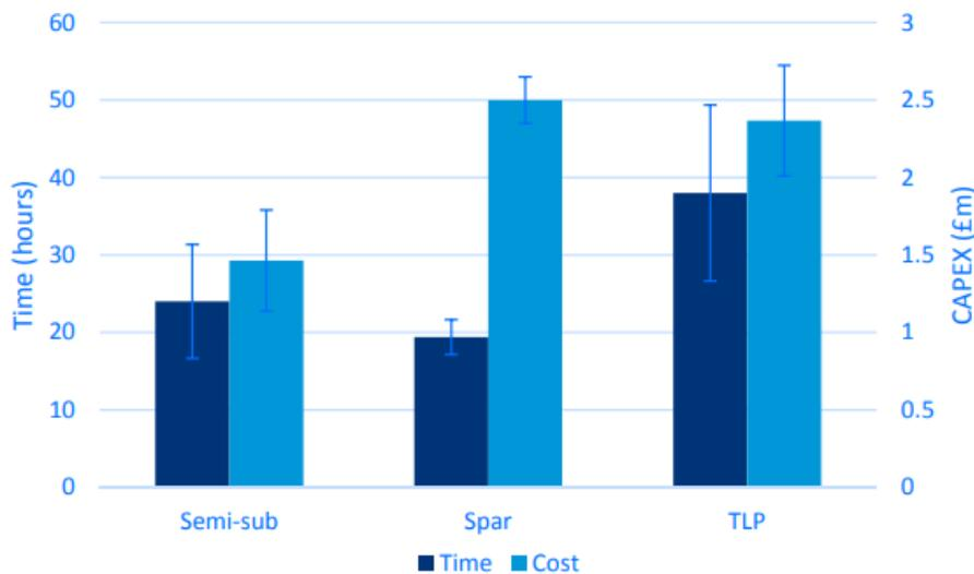
Figure 3.9 Installation time and cost for each type of floating platform [9]
