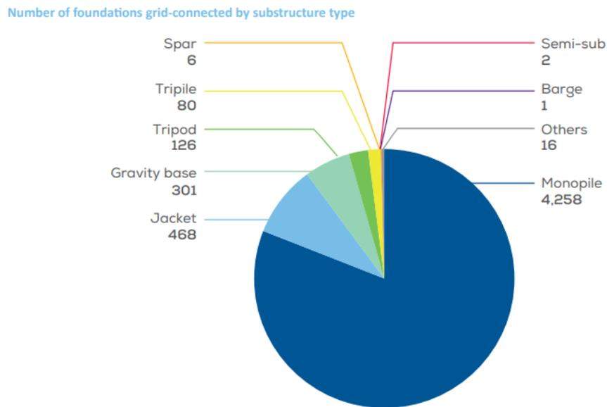
Figure 2.1 Distributions of offshore wind turbine substructures in Europe [4]
