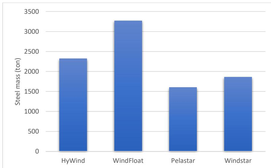
Figure 5.11 Comparison of the structure design based on the steel mass
