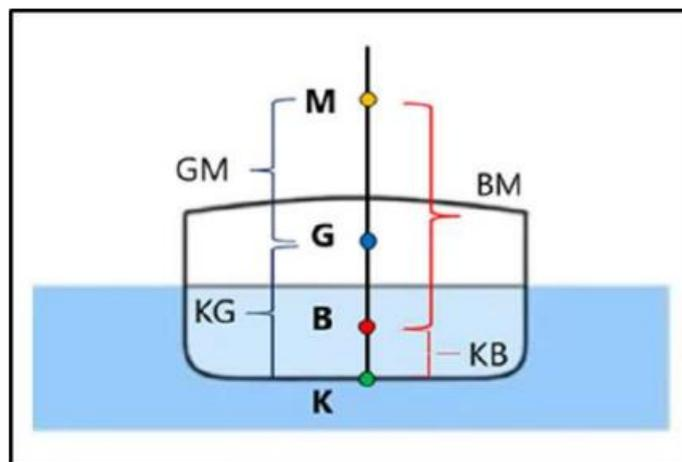
*Figure 4.7 Representation of metacentric height*
