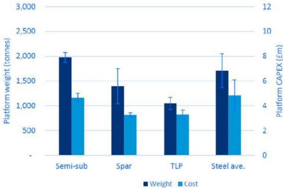
Figure 3.1 Platform weight vs cost (steel). Adapted from [9]
