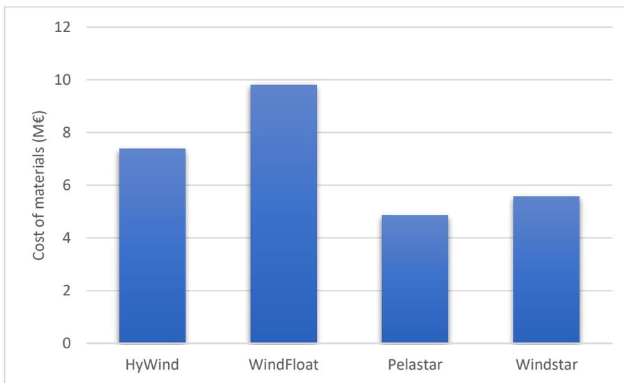
Figure 5.10 Comparison of the structure design based on the cost of materials
