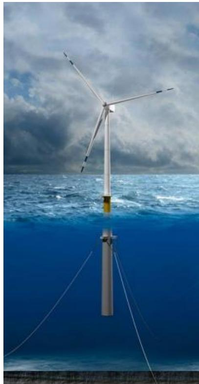
*Figure 2.5 Spar-buoy substructure concept*
