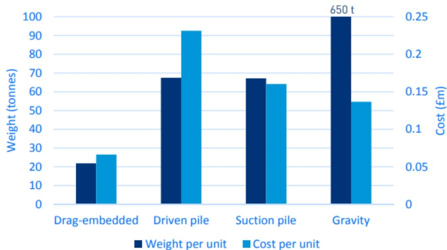
Figure 3.5 Anchor weight and cost per unit, by anchor type [9]
