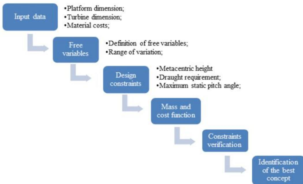
*Figure 5.1 Design optimization process through genetic algorithm*
