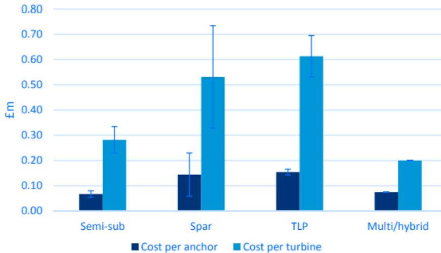
Figure 3.6 Anchor cost per unit and per turbine, by floater typology [9]
