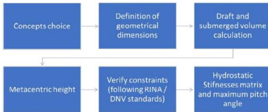
Figure 4.2 Operating scheme of hydrostatic tool
