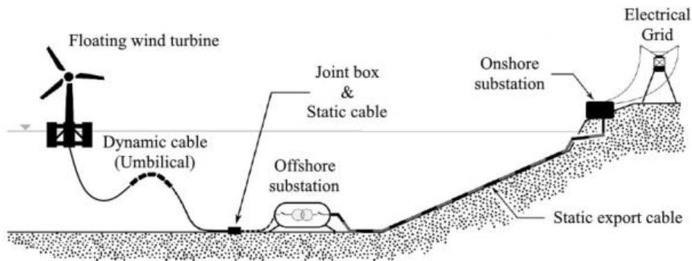
*Figure 3.8 Power transmission system of a floating offshore wind [15]*
