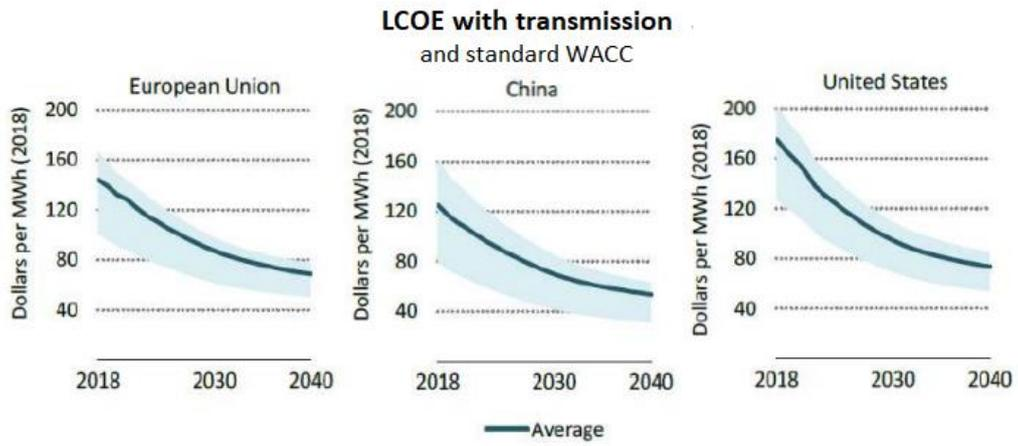
Figure 1.6 LCOE for new offshore wind project in Europe, China and USA in 2018-2040 period
