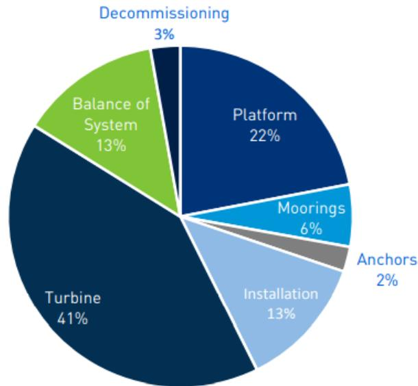
Figure 3.11 CAPEX breakdown for a commercial scale floating wind farm [9]
