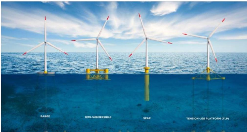
*Figure 2.3 Floating structures classification*
