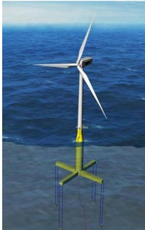
*Figure 2.7 TLP structure design*
