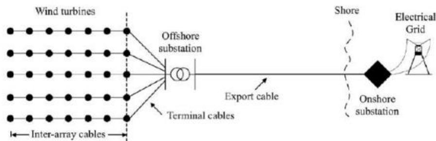
Figure 3.7 Electrical power transmission system of an offshore wind farm in top view [15]
