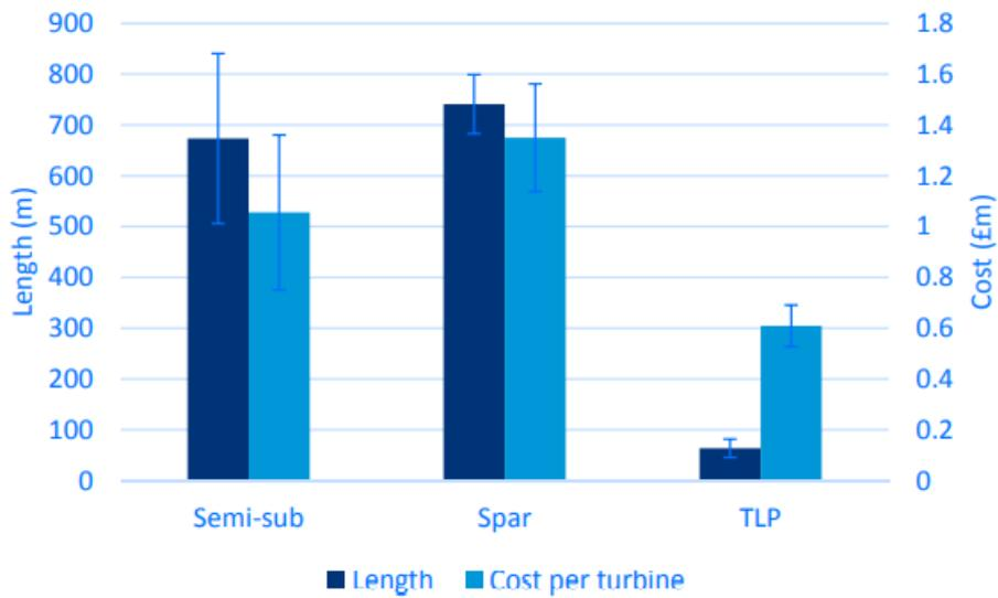
Figure 3.4 Mooring length and cost per turbine, by floater typology [9]
