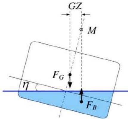
Figure 4.9 Floating structure in heeled condition
