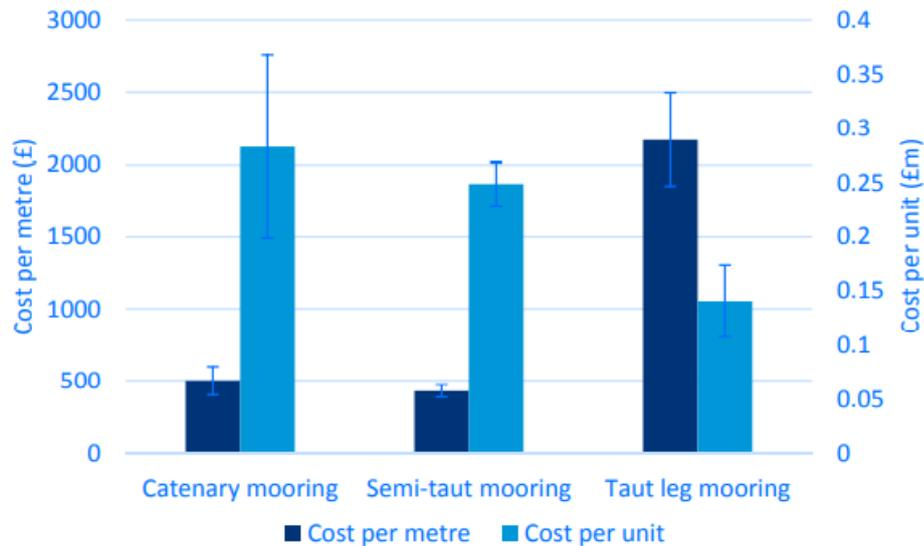
Figure 3.3 Moorings cost per meter and cost per unit [9]
