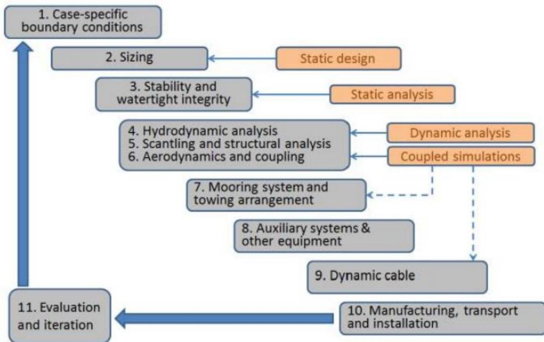
Figure 4.1 Design procedure for a floating offshore wind turbine system [18]
