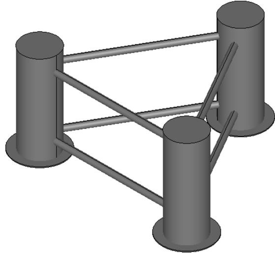
*Figure 4.4 WindFloat concept representation*
