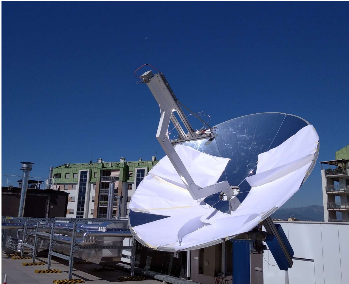
Figure 72: Parabolic collector with covered reflected surface.
