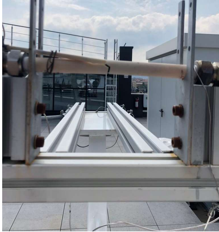
Figure 71: Alumina tube after thermal shock.
