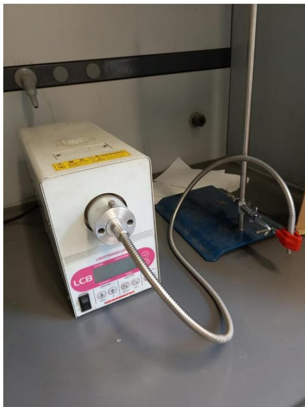
*Fig 39. UV-lamp used to UV-cure chitosan samples*
