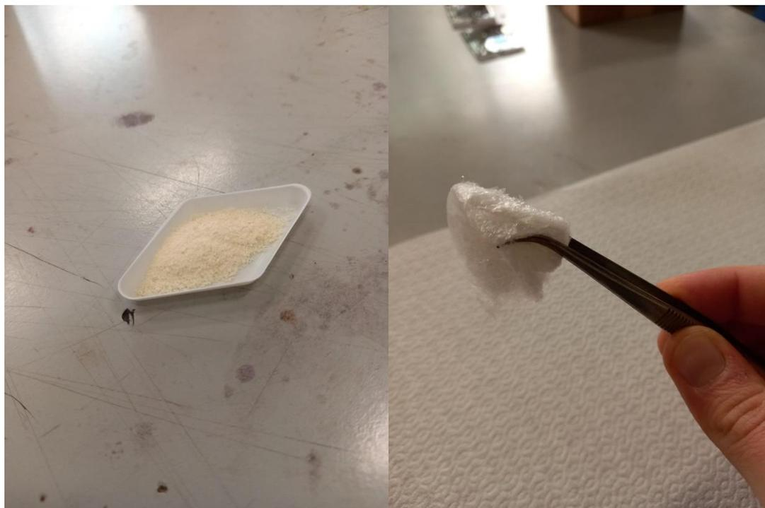
*Fig 36. Raw chitosan (left) and methacrylated chitosan after lyophilization (right)*
