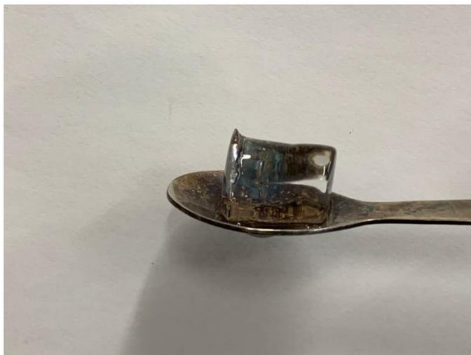
*Fig 38. A chitosan hydrogel as just UV-cured*
