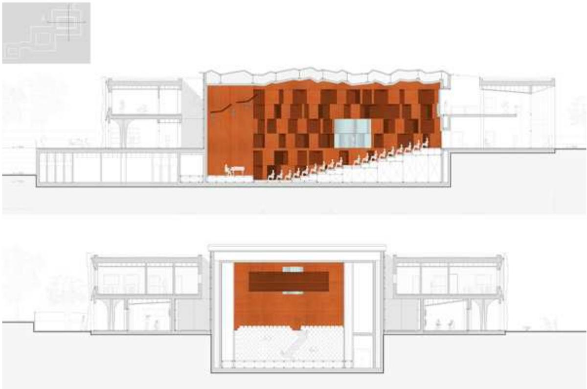
The lining of the hall is made up of modular panels in wood, a solution which allows to split the side walls of the room, creating niches and inclined planes. This choice is justified by the need to converge noise to break the parallelism between the walls, to direct the sound waves reflected in a homogeneous environment and to interrupt large and otherwise monotonous areas.
