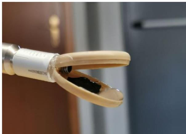
**Figure 5.6** PA molded sample, pressure test.
