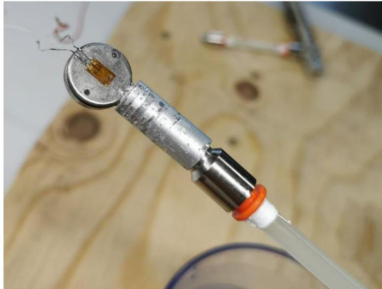
*Figure 4.3* Hand-made fitting connection.
