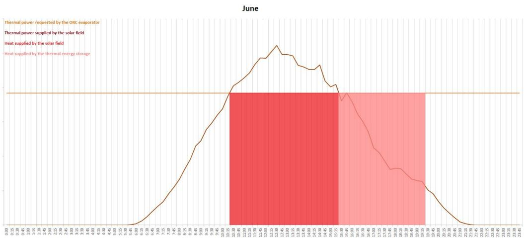
Figure 39 - Power profile during a typical June day
