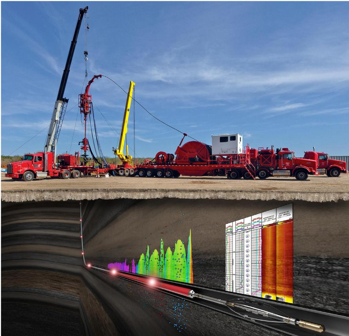
Figure 5.11: SPECTRUM® FUSION Real-Time Hybrid Coiled Tubing Service, [36].
