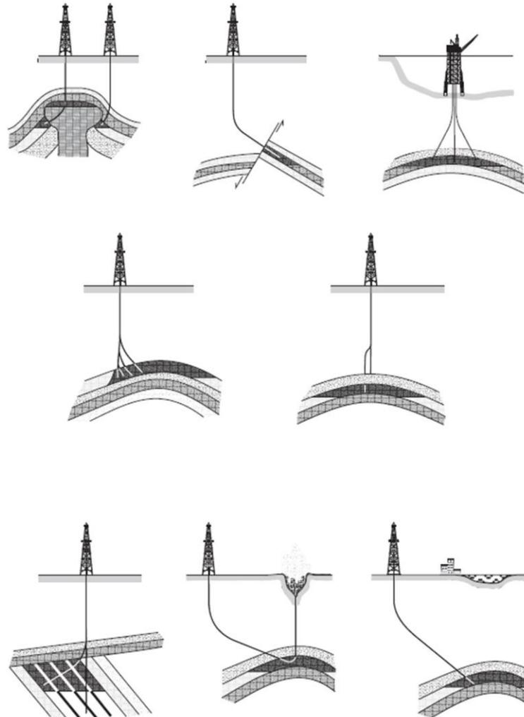
**Figure 2.2:** Directional Drilled wells, [6].
