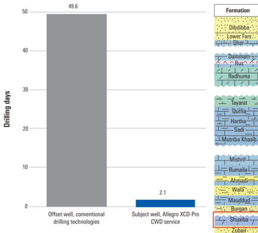
**Figure 4.21:** Comparison between Conventional Drilling Technology vs Allegro XCD-Pro, [43].
