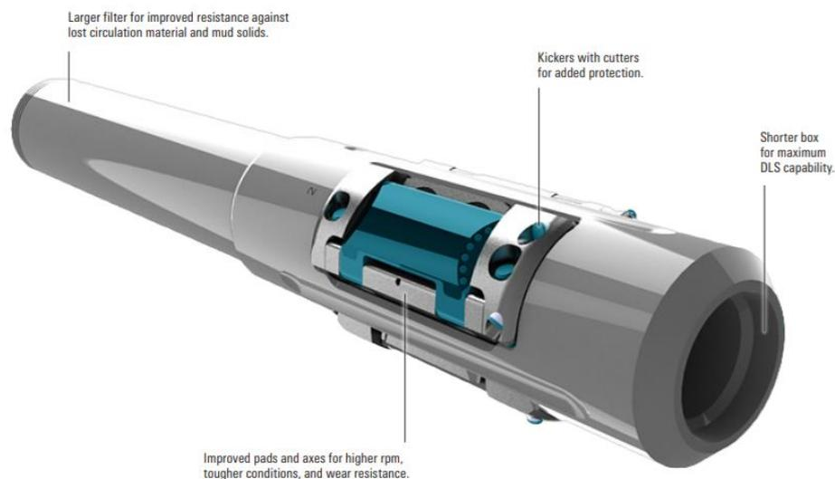
**Figure 4.9:** PowerDrive Orbit G2 Rotary Steerable System, [19].
