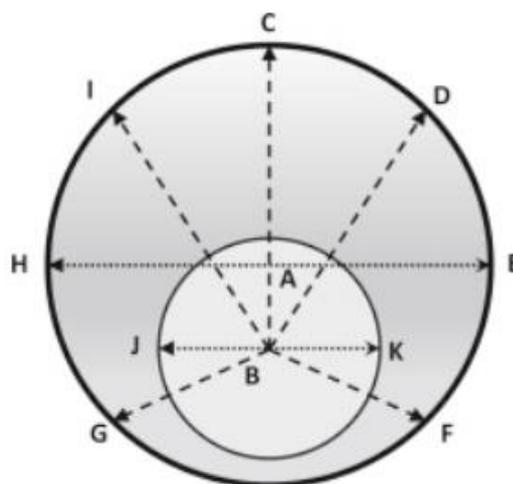
**Figure 2.12:** Tool centering in the wellbore, [6].
