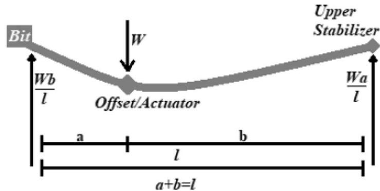
Figure 3.8: Beam bending analysis, [11].
