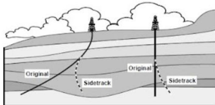
**Figure 2.6:** Sidetracking
