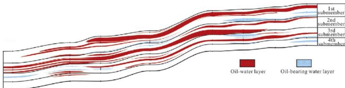
**Figure 4.2:** The quasi-continuous oil tight sandstone reservoirs, [15].
