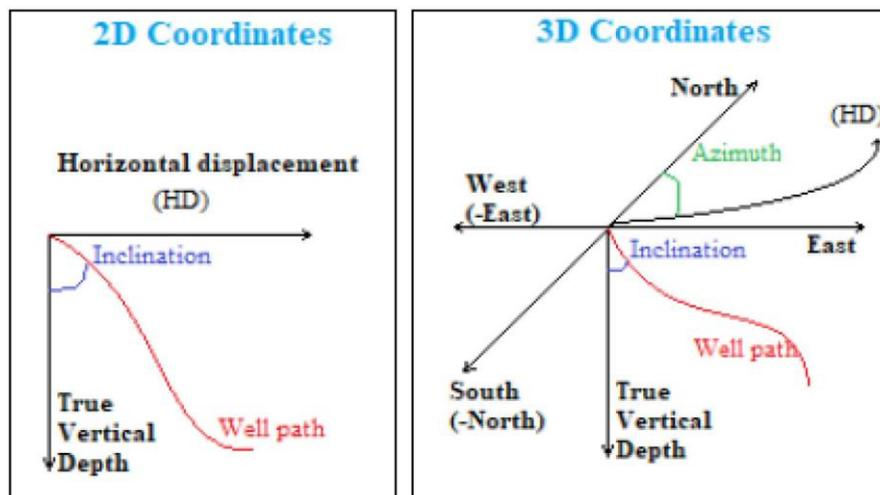
Figure 3.9: 2D and 3D cases for well path visualization, [11].
