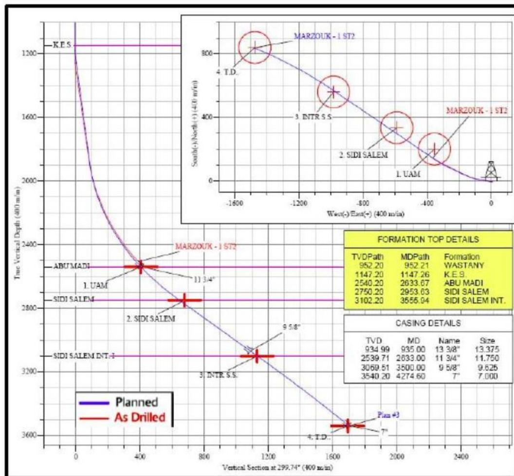
Figure 2.5: J Profile Directional well plan (Jones et al., 2008), [7].
