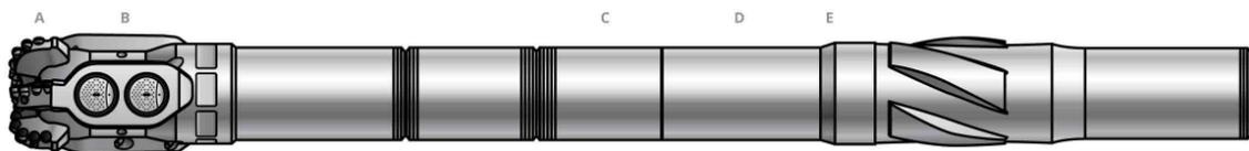
**Figure 4.7:** NeoSteer CLx RSS Tool Assembly, [17].
