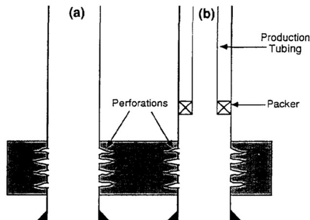
**Figure 5.3:** (a) perforated completion. (b) completion string inside perforated casing, [29].
