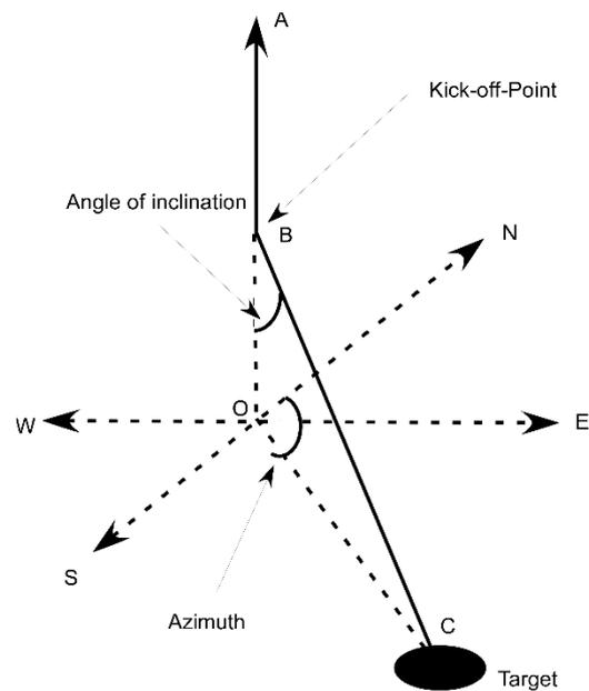
**Figure 2.1: Measurement Parameters of a directional well, [5].**
