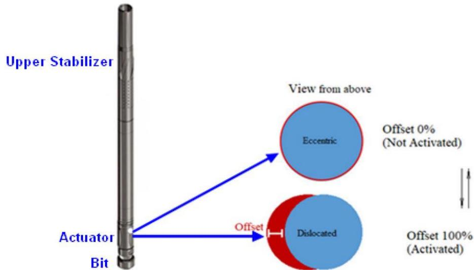
Figure 3.3: RSS work principle, [11].
