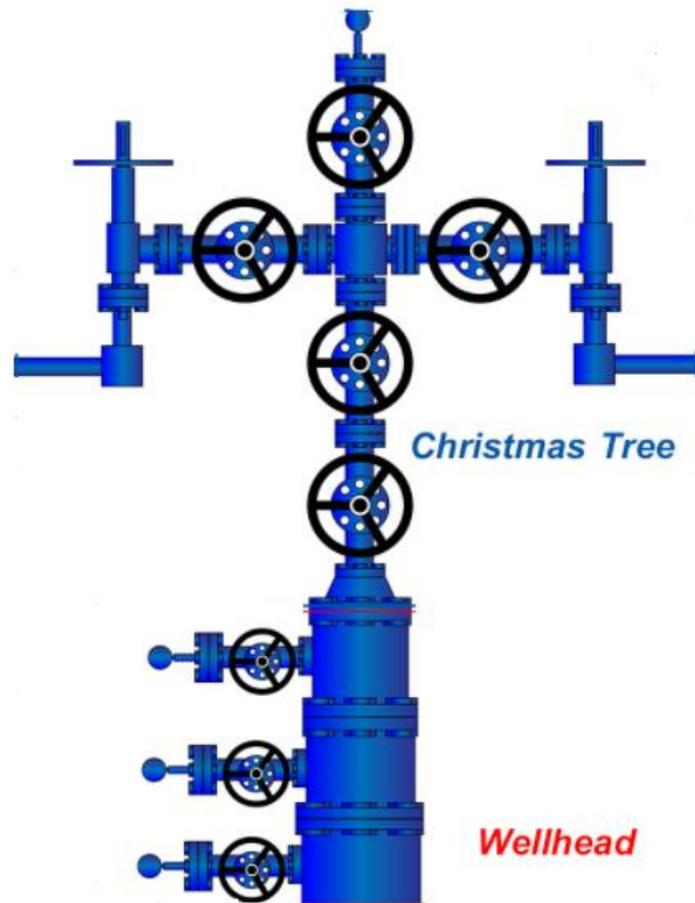
**Figure 5.7:** Wellhead and Production Christmas Tree diagram, [37].
