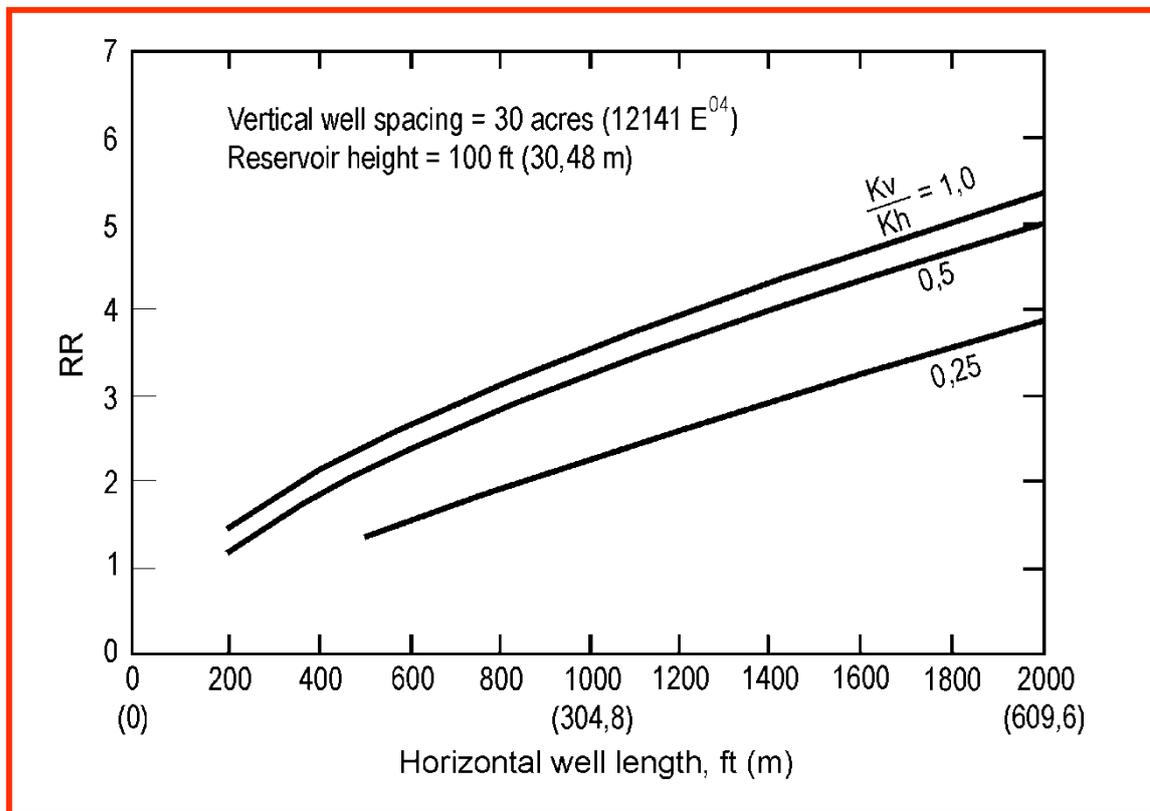
**Figure 4.5:** Horizontal Well Productivity as a Function of  $k_v/k_h$  Ratio, [15].
