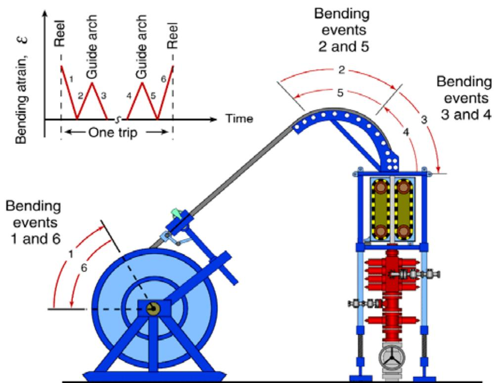
Figure 5.10: Coiled tubing method, [35].
