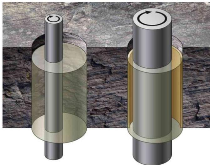
**Figure 4.20:** Casing while Drilling.
