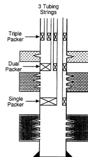
**Figure 5.5:** Wellbore diagram of a conventional triple completion, [29].
