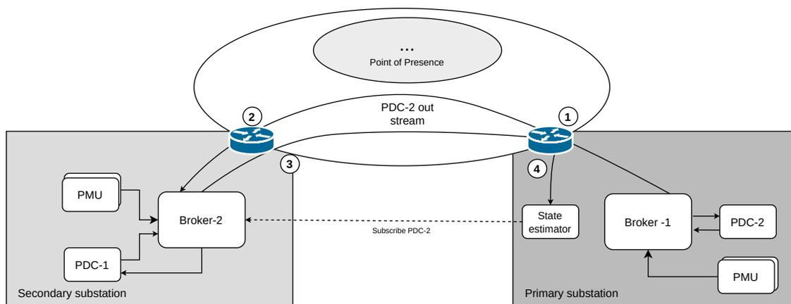
Figure 6.6: Unoptimized traffic caused by subscription to a wrong broker instance
