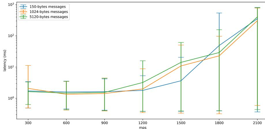
Figure 5.8: Message latencies varying the dimension of the payload with QoS-1
