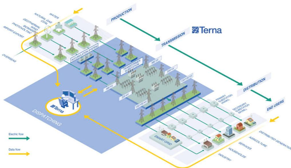
Figure 2.6: Terna's transmission system [61]
