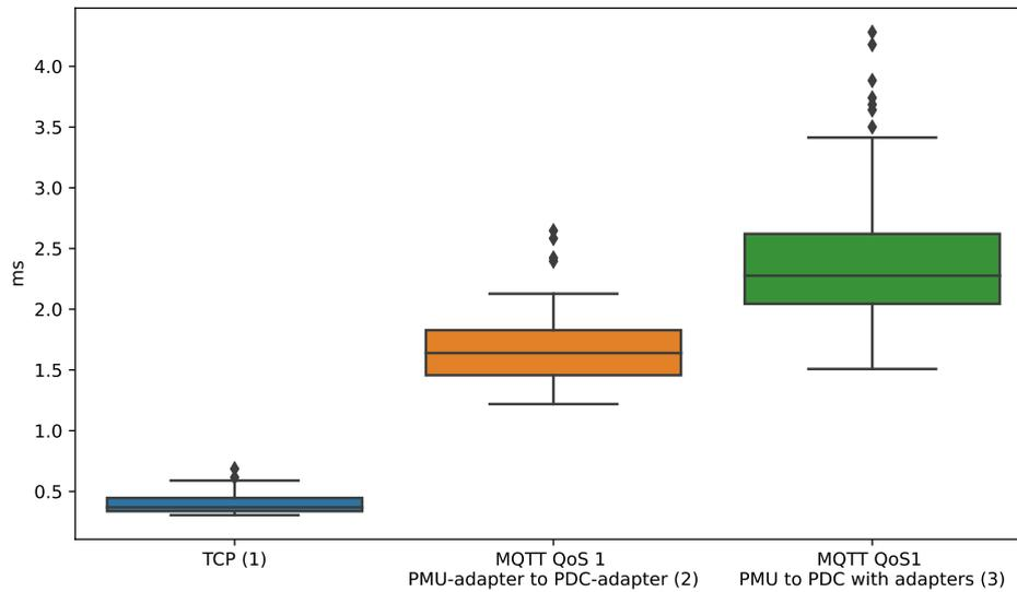
Figure 7.6: Message latency of IEEE C37.118 data transported over TCP and MQTT QoS 1
