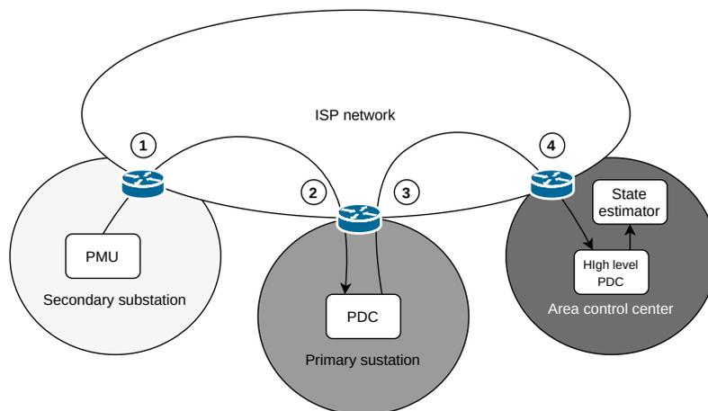
Figure 6.2: Data enters and exits from the power provider network four times
