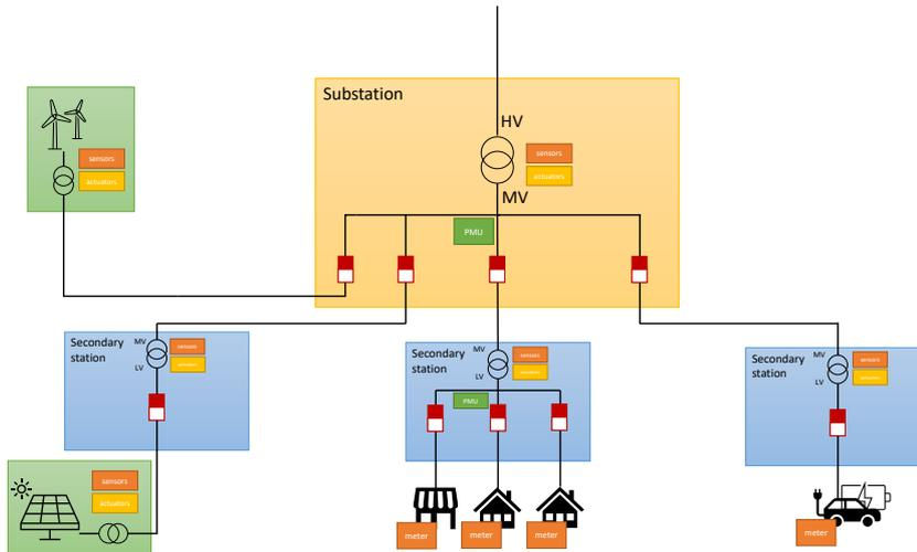
Figure 2.10: Electrical architecture of the distribution system.
