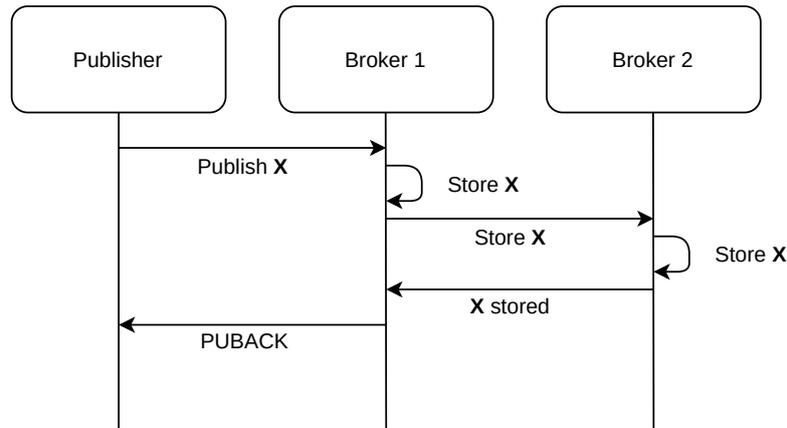
Figure 5.3: Interaction between publishers and broker instances with queue mirroring enabled. Time from up to down.
