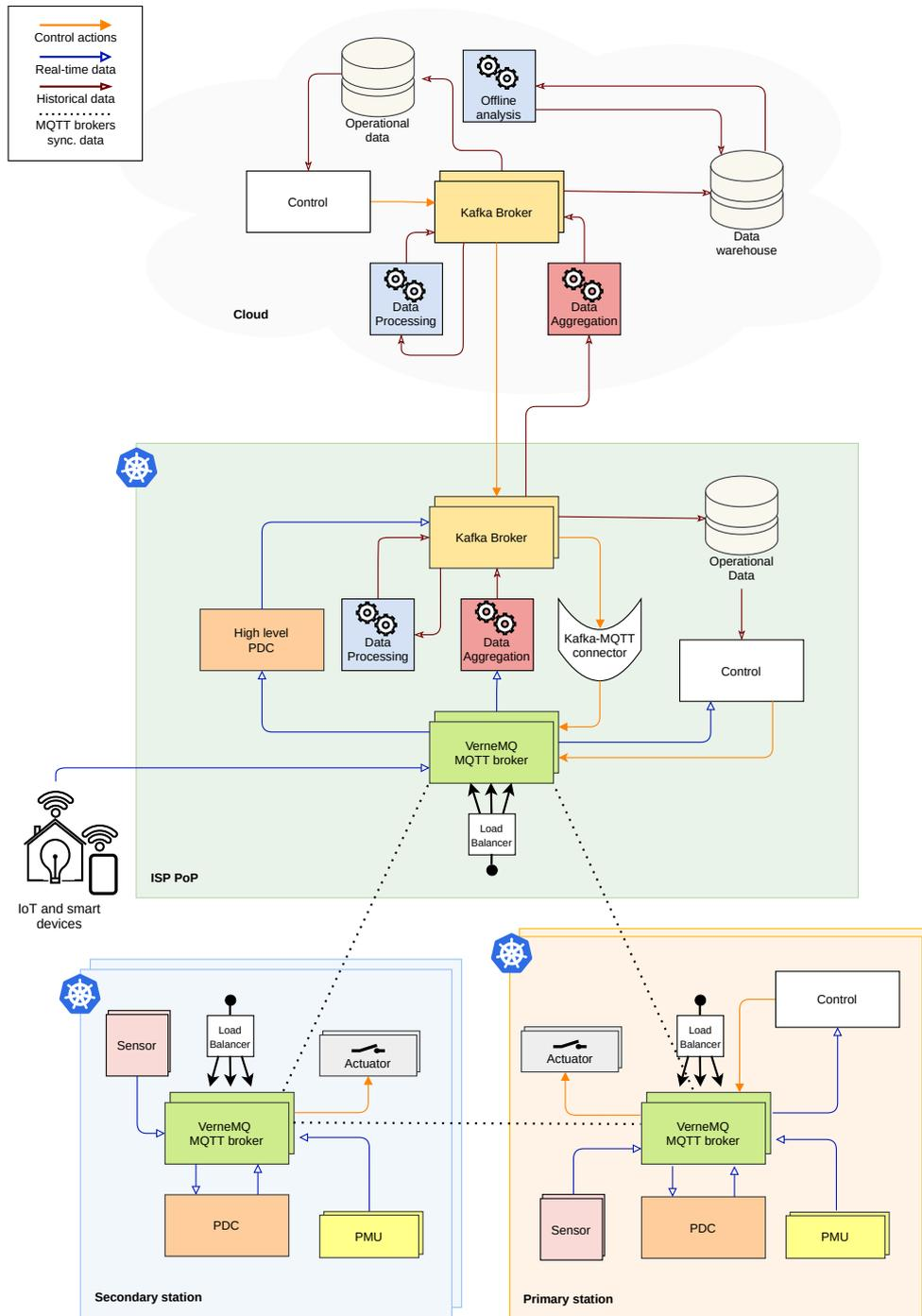
Figure 7.1: Implemented architecture: the distributed broker collect data from the edge, which is then processed in Kafka
