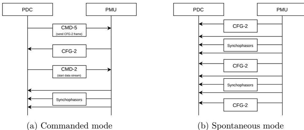
Figure 4.4: Exchanged messages in commanded and spontaneous modes. Time from up to down.
