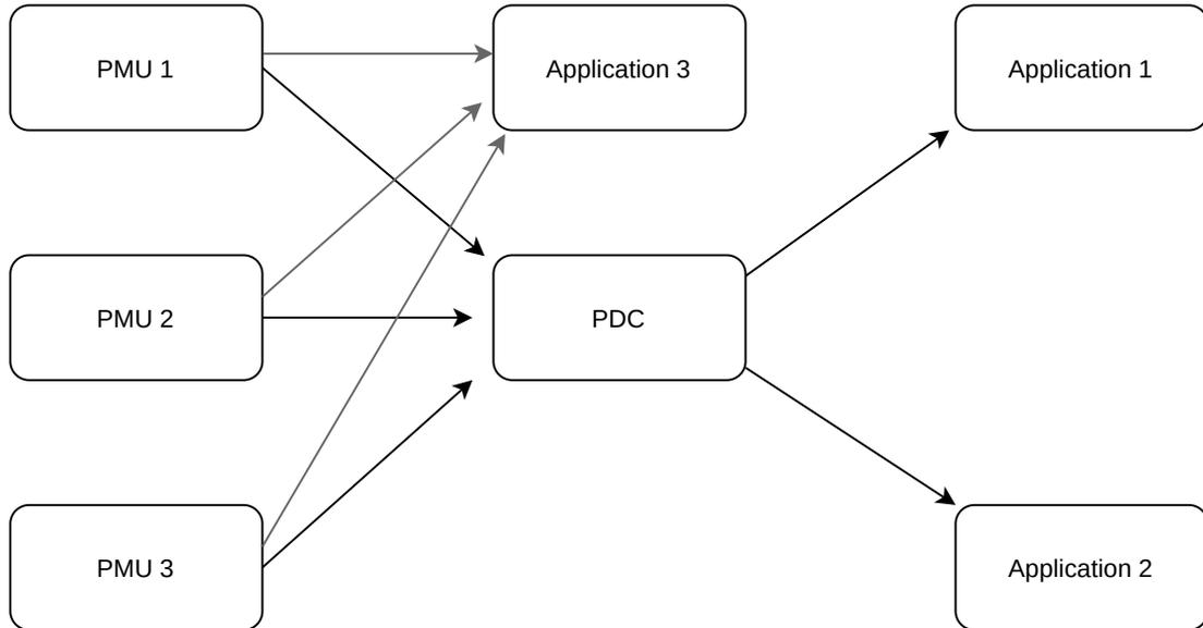
Figure 4.1: Point-to-point interaction between PMUs, PDC and applications
