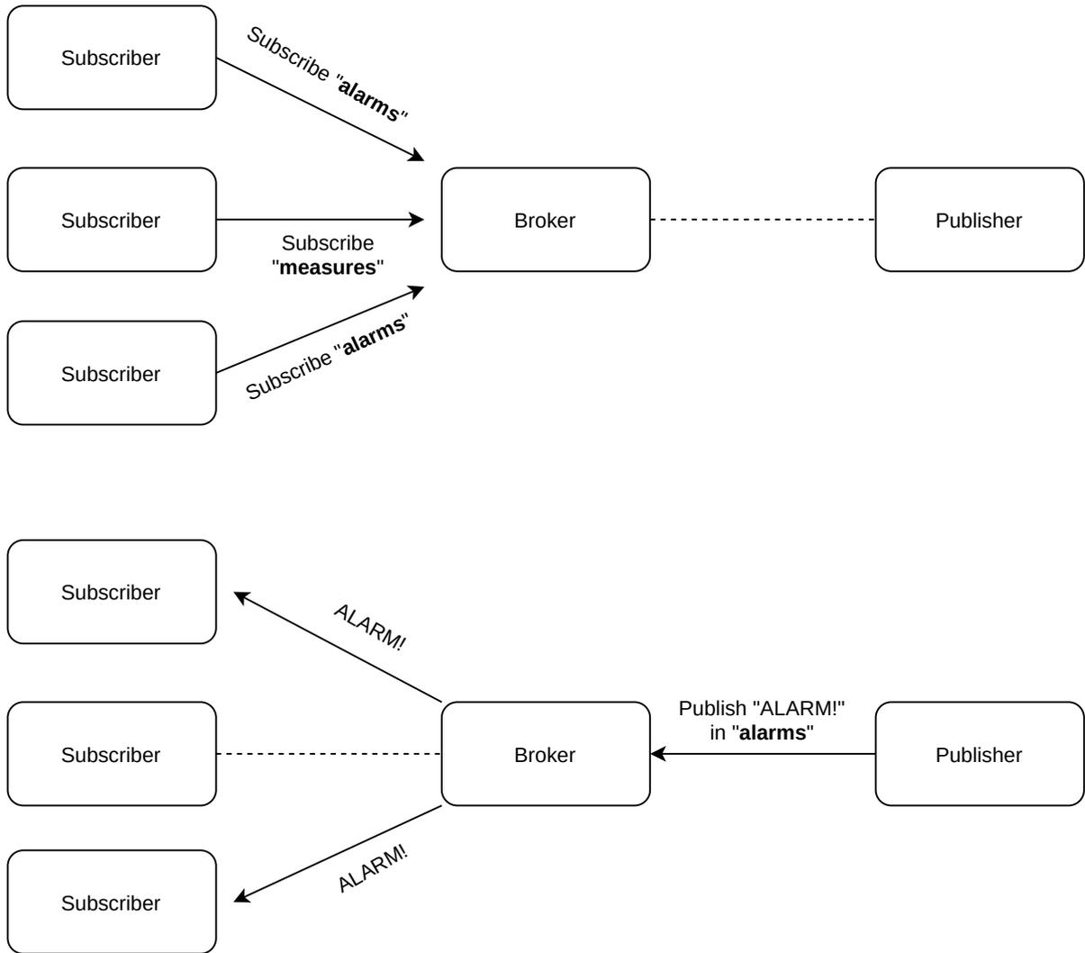
Figure 3.1: Example of interaction between publishers and subscribers with message broker
