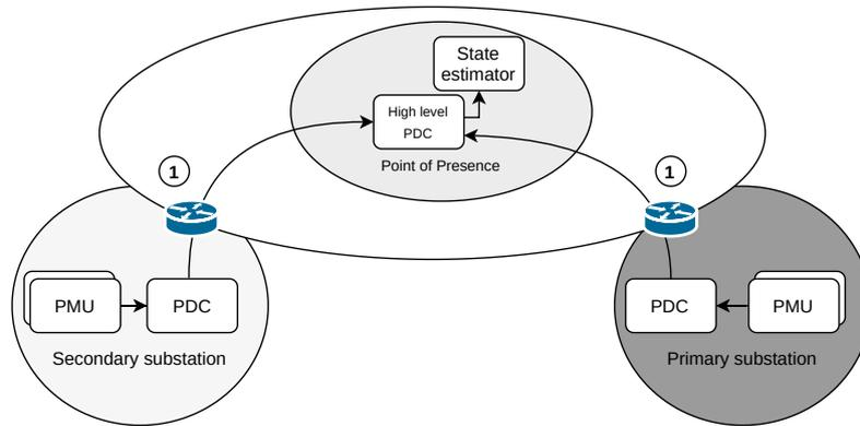
Figure 6.4: Data exits a single time from the electricity provider network reaching the PoP
