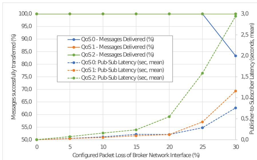
Figure 5.1: © 2021 IEEE - Message loss and latency for each QoS level, increasing the network loss rate [41]
