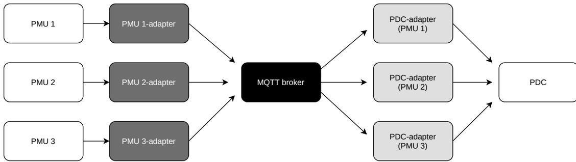
Figure 7.3: Example of a deployment of the adapters
