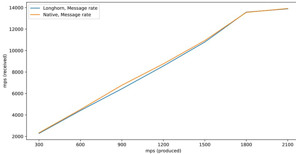
Figure 5.7: 150 bytes messages - received message rate comparison increasing producers message rate, with native storage and Longhorn replicated storage
