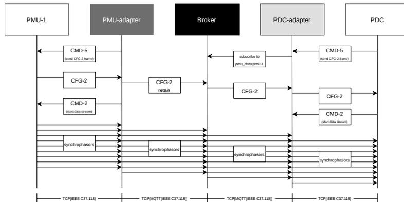
Figure 7.2: Schema of the interaction between adapters and broker
