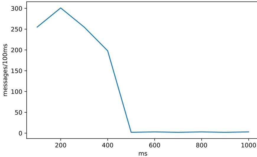
Figure 7.5: Message rate from connection restore after 1 minute of disconnection from the broker
