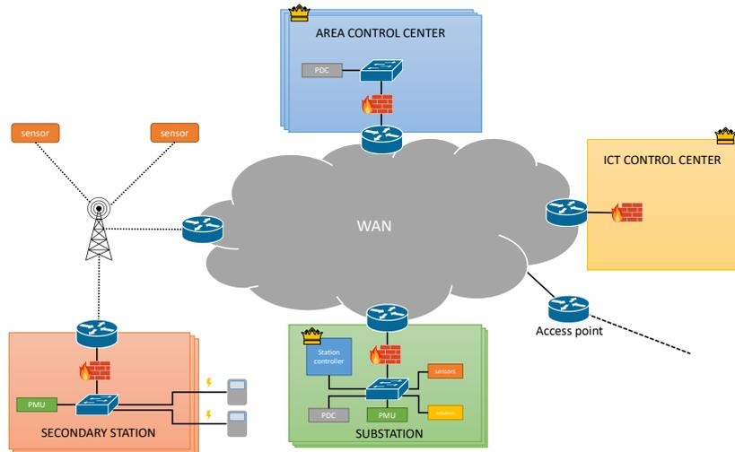
Figure 2.7: ICT network architecture in the distribution system.
