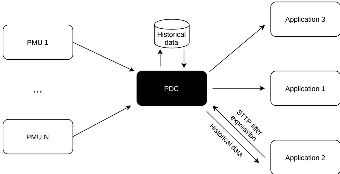
Figure 4.3: Example of architecture using the STTP protocol and the PDC as a broker
