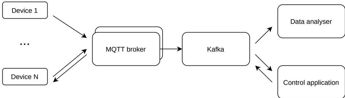
Figure 3.2: Example of integration of MQTT and Kafka
