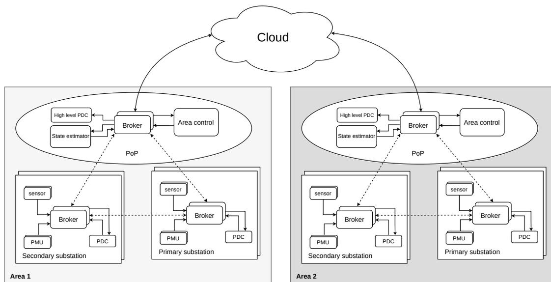
Figure 6.5: Distribution system as a data-centric architecture
