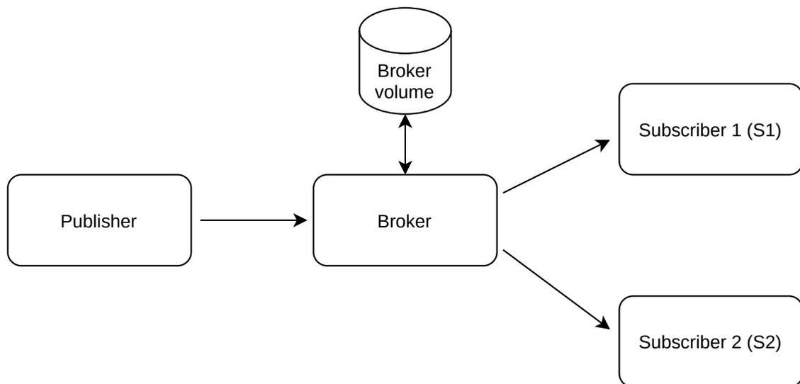
Figure 5.2: Schema of the scenario of the Grüner et al. data persistency experiment
