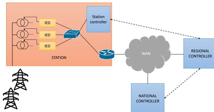
Figure 2.5: ICT network architecture of the transmission system.
