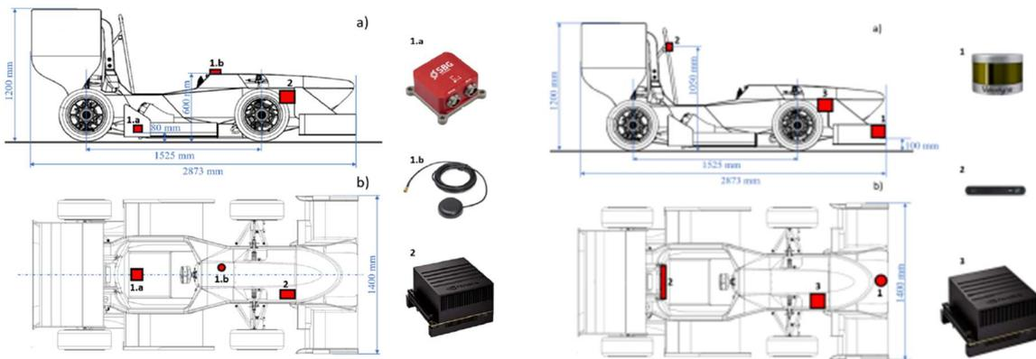
Figure 2.14: Hardware Configuration of the SC19
