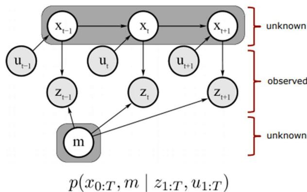
Figure 2.12: Graphical Model of the SLAM Process
