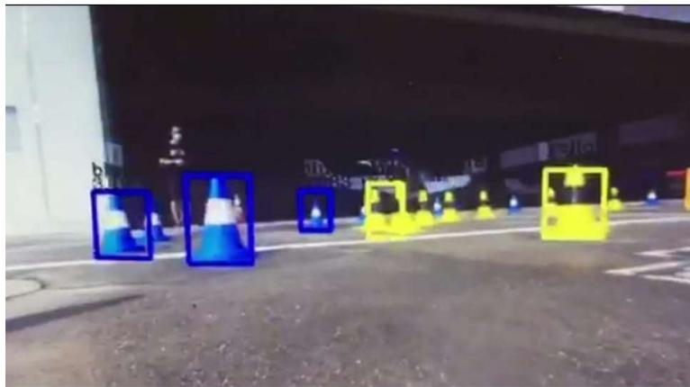
*Figure 4.8: /processedImage Output Topic of a Real Experiment*
