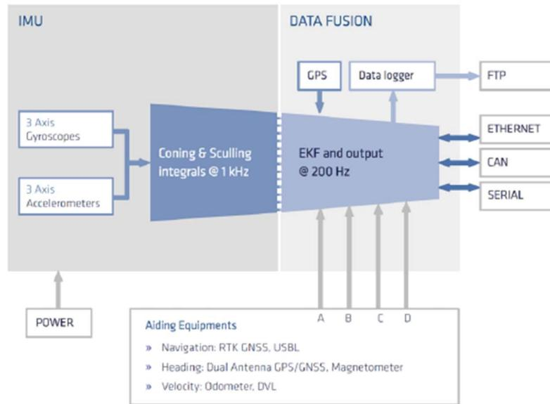
Figure 2.8: INS Internal Architecture
