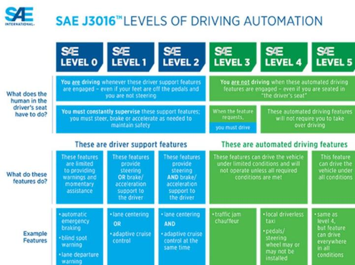
Figure 1.2: SAE Levels of Driving Automation
