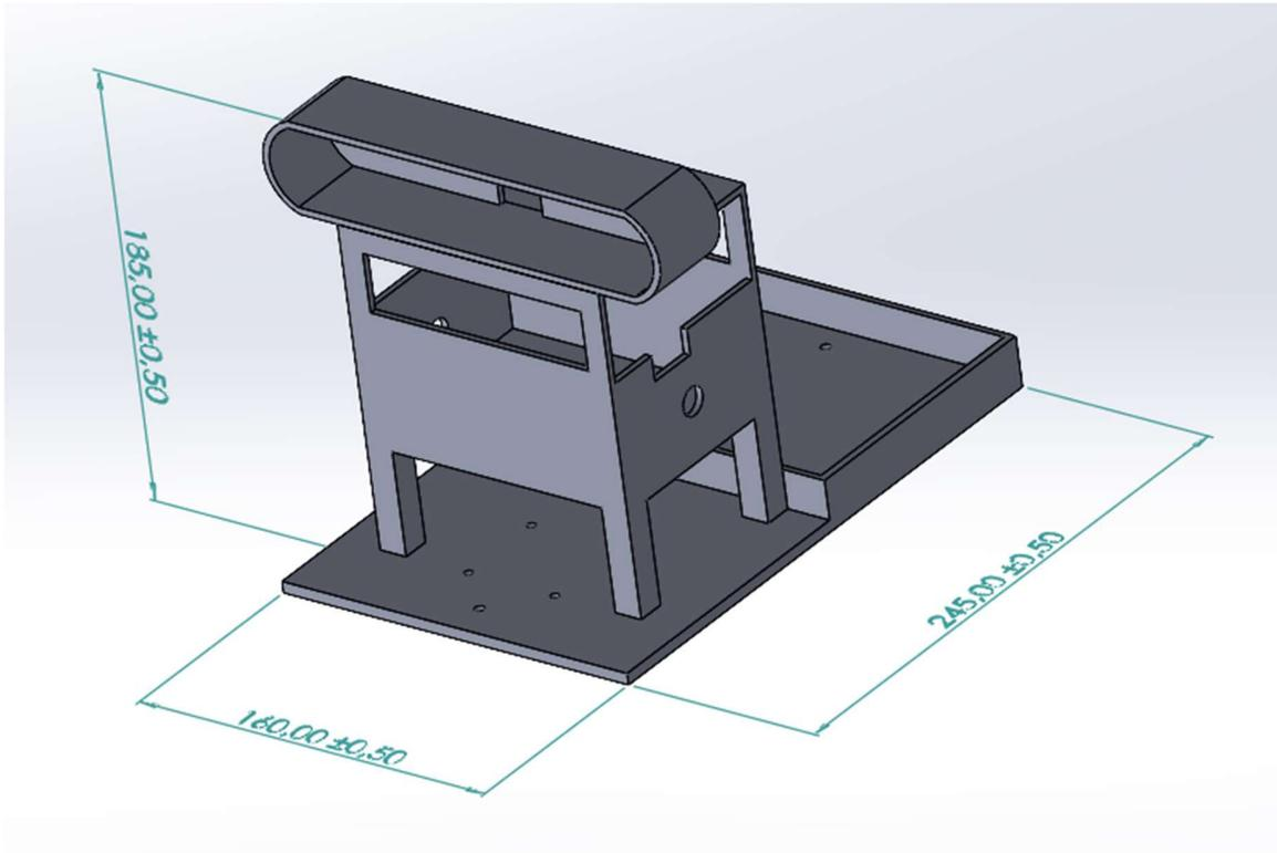
Figure 4.6: 3D Structure for the RC Model
