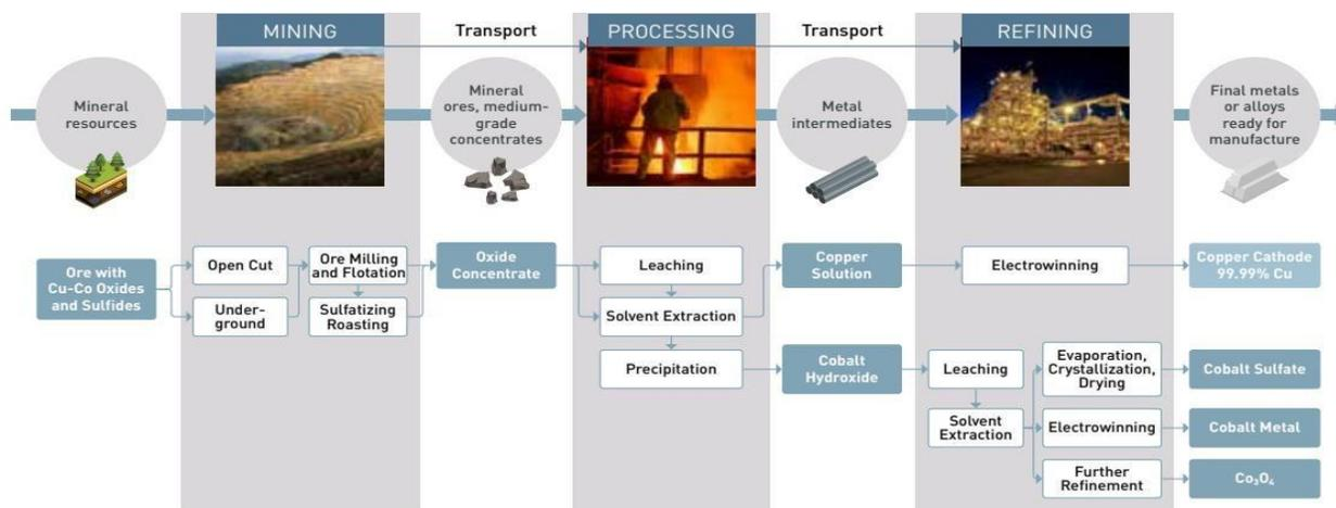
Figure 4: Cobalt production as byproduct of copper oxides (hydro) (Dai et al., 2018).
