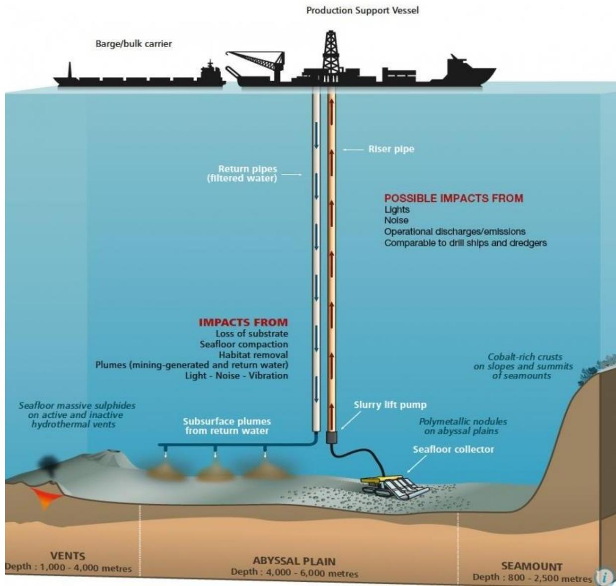
Figure 12: A schematic view of continuous mining.
