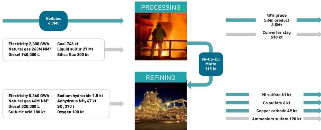
Figure 17: Sample material flows for 4.9 mt/year nodule processing and refining plant.
