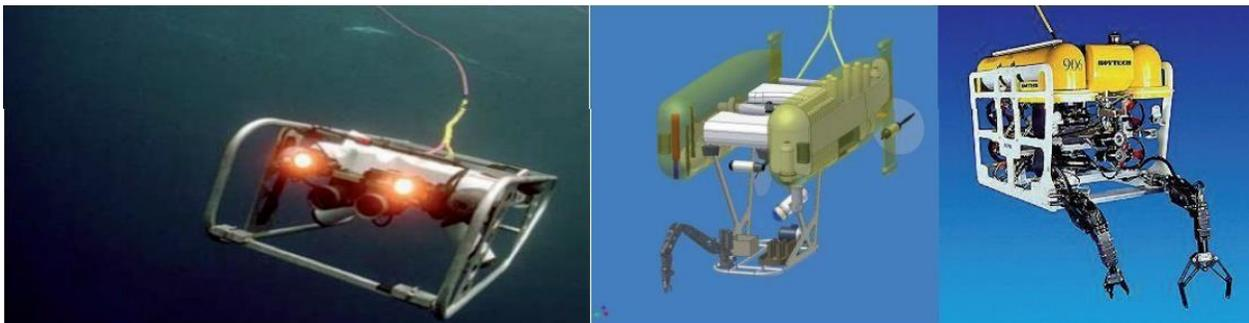
Figure 10: Types of remotely operated vehicles (Egorov, 2014)
