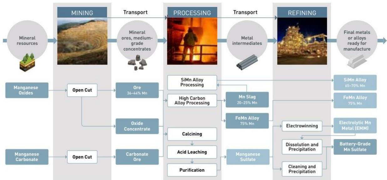
Figure 5: Manganese sulfate and alloy production (Dai et al., 2018)
