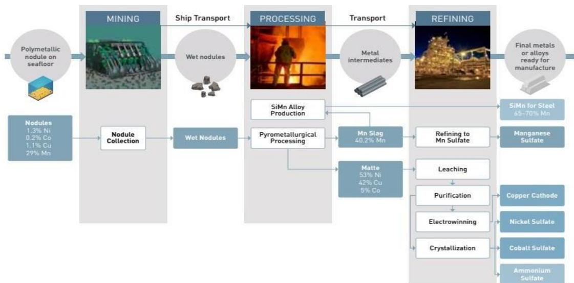
**Figure 16: Processing polymetallic deep-sea nodules.**
