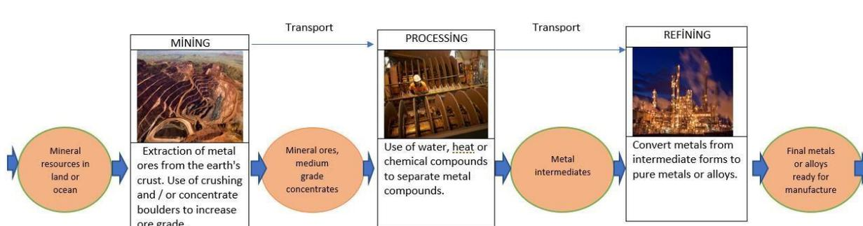
Figure 2: Generalized production of metals, cradle-to-gate (Nuss and Eckelman, 2014)
