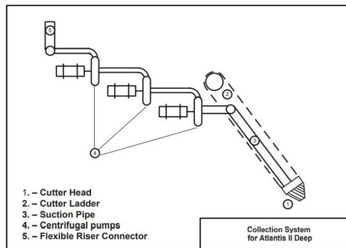
**Figure 14: Schematic Of The New Collection System**
