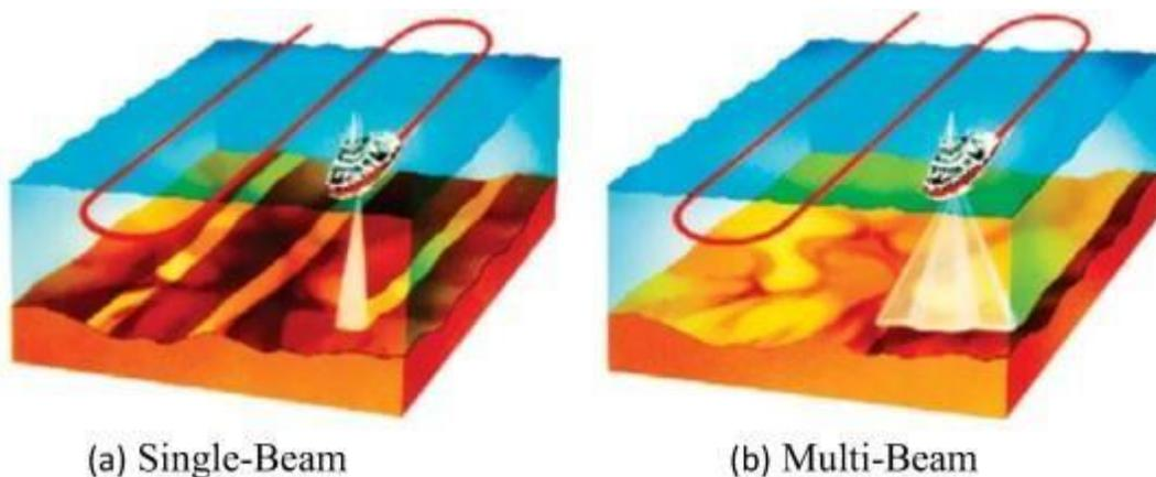
Figure 9: COVERAGE OF SINGLE-BEAM AND MULTI-BEAM ECHO SOUNDERS (KEARNS AND BREMAN, 2010).
