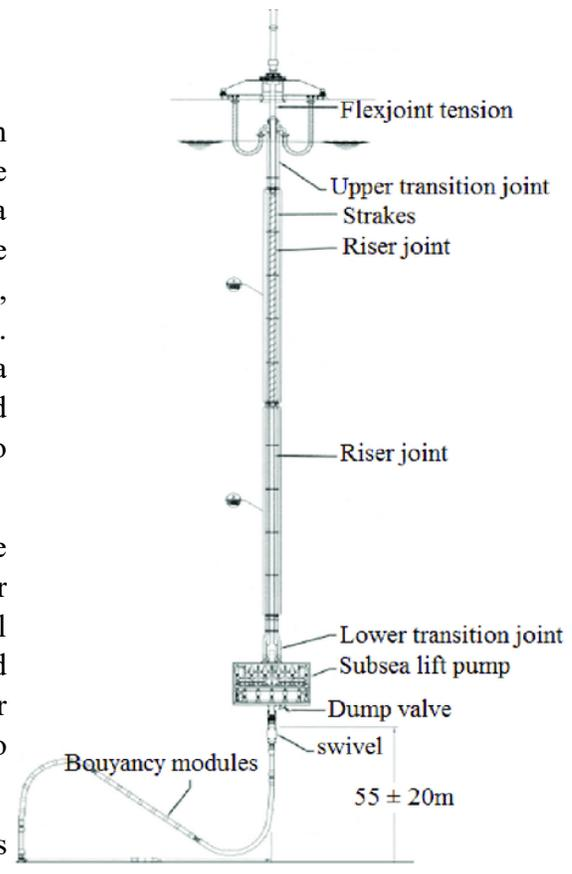
Figure 15: Nautilus: riser and lift system
