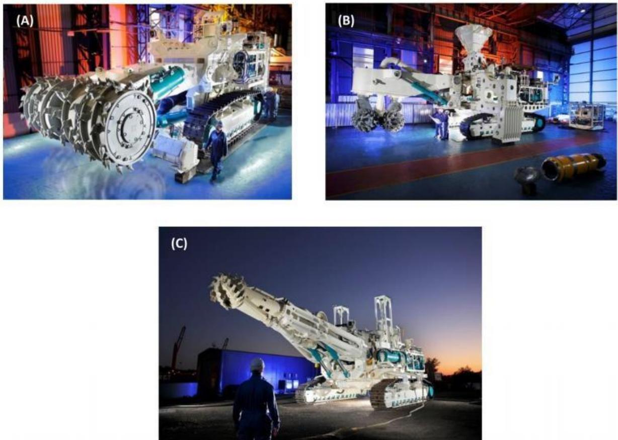
Figure 13: Machinery for the exploitation of resources of the seabed, owned by Nautilus Minerals company (a: bulk cutter (bc), b: auxiliary cutter (ac), c: collection machine (cm)) (modified from Nautilusminerals, 2019).
