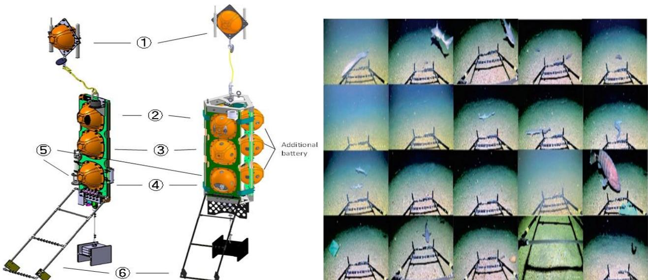
Figure 11: A) External view of edokko mark 1. The left side is a lightweight model. The right side is a long-term observation model.
