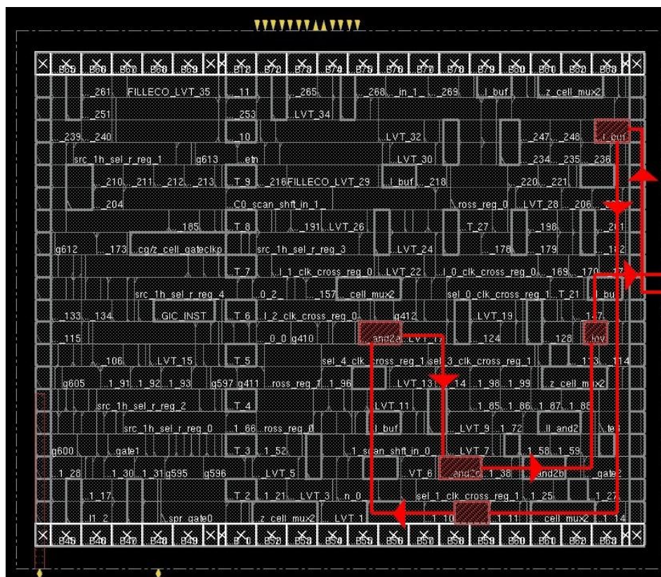
Figure 7: Physical view of the dsc_clkctrl_gcm5 module showing the path of the clock pll_0.
