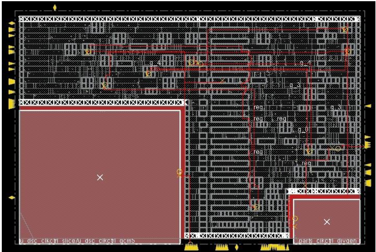
Figure 8: Physical view of the ssslice module showing the path of the clock pll_0. (A circle is the start point of a signal and a cross is its endpoint).
