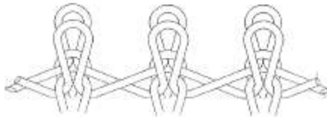
**Figura 3-14:** Schema costruzione interlock (Handbook of technical Textile, Fig. 5.14 Weft-knitted structures E)
