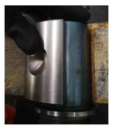
*Figure 70.* Step 1 – Putting the bushing on the engineering blue on the spindle.
