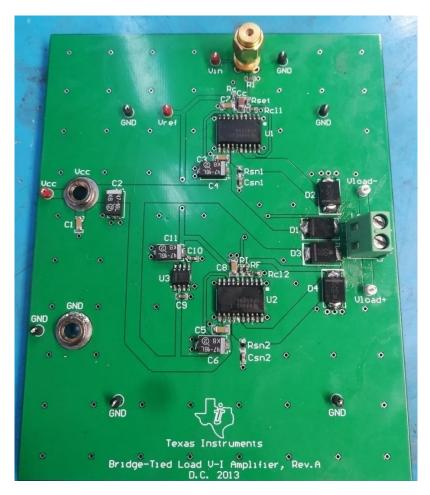
Figure 34. Homemade Texas Instrument V-I amplifier PCB.
