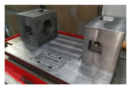
Figure 40. Cases and metal plate before burnishing operation.
