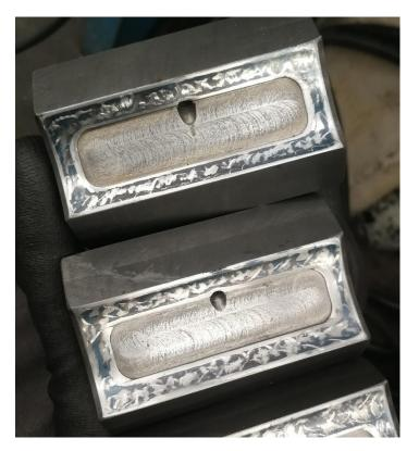
Figure 73. Final result of scraped pads.
