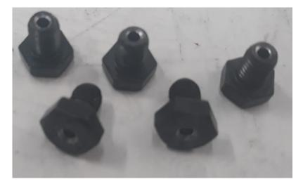
Figure 41. Drilled screws to allow O-ring crushing.
