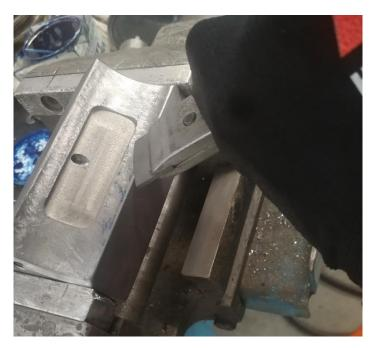
Figure 72. Step 3 - Scraping process.
