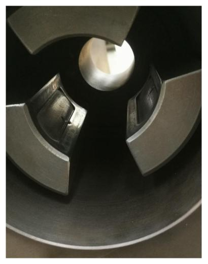
Figure 45. Bushings assembled inside the case.
