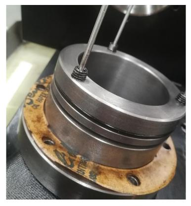
Figure 42. Pipes and stopper preassembly.
