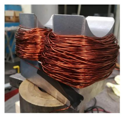
Figure 29. Magnet loader (electromagnet) with 450 coils.
