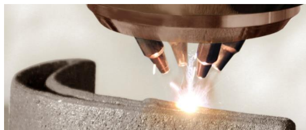
Fig. 1.11 Deposition head with 4 powder nozzles configuration adopted by Prima Additive [25]
