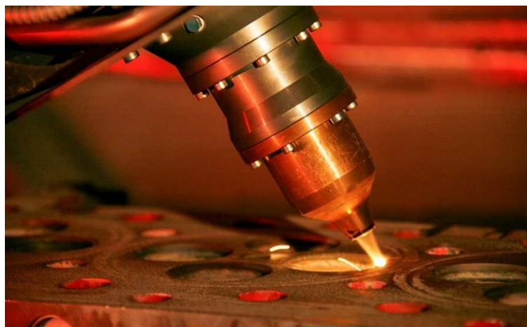
Fig. 1.9 An example of oblique deposition [26]
