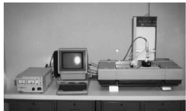
Fig. 1.4 The SLA-1 system: the first AM technology launched in 1987 by 3D systems [1]
