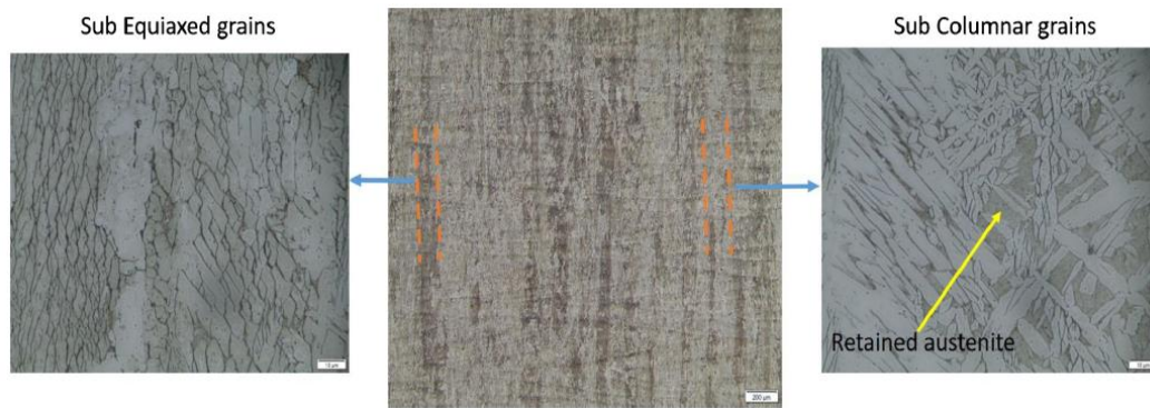
Fig. 2.6 Equiaxed and columnar grains in a 17-4 PH sample [38]
