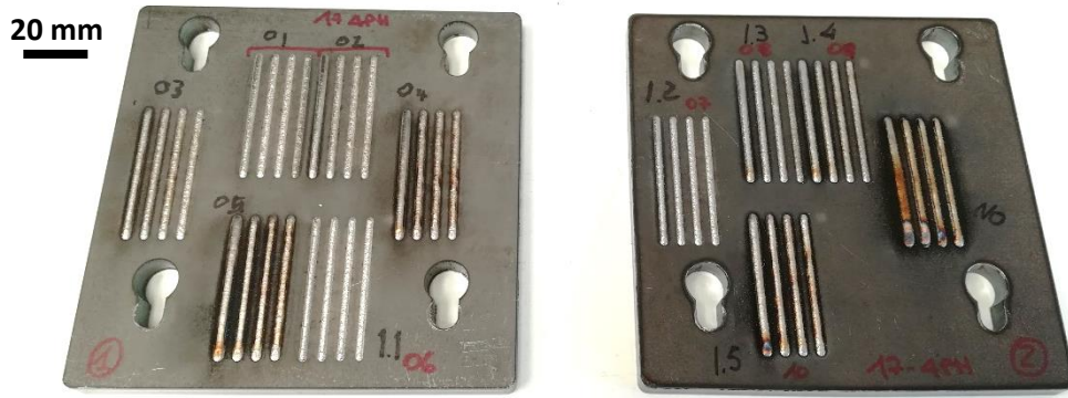
Fig. 3.8 Single Scan Tracks deposited on two baseplates
