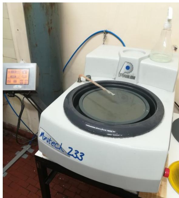
Fig. 3.10 Polishing machine Presi Minitech 233
