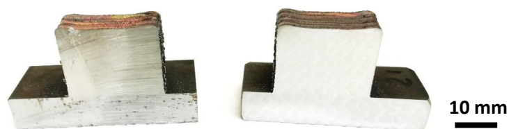
Fig. 3.16 Massive cube sections before and after grinding and polishing operations
