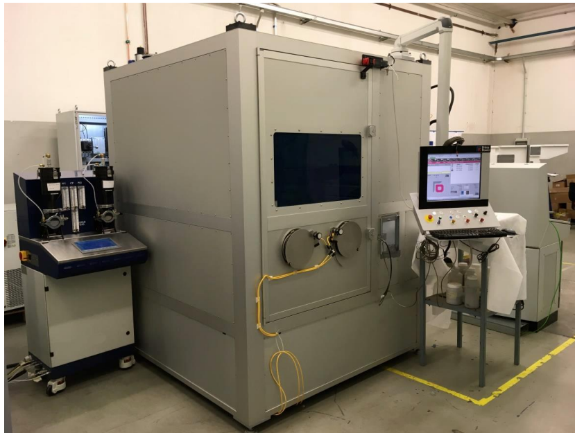
Fig. 3.1 DED machine prototype in Prima Industrie [48]
