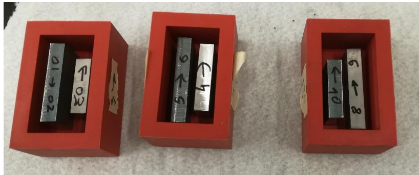
Fig. 3.9 Rubber moulds used to mount samples in resin. Keeping trace of the sample ID number is crucial.
