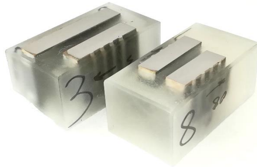
Fig. 3.11 SST mounted in resin and polished
