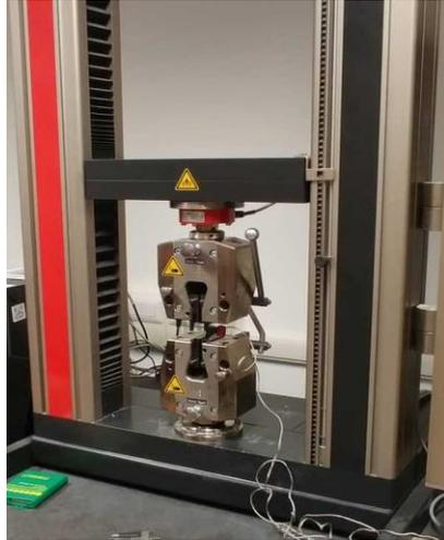
Figure 31: Zwick Roell -Ulm Germany Z050 tensile-tester.
