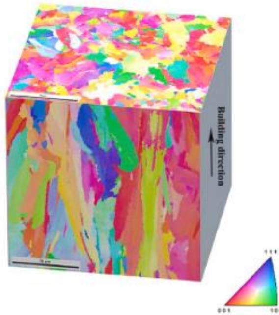
Figure 18: Electron backscatter diffraction (EBSD) scan of an Inconel 718 sample produced by LPBF. It can be noticed that grains are elongated through the building direction (z axis) while are irregular in the plane x-y [37].
