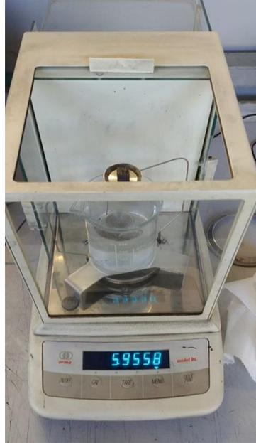
Figure 25: Analytic balance for Archimedes' method.
