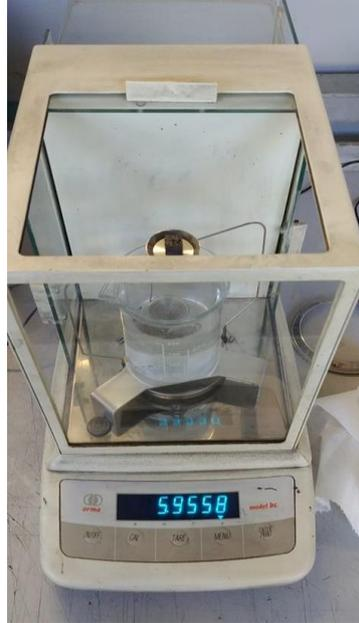
Figure 25: Analytic balance for Archimedes' method.
