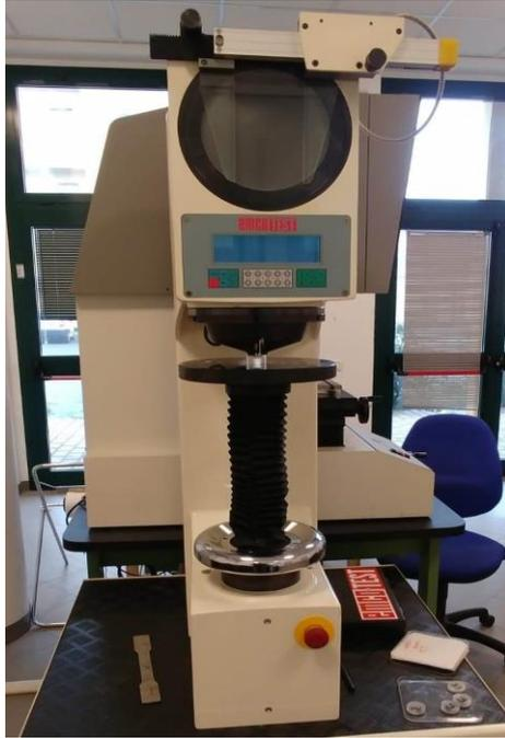
Figure 30: EMCO TEST M4U hardness test machine.
