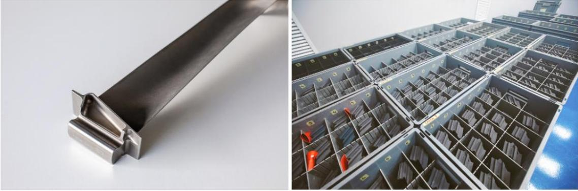
Figure 11: Turbine blades made of TiAl produced via EBM by Avio Aero [26].
