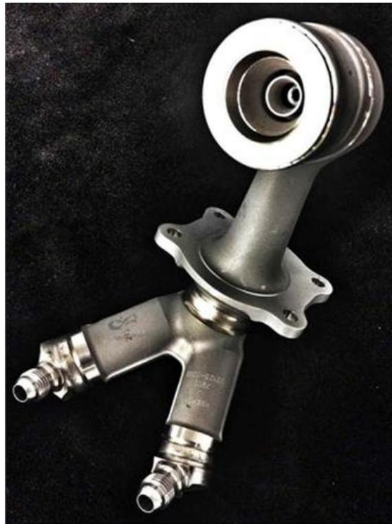
Figure 10: GE Leap Engine fuel nozzle created using laser powder bed fusion via the EOS metal powder bed fusion machine [1].
