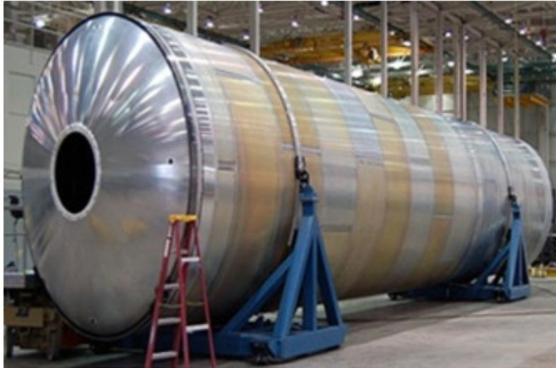
**Figure 3.12:** Aluminum-Lithium (Al-Li) cryogenic tank [15]
