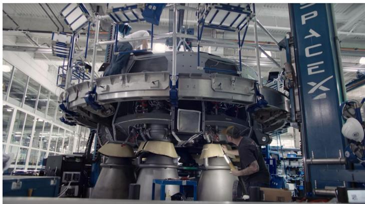
**Figure 3.11:** Falcon 9 thrust structure and engines. *Courtesy of SpaceX*
