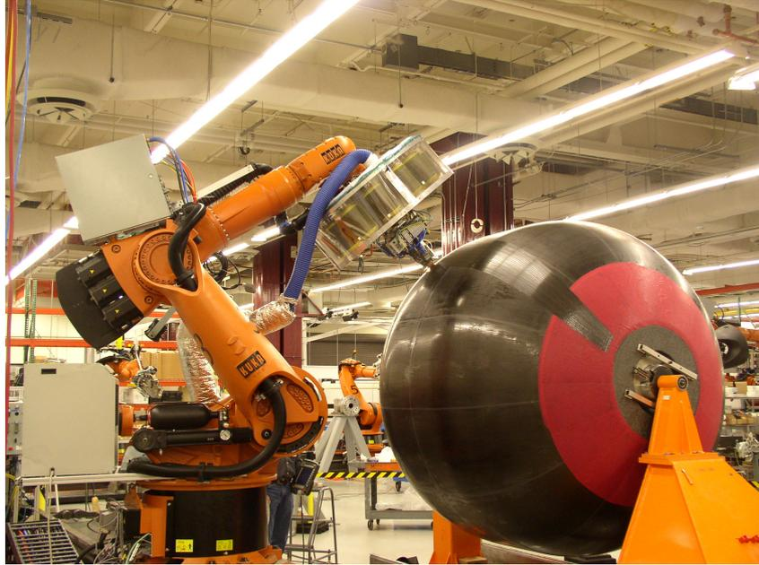
**Figure 3.13:** Example of composite-fibre cryogenic tank from NASA [16]
