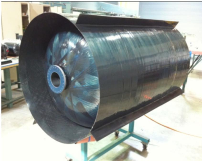
**Figure 3.14:** Example of subscale composite-fibre cryogenic tank [17]
