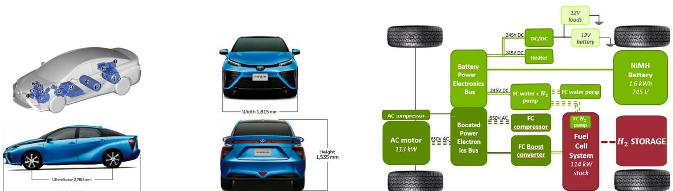
Figure 6.1 – Toyota Mirai dimensions and components distribution
