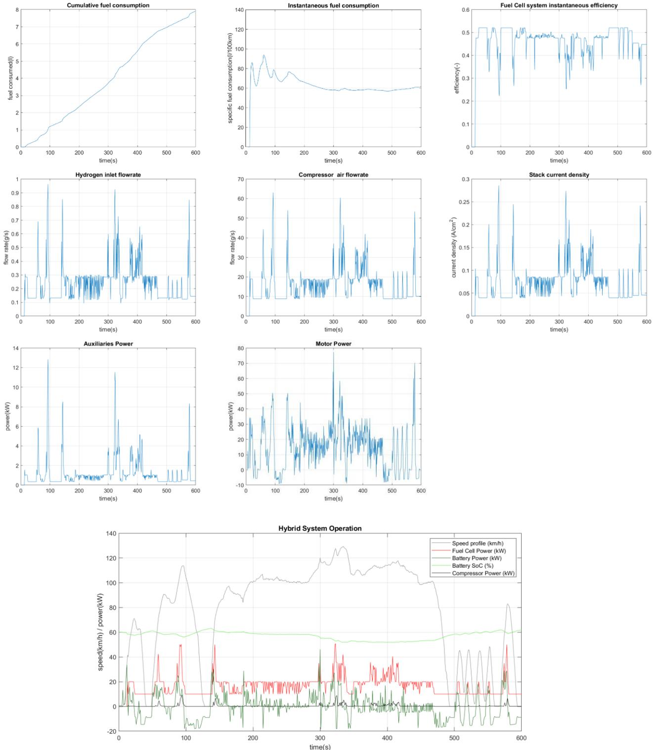
Figure 5.30 – Results on US06 driving cycle: a) Cumulative consumption b) Instantaneous specific consumption c) Fuel cell system efficiency d) Hydrogen flowrate e) Air flowrate f) Current density g) Auxiliary system power h) Motor power i) Hybrid system operation
