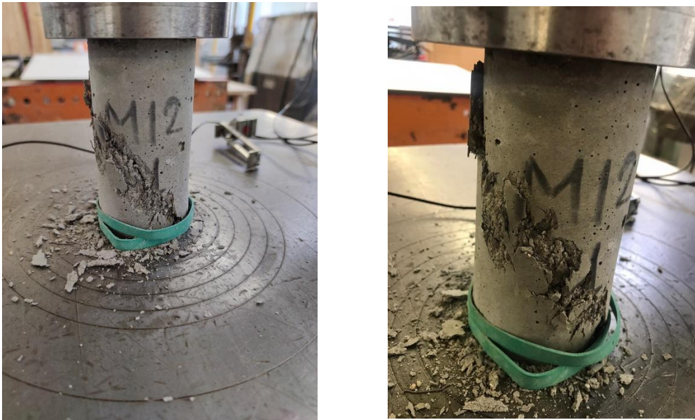
Figure 33 Failure of the specimens subjected to compressive load
