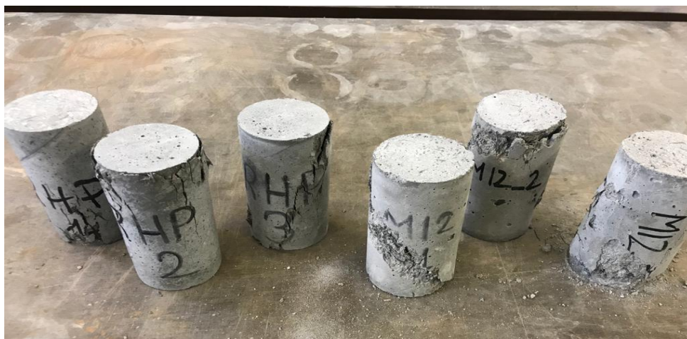
Figure 38 The sets of mix Resilia HP and 12 specimens subjected to the compression loading
