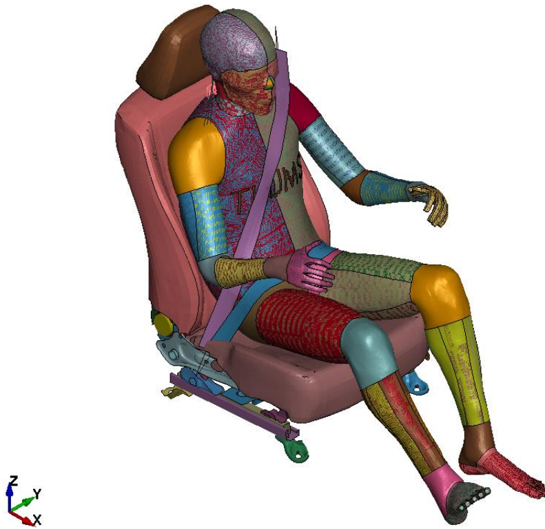
Figure 6.4: THUMS with Seatbelt
