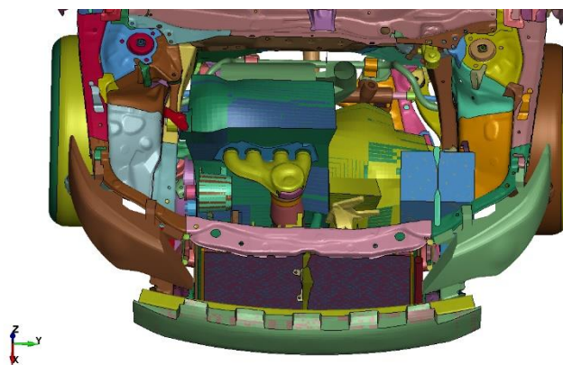
Figure 3.15: FE Model - Engine Bay Detail
