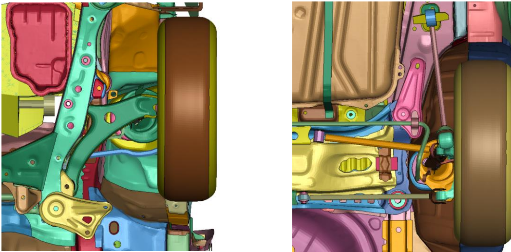
Figure 3.17: FE Model - Front (LEFT) and Rear (RIGHT) Suspension Detail
