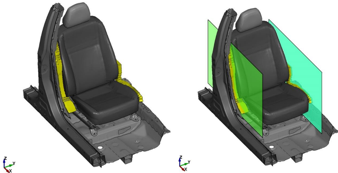
Figure 3.31: Passenger seat spacers: Position detail (LEFT); Section Planes (RIGHT)
