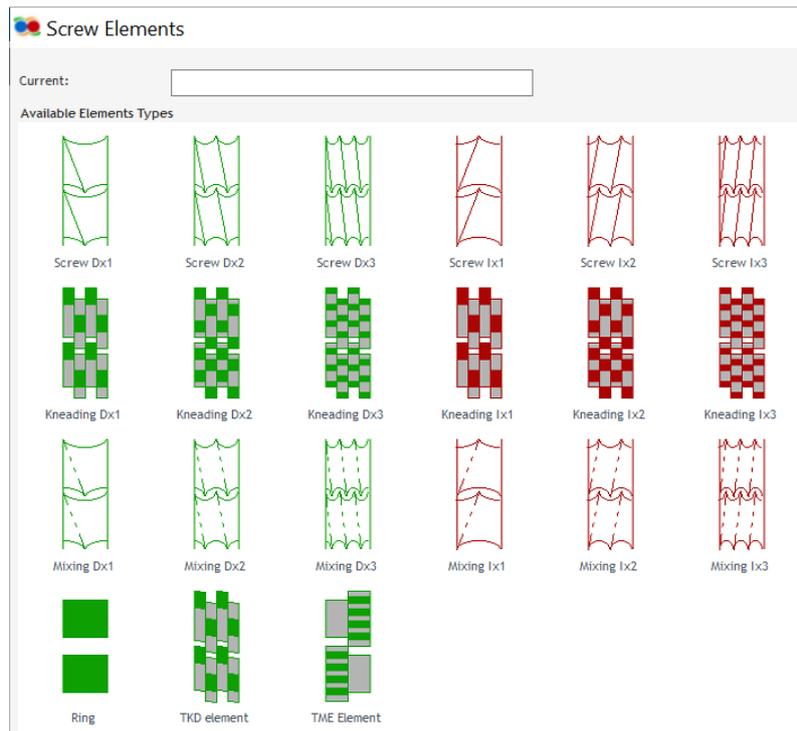
Figure 93. Screw elements available in Ludovic software.
