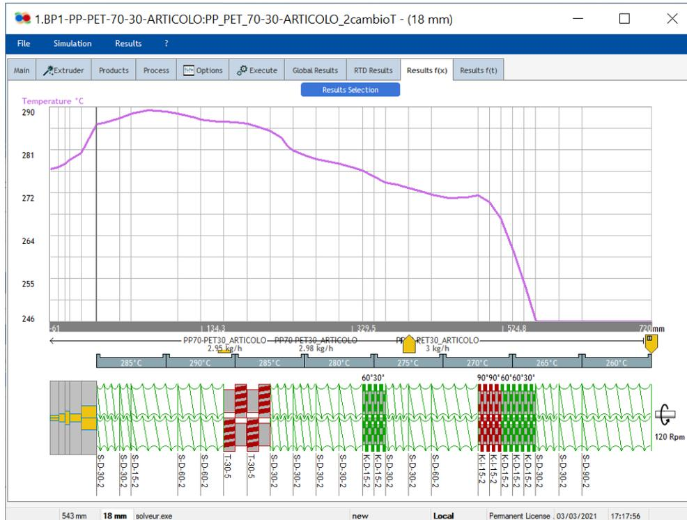
Figure 128. Temperature graph for 70% PP and 30% PET, at 120rpm and with the modified profile temperature.
