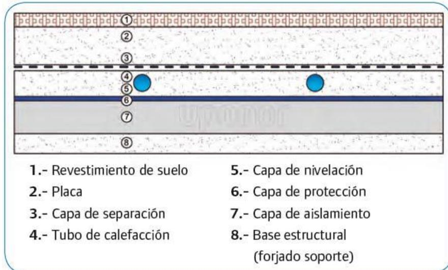
Figure 8. Radiant floor structure type D
