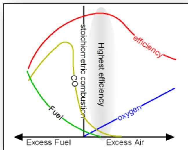
Figure 11. Combustion efficiency diagram
