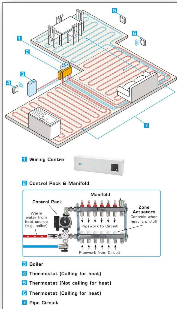
Figure 2. System Components
