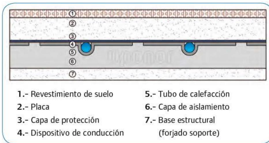
Figure 7. Radiant floor structure type B
