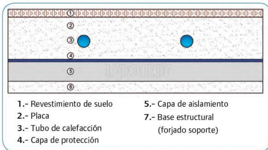
Figure 6. Radiant floor structure type A and C
