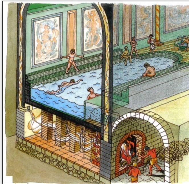
*Figure 1. Hypocaust heating system*
