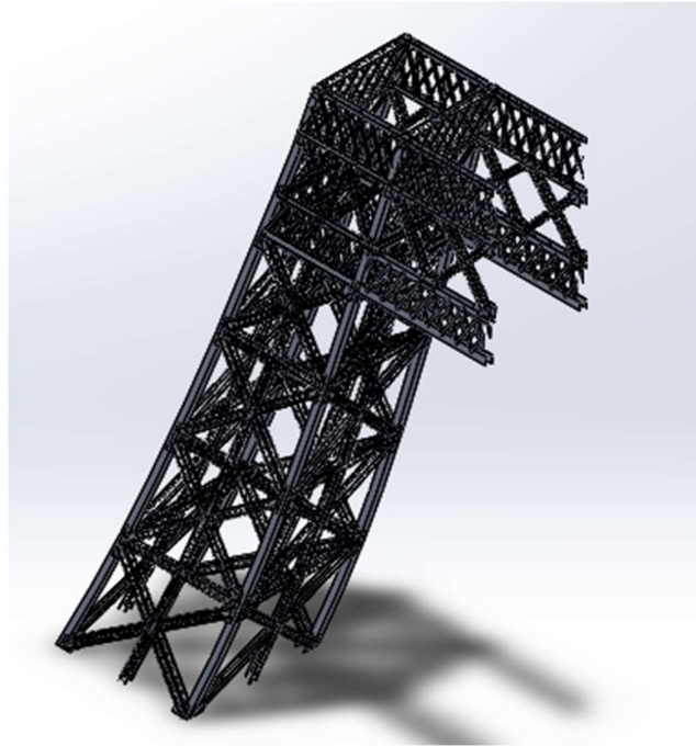
Fig. 30 Crossbars Assembled in Intermediate Stage
