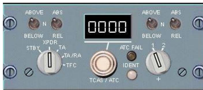
Figura 5.12: *TCAS/ATC Transponder Control Panel* Airbus A320
