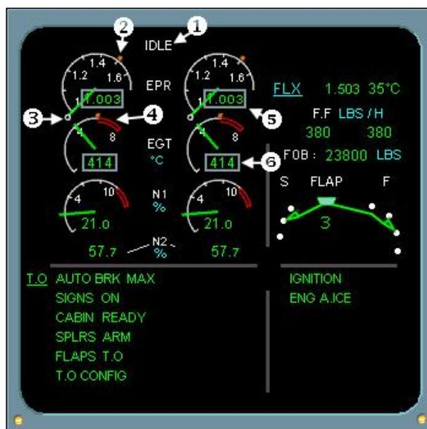
Figura 5.6: ECAM\_E/WD (Engine Warning Display)
