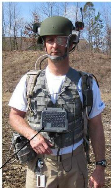
**Figura 1.2:** Augmented reality system, ULTRA-Vis
