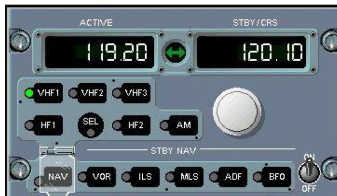
**Figura 5.11:** Radio Management Panel Airbus A320
