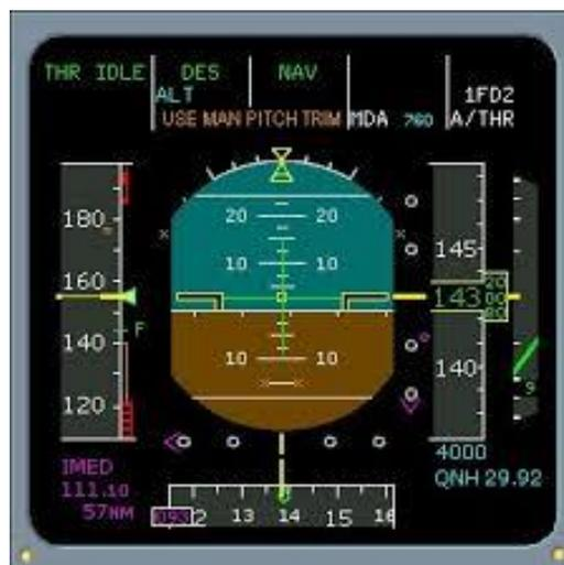
Figura 5.5: Primary Flight Display Airbus A320
