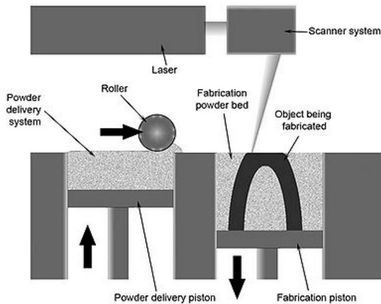
*Fig. 10. Powder bed fusion process*
