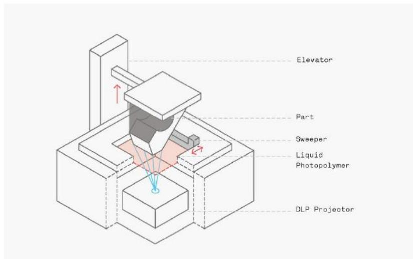
*Fig. 8. Schematic of DPL printer*
