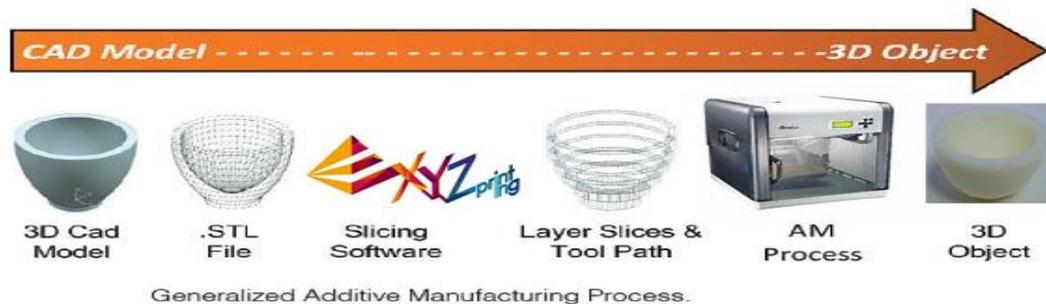
*Fig. 1. Generalized Additive Manufacturing process*
