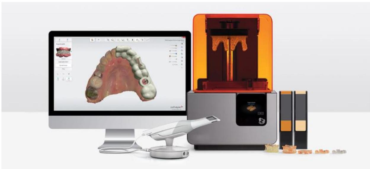
*Fig. 34. Intraoral scanner and 3D printing devices*
