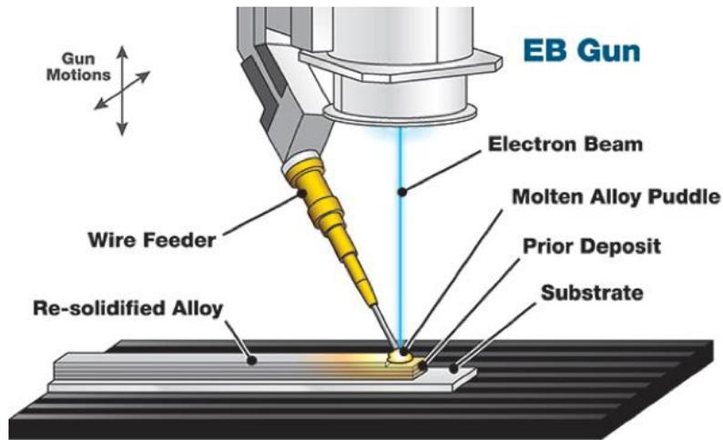
*Fig. 11. Direct Energy Deposition*
