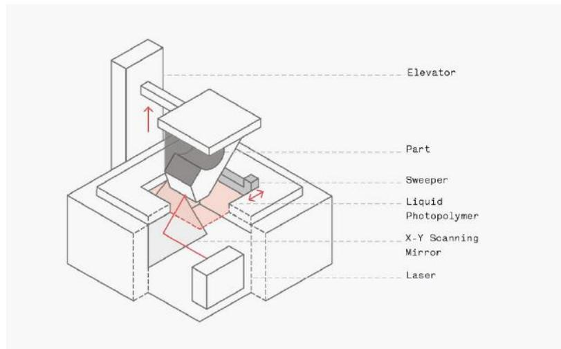
*Fig. 7. Schematic of SLA printer*
