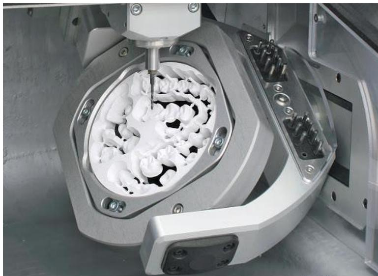
*Fig. 39. Milling machine for dental applications*
