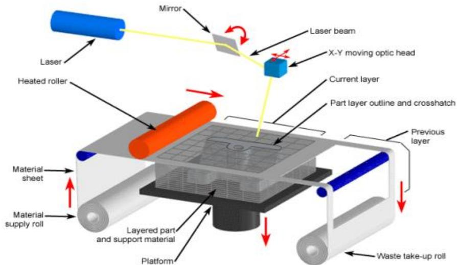
*Fig. 5. Laminated object manufacturing*
