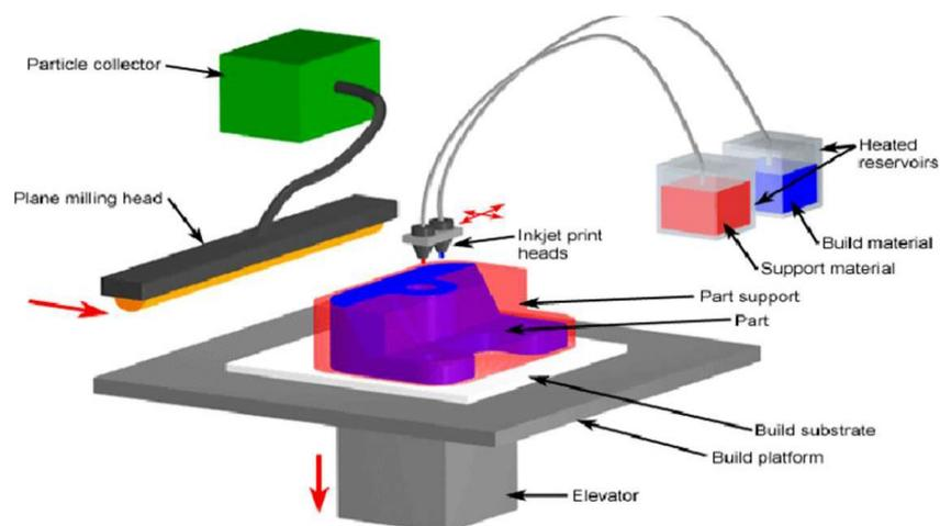
*Fig. 3. Material Jetting process*
