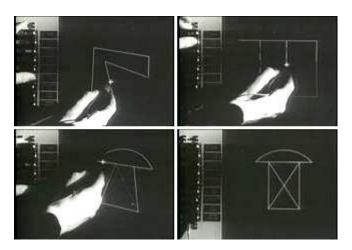
Sketchpad was the first program that revolutionized the methods of interaction with computers and was the predecessor of the current graphics programs, introducing the concept of direct manipulation and that of metaphor. Sketchpad allowed instances of geometries, snap and even three-dimensional parametric modeling
