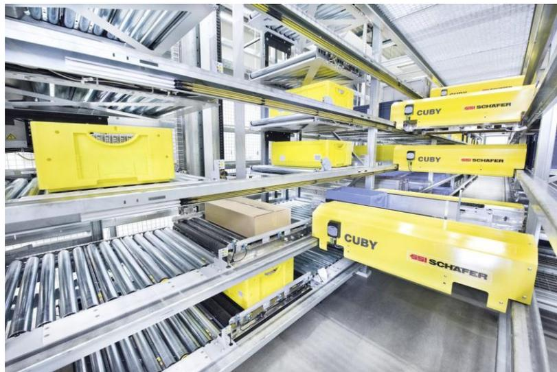
**Figure 2.3** - Shuttle-based storage and retrieval system
