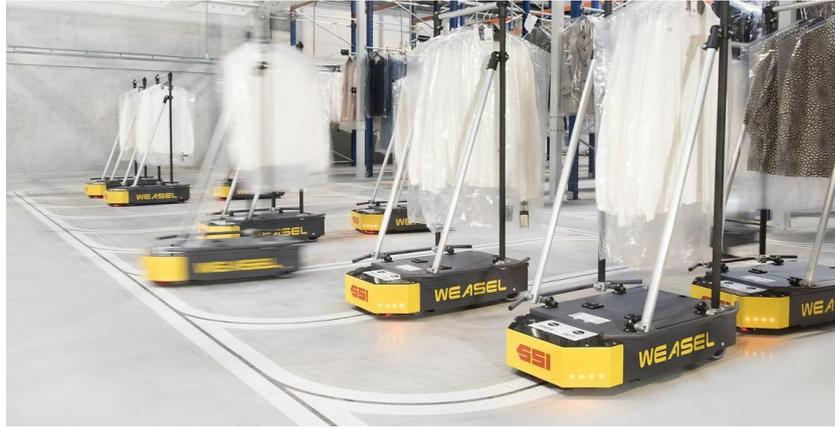
**Figure 2.5** - Automated Guided Vehicles (Unit load handlers)
