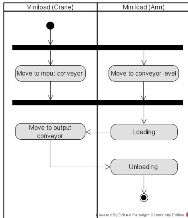
**Figure 5.4 - Transfer activity diagram**
