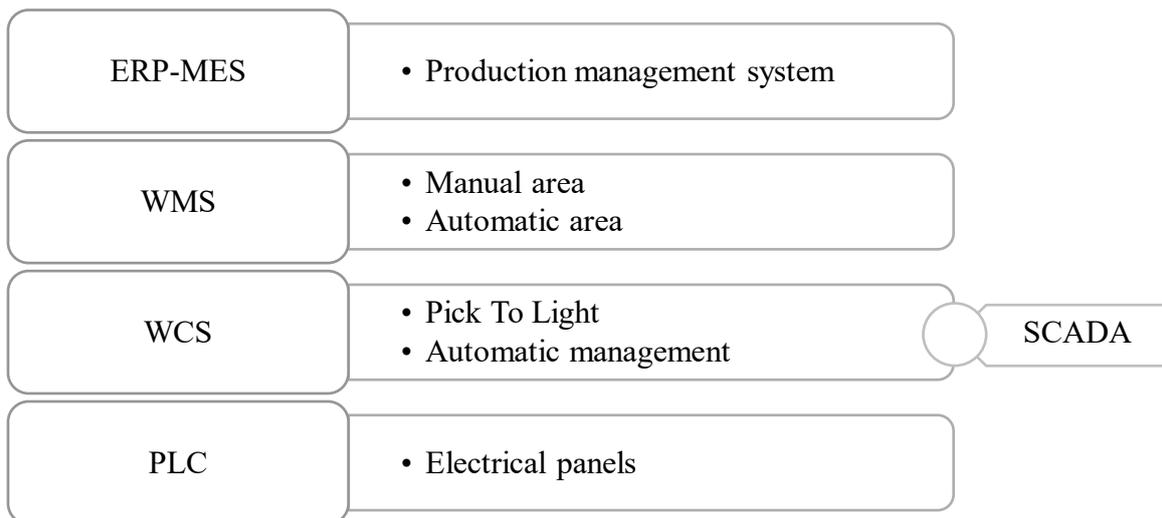
**Figure 4.5** - IT structure of the automatic warehouse
