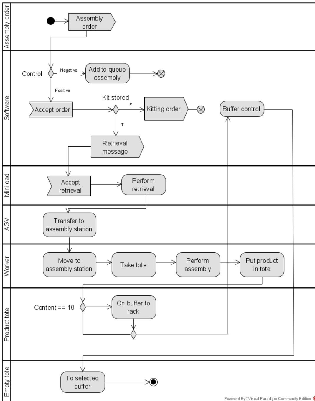
**Figure 5.8** - Assembly activity diagram
