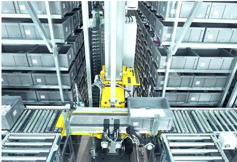
**Figure 2.2** - Mini-load stacker crane
