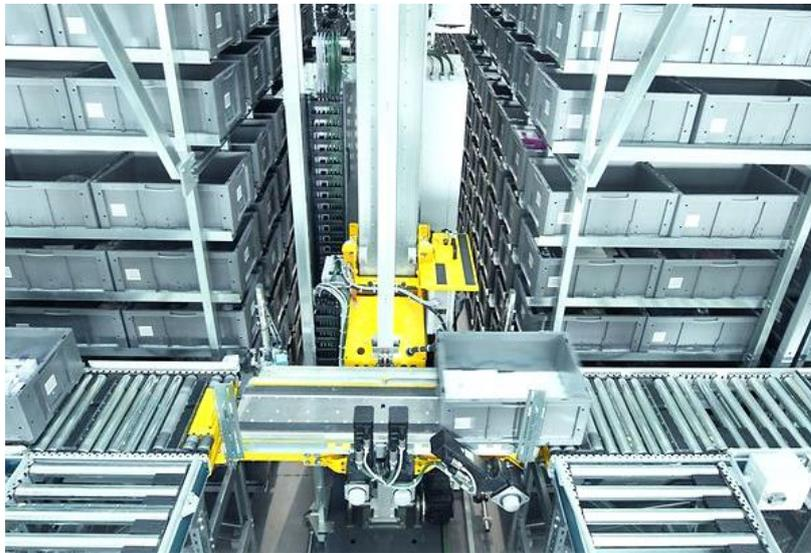
**Figure 2.2** - Mini-load stacker crane
