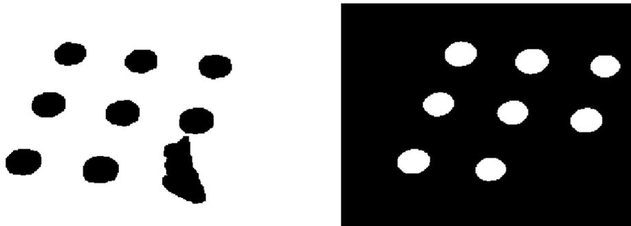
**Figure 5.25:** Left: board before applying the morphological filters, right: board after applying the morphological filters.
