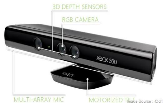
**Figure 4.2:** The RGB-Depth Microsoft Kinect v.1 camera is equipped with RGB sensor, an IR depth sensor and an IR projector. From [40]
