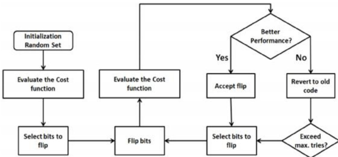
We want both balanced and minimum auto-correlation side-lobe properties for our spreading sequences. We set these properties as initial necessities for the initial set of sequences but after some of the bits have been flipped, those characteristics could not be kept.
