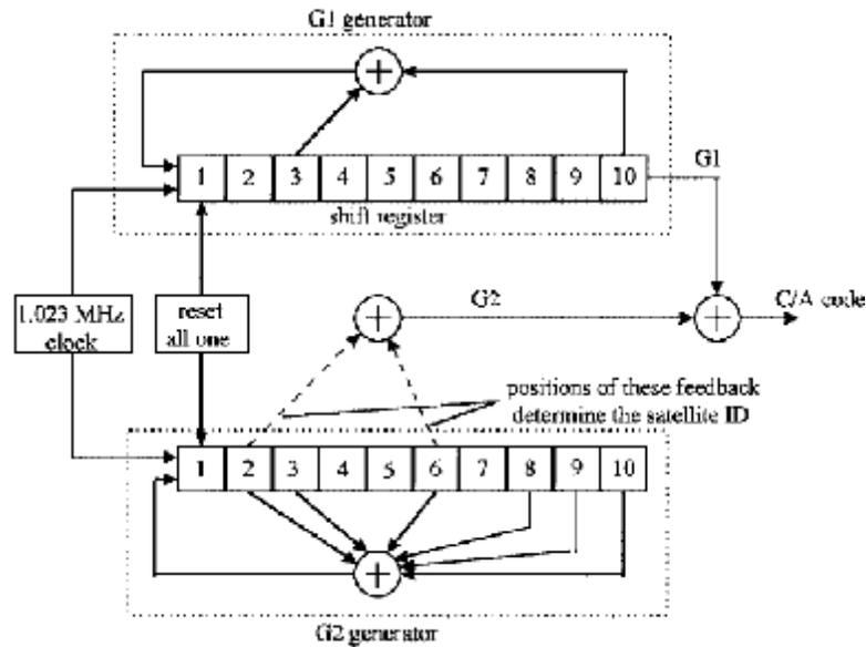
We pick two maximum length sequences of the same length  $2^n - 1$ , where  $n$  is the size of the LFSR used to generate the maximum length sequence. It can be written also as two polynomials, where the powers correspond to the index of registers, having output to ex-or function. 32 different permutations of this indexes are taken to generate 32 unique PRN codes for each of 32 satellites that transmit data in GPS.
