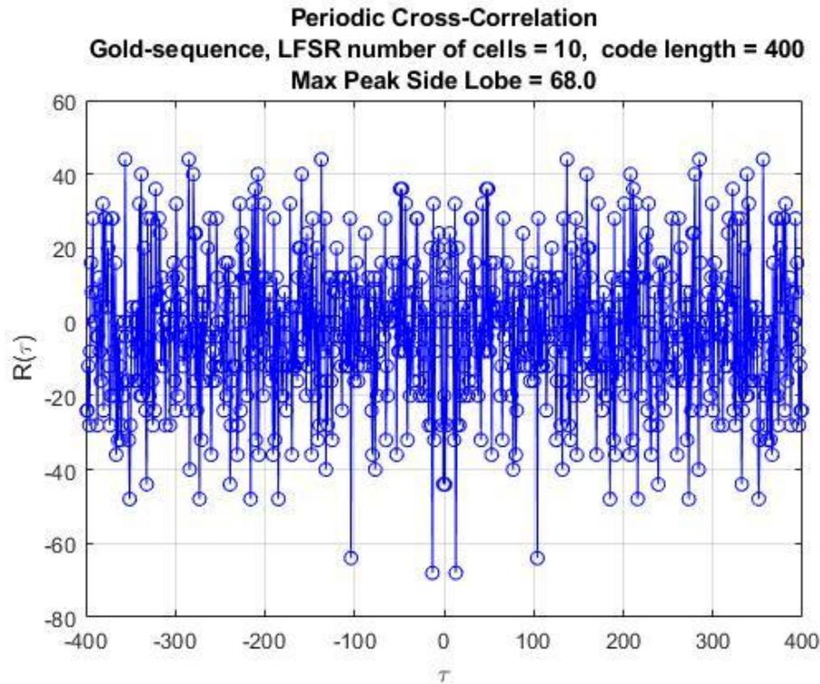
Note: In all four different lengths (1023,1000,700,400), we kept the number of cells fixed equal to 10 and a fixed initial seed value [0 0 0 0 0 0 0 0 1].
