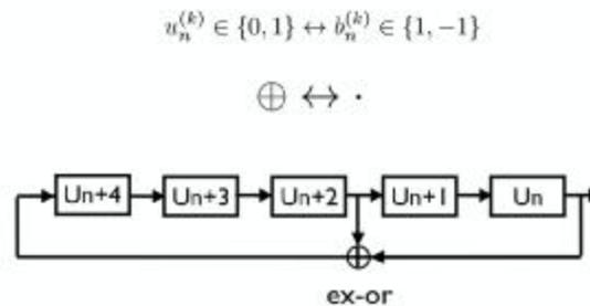
In figure 2.1,  $n$  represents the time index and  $+$  is modulo-2 addition which corresponds to the ex-or when bit values are 0 or 1. Initial state of the registers can be any state except for the all zero state. The reason is that m-sequences are periodic and shift registers are able to cycle through every possible binary value (except for the all zero vector). It is common to describe the design of linear sequence generators by means of polynomials of the form: [3]
