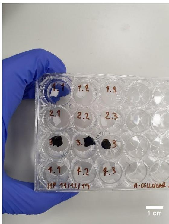
**Figure 2.1:** Digital photo of the cylindrical hydrogel samples used for the water uptake test in triplicate. This photo was taken at the end of the test. Samples shown from the top to the bottom of the image are: GG3(1), GG2(2), GG/GEL(4). Scale bar = 1cm.
