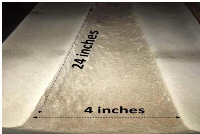
Fig. 4.22: Clean large hole created by Laser perforation
