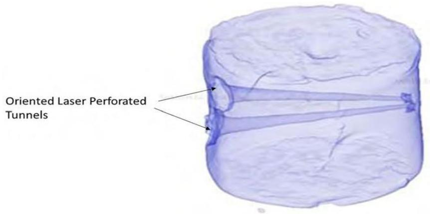
Fig. 4.14: CT-scan of the unconsolidated sand core shows multi laser perforation
