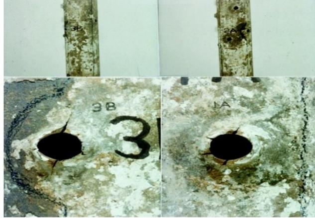
Fig. 2.1: Casing perforated by a bullet in a surface test.
