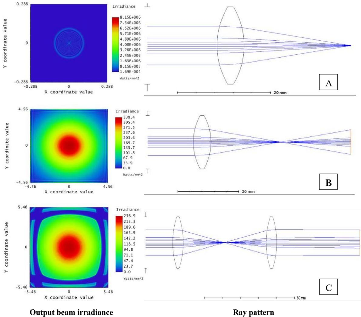
Fig. 4.19: Light focusing (A), after focusing (B) and collimation (C) using a bi-convex lens (adopted from batarseh 2019a)
