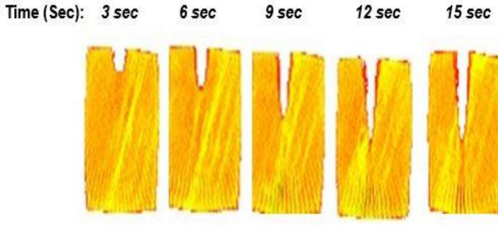
Fig. 4.13: CT Scan shows Lasing Time effect on depth of Penetration in Berea Sandstone
