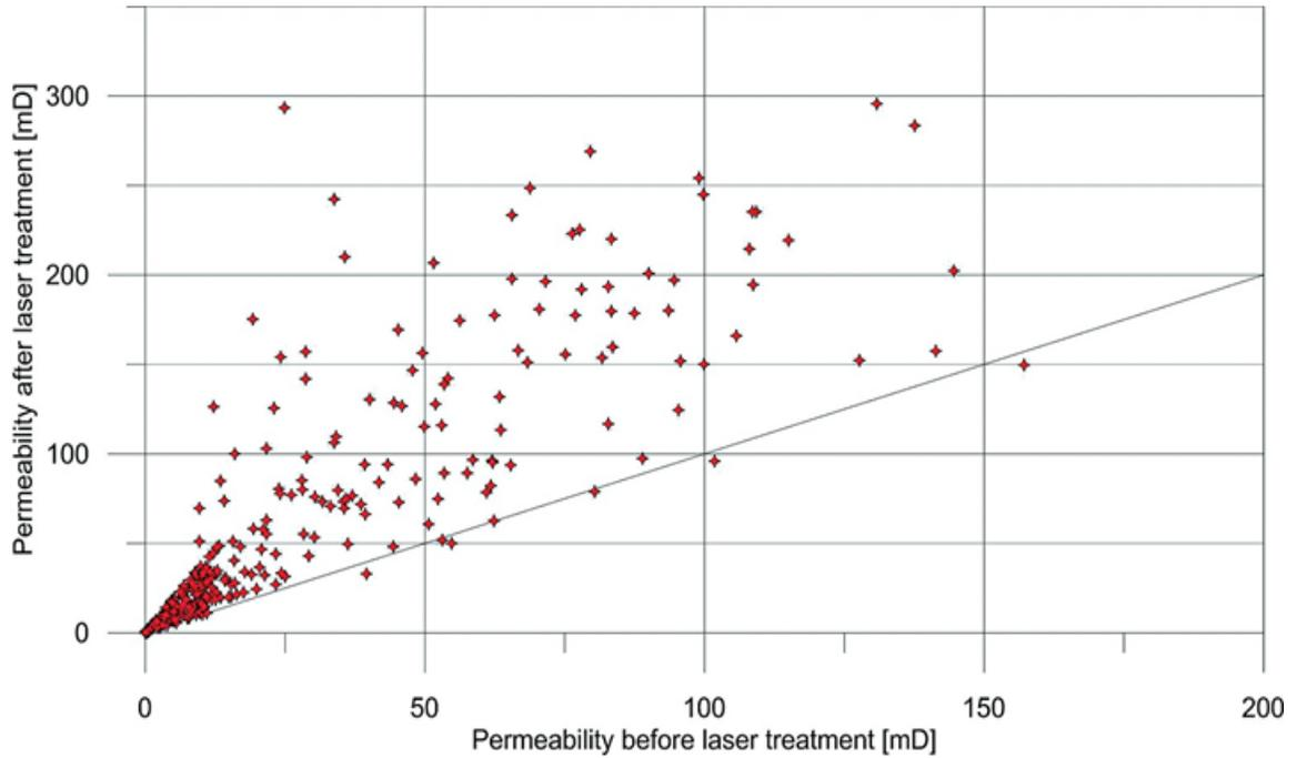
Fig. 4.23: Increases of Induced permeability as a result of heat shock fracturing due to drilling by laser
