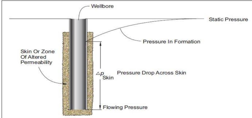
Fig. 3.9: Distribution of pressure in a reservoir with existing of Skin
