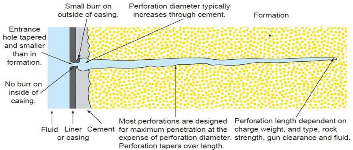
Fig. 3.1: Geometry of perforation
