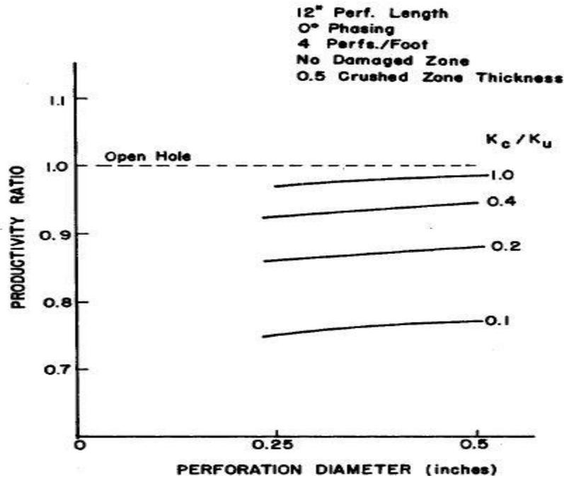
Fig. 2.15: Productivity ratio versus perforation diameter (Locke, 1981)
