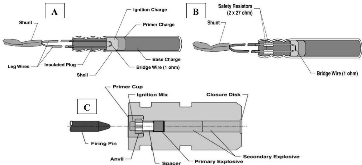
Fig. 2.4: Detonator types
