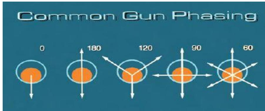
Fig. 2.16: Mostly used charge phasing (King, 2007)
