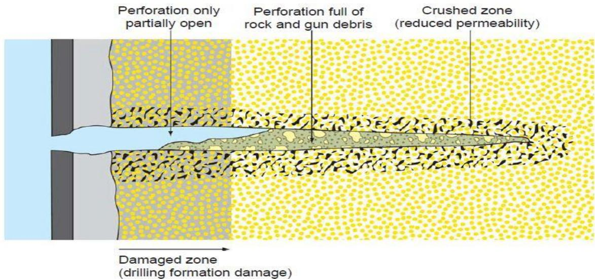
Fig. 2.11: hole immediately after perforation.
