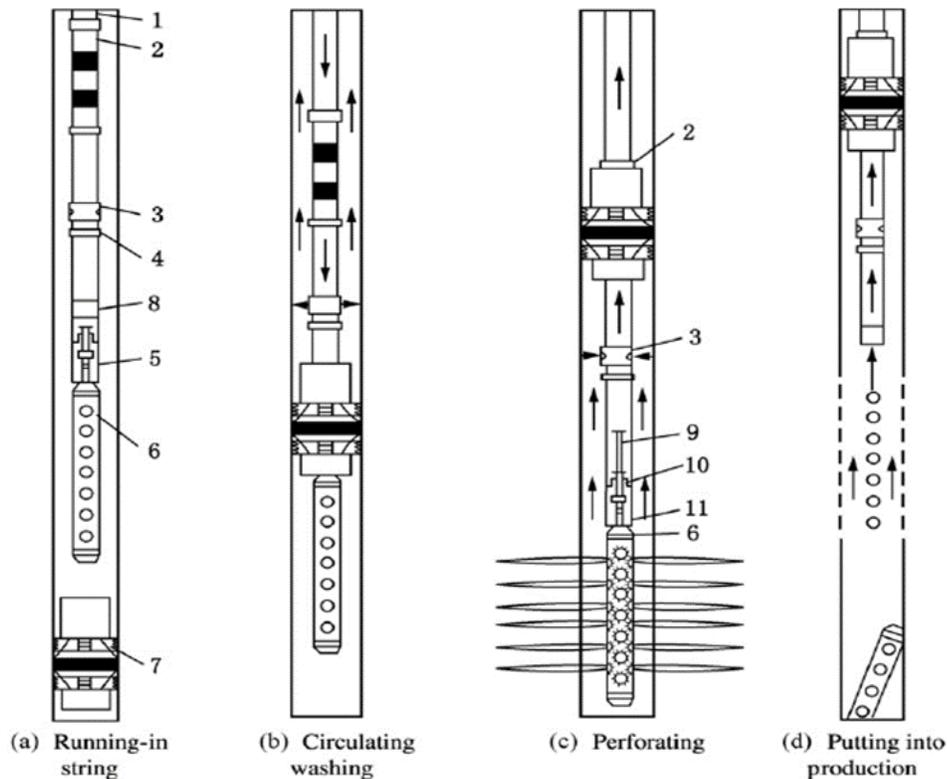
Fig. 2.10: Combined technology for TCP and placing on production. 1, tubing; 2, seal assembly; 3, circulating sub disc type; 4, tubing collar; 5, gravity detonation head and releasing device; 6, perforating gun; 7, packer; 8, guide sub; 9, bar; 10, impact; 11, detonator.
