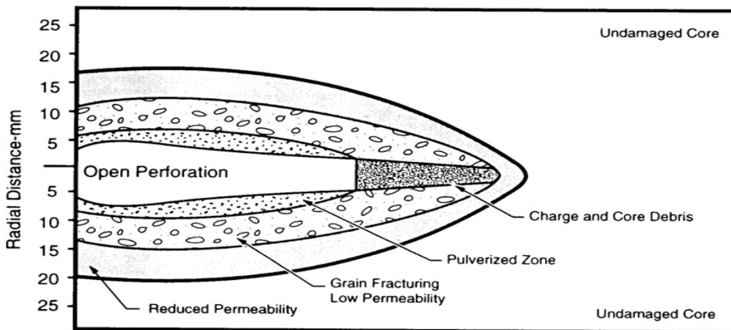
Fig. 3.5: Perforation damage type (McElfresh et al., 2004).
