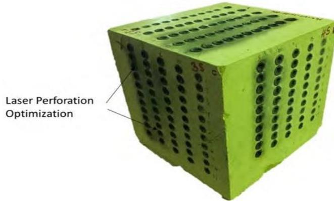
Fig. 4.7: Example of multiple perforations made on Yellow limestone (LSSY) for optimization and development.
