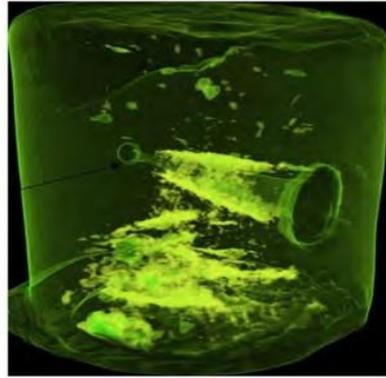
Fig. 4.11: CT-scan in unconsolidated sand laser perforation
