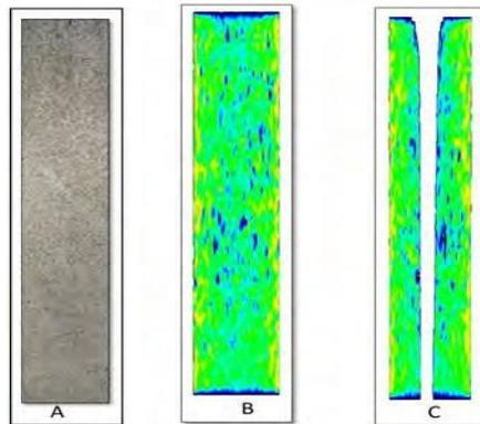
Fig. 4.9 CT Scan indicating a Yellow limestone rock before and after laser perforation. A: the rock top region, B: CT scan before perforation, C: CT scan after perforation.
