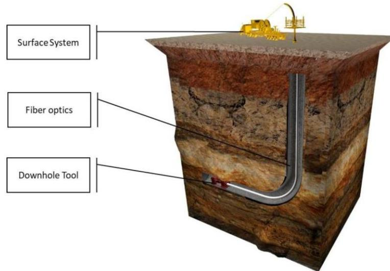
Fig. 4.15: HPL system components for field operations (Sameeh Batarseh et al., 2018)
