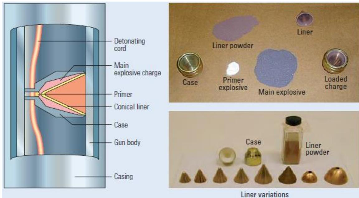
Fig. 2.5: Shaped charge (Baumann et al., 2014).
