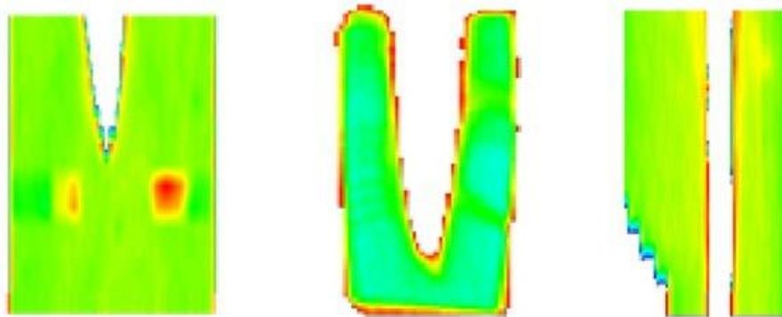
Fig. 4.10: CT scans displays various hole shapes in various rocks
