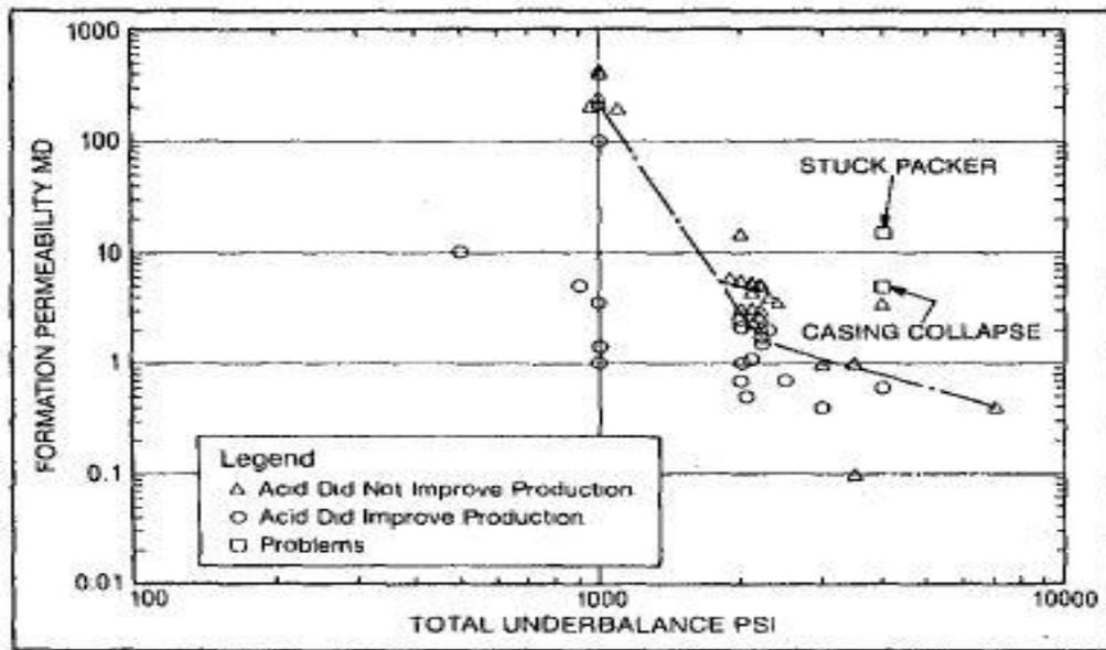
Fig. 2.12: Underbalanced pressure used on TCP in sandstone gas zones (King et al., 1986)
