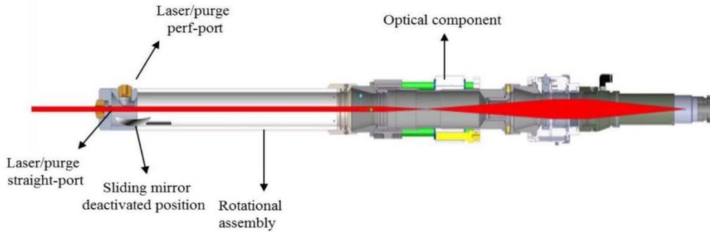
Fig. 4.20 Showing straight beam orientation mode in Laser perforation gun
