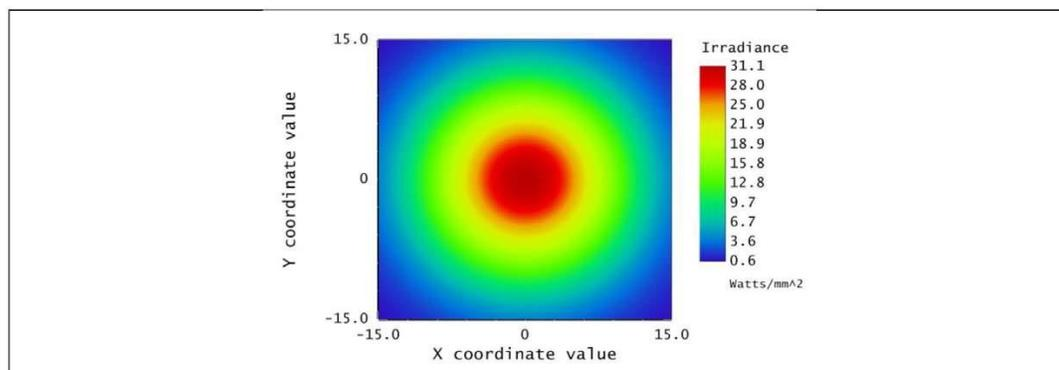
Fig. 4.18: Gaussian beam irradiance with a beam waist of 30 mm
