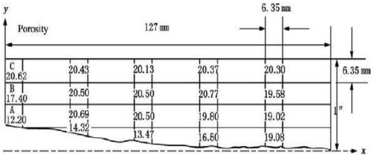
Fig. 3.6: Distribution of porosity (%) around perforation (Asadi & Preston, 1994)
