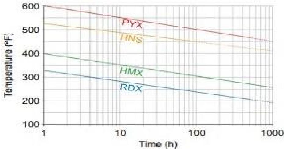
Fig. 2.6: stability temperature for perforating explosives
