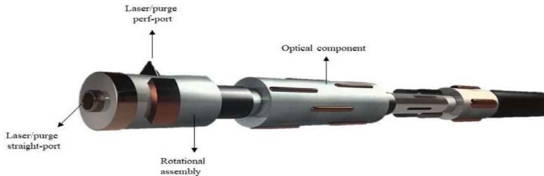
Fig. 4.17: The gun of Laser perforation two laser ports
