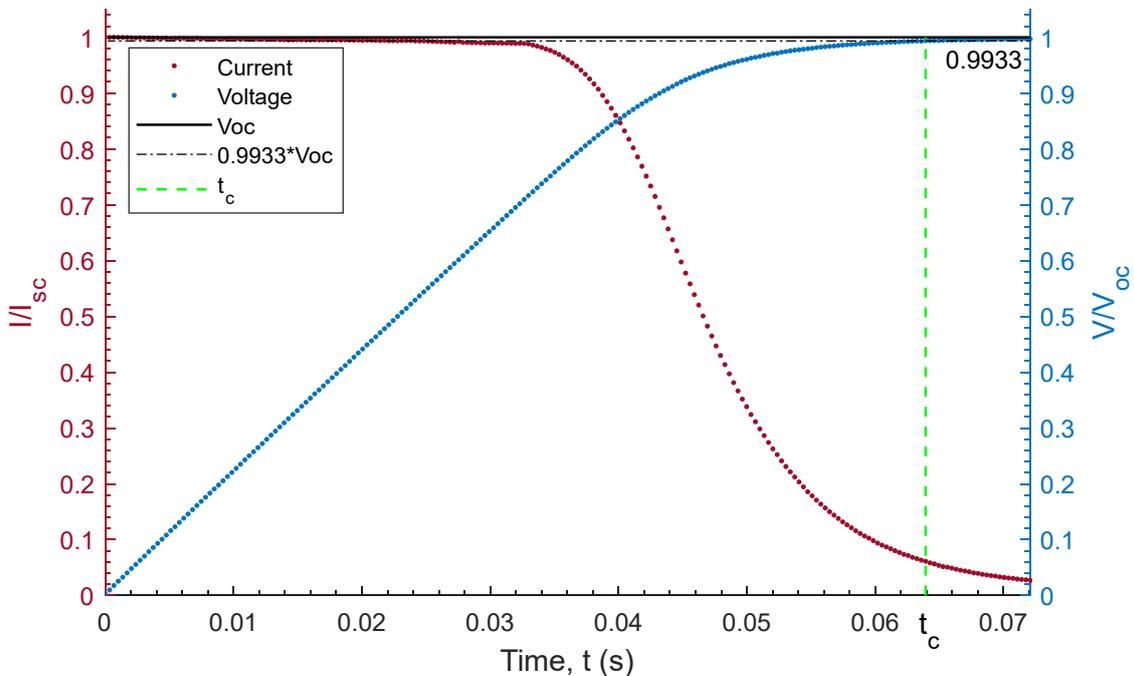
Figure 4.2: Charging transient of a capacitor connected with a PV module.
