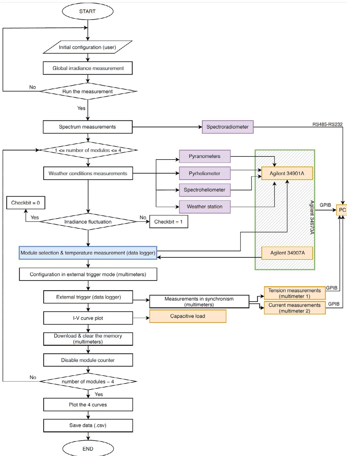
Figure 4.8: LabVIEW measurement control software flowchart
