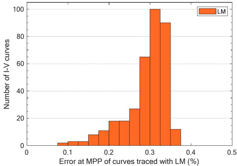
Figure 11.2: Distribution of the error at MPP for curves traced with LM method
