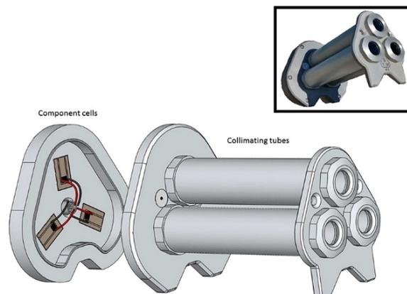
Figure 4.14: Picture of Tri-band spectro-heliometer from IES-UPM [27]
