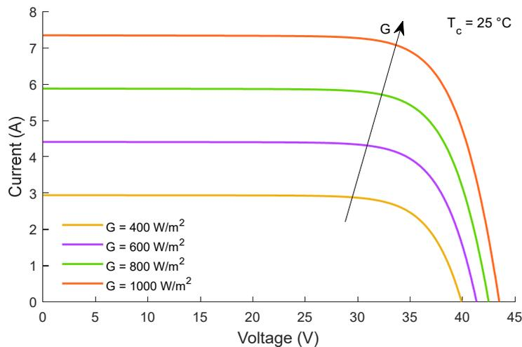
Figure 2.12: Dependence of the  $I$ - $V$  curve on irradiance
