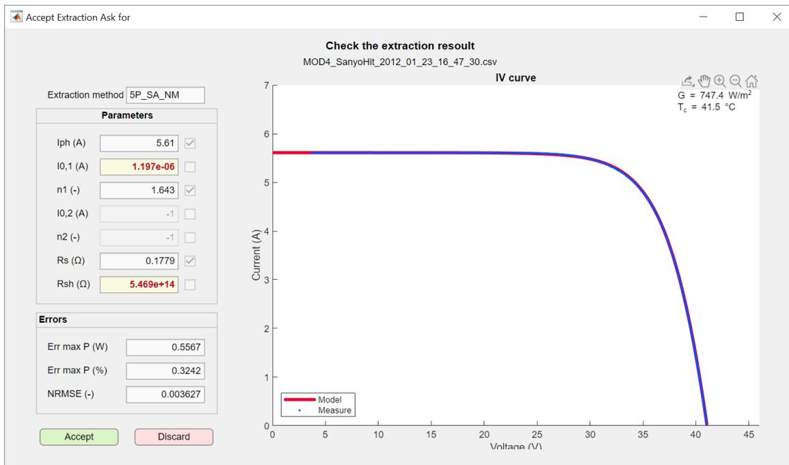
Figure 7.2: Picture of the “Parameters extraction result GUI”
