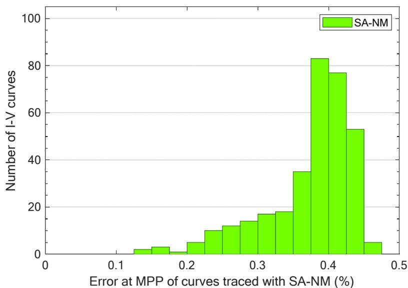
Figure 11.3: Distribution of the error at MPP for curves traced with SA-NM method
