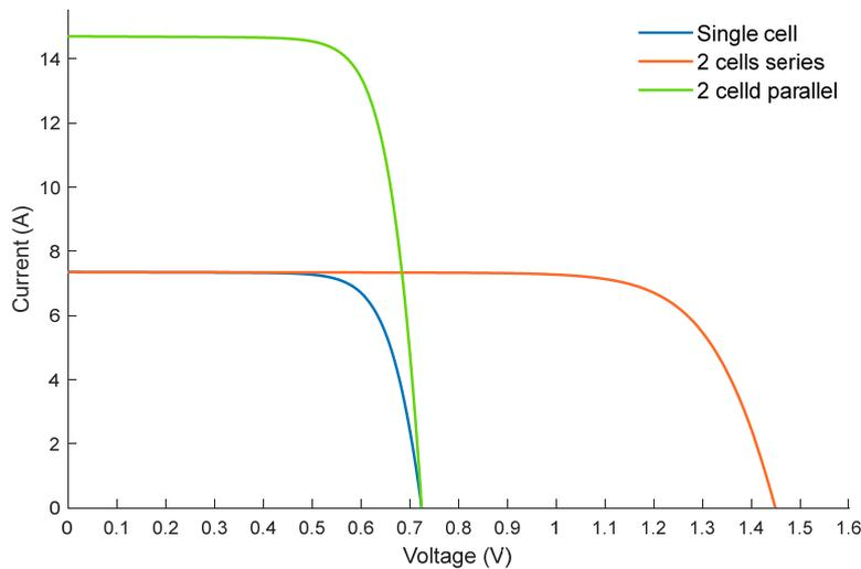
Figure 2.13: Series and parallel of equal  $I$ - $V$  curves
