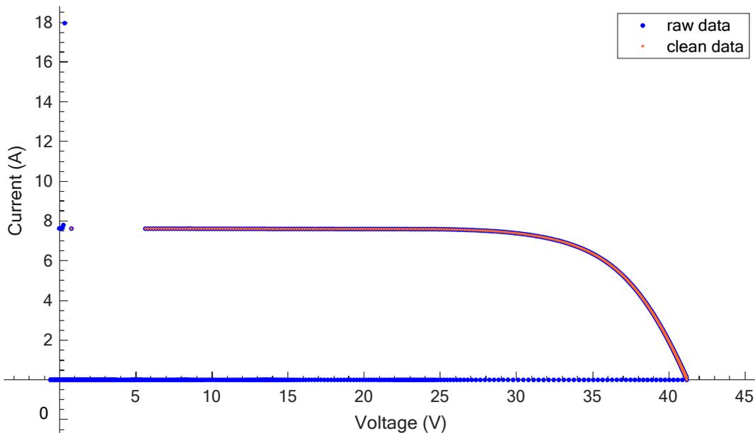
Figure 6.10: Extraction of the electrical quantities (in blue) from raw data (in orange)
