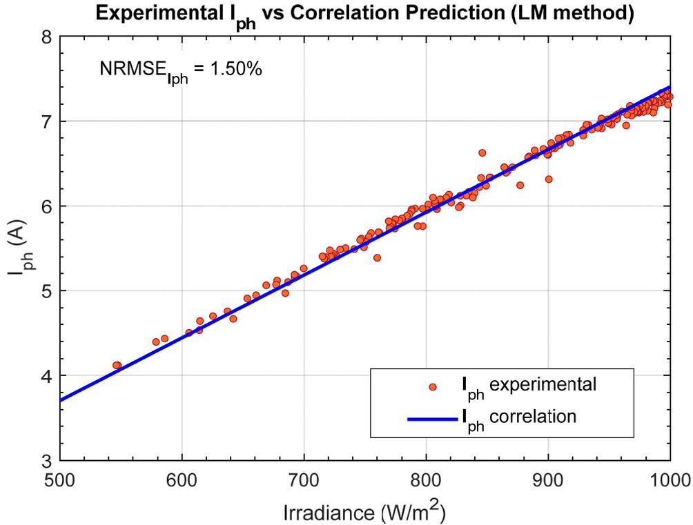
Figure 11.5:  $I_{ph}$  tendency with irradiance (LM algorithm)
