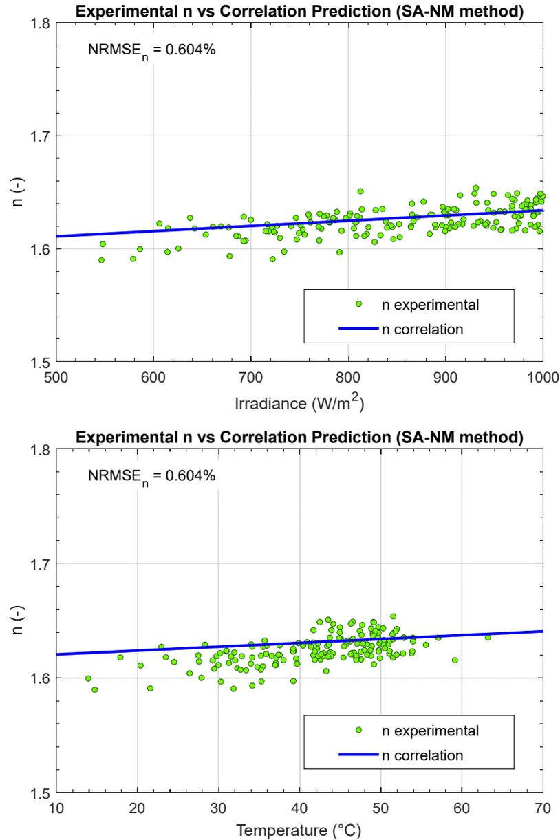
Figure 11.10:  $n$  tendency with irradiance and temperature (SA-NM method)
