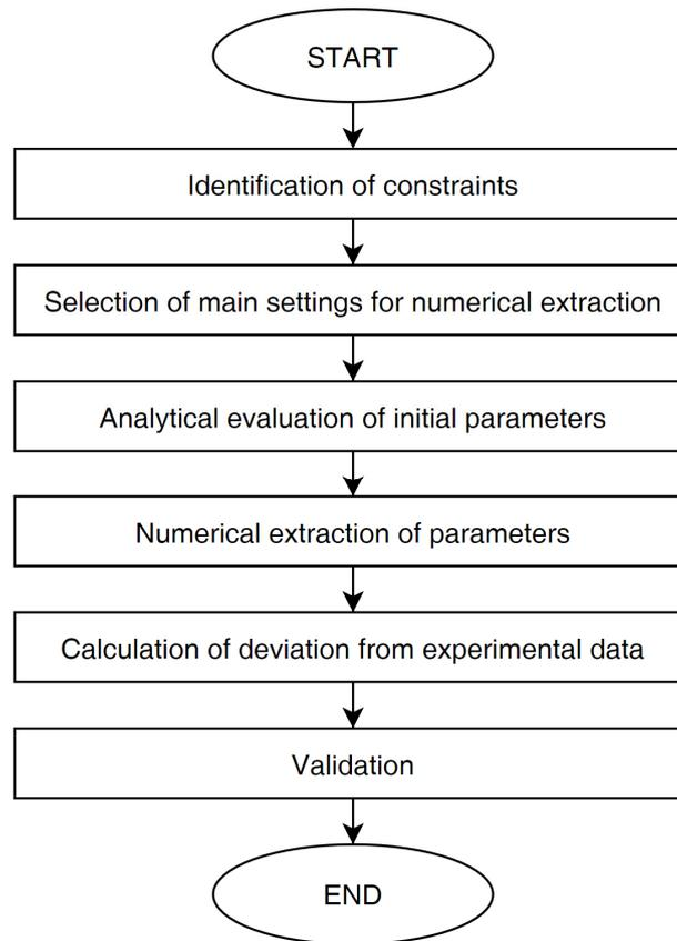
Figure 7.3: Flowchart of the parameters extraction procedure
