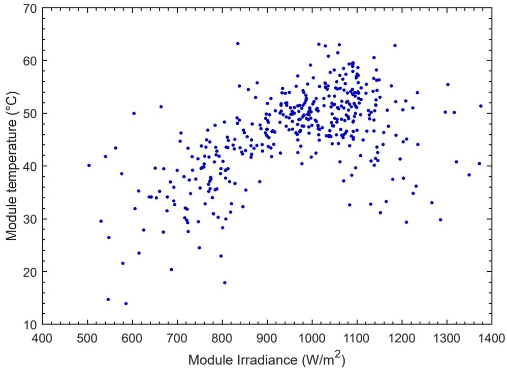
Figure 10.4: Irradiance and temperature of the  $I$ - $V$  curves for parameters extraction
