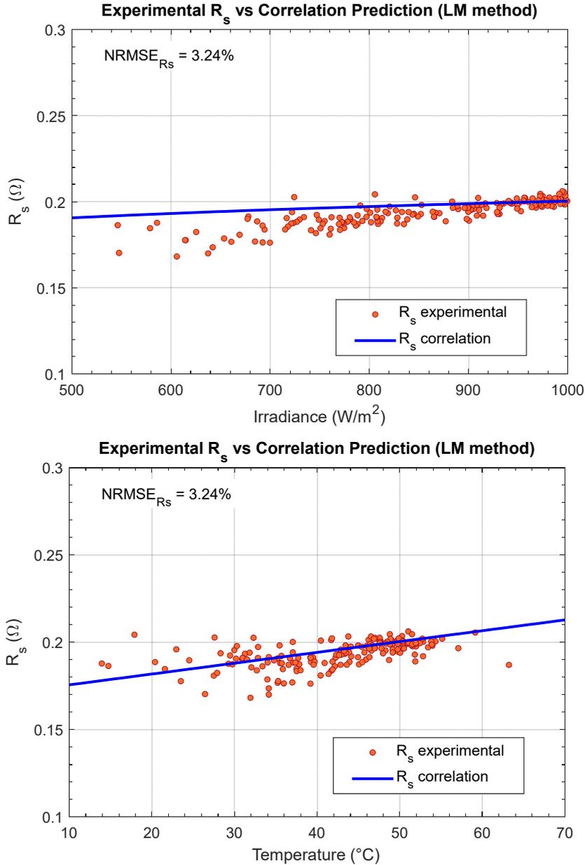
Figure 11.11:  $R_s$  tendency with irradiance and temperature (LM algorithm)
