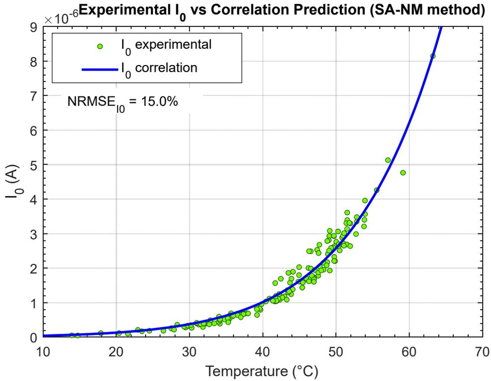
Figure 11.8:  $I_0$  tendency with temperature (SA-NM method)
