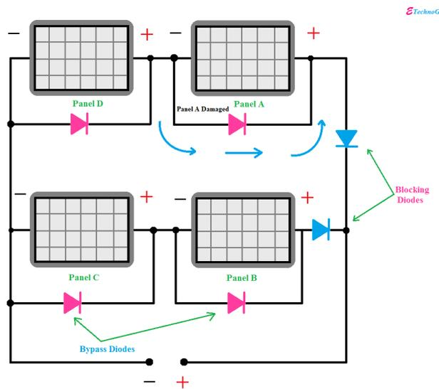
Figure 2.16: Bypass and blocking diodes [18]
