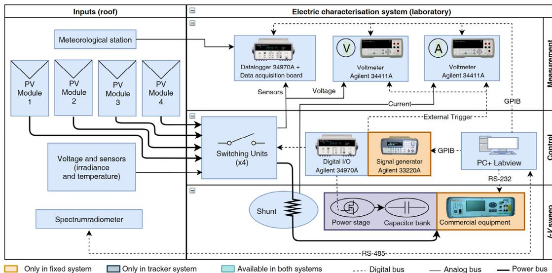
Figure 4.3: Global scheme of the measurement systems
