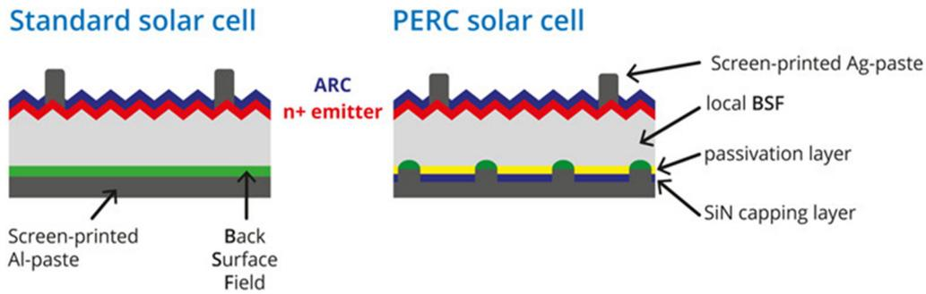
Figure 2.5: Detail of a PERC cell's layer [10]
