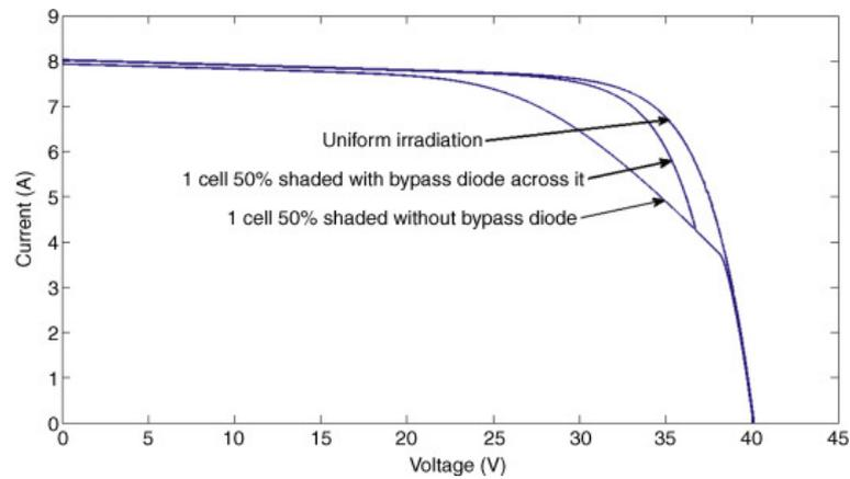
Figure 2.14: Series connection of cells with different  $I$ - $V$  characteristics [15]
