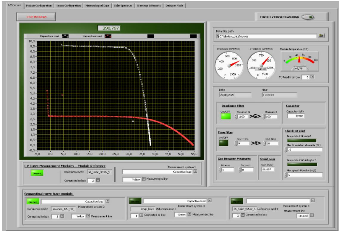
Figure 4.7: LabVIEW graphical user interface of tracker system (*I-V*-curve tab)
