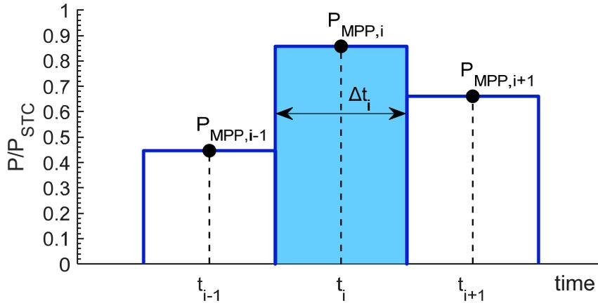
Figure 9.2: Computation of the integration time
