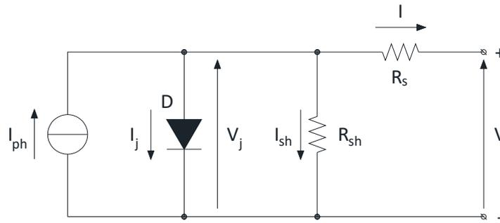
Figure 2.17: Five-parameters circuit model
