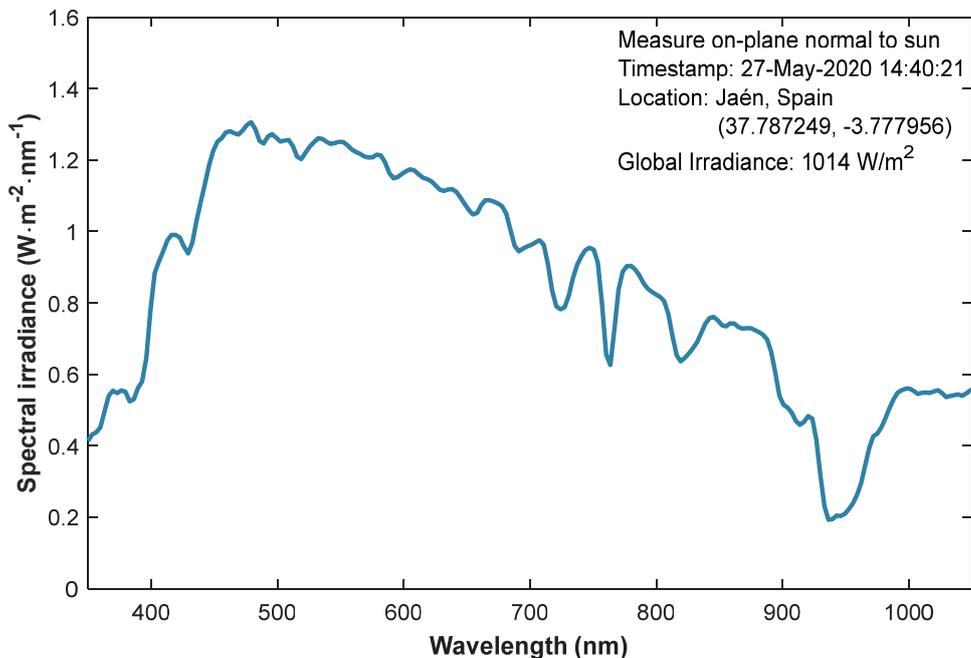
Figure 4.12: Spectral irradiance distribution measured by EKO MS-700
