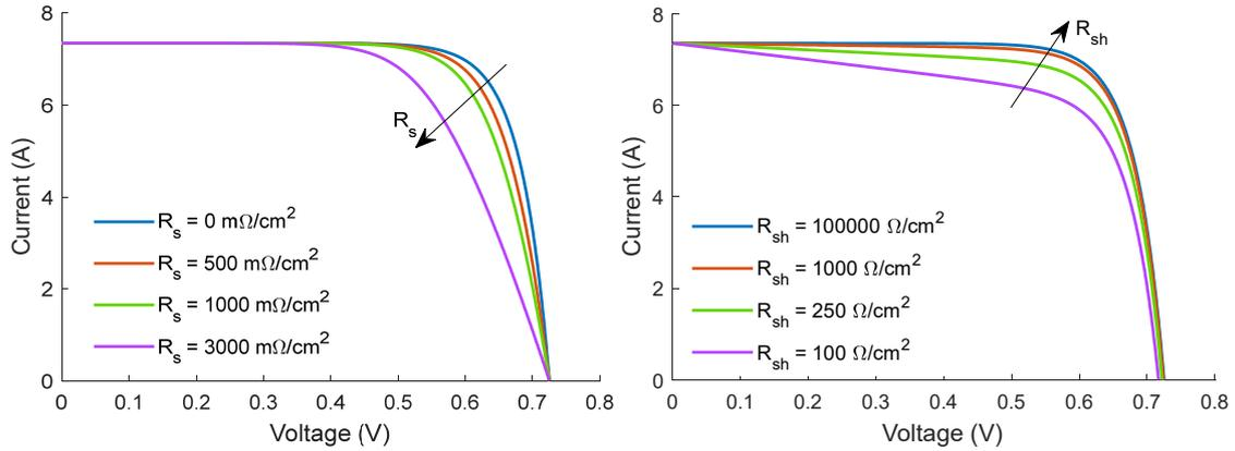
Figure 2.18: Dependence of the  $I$ - $V$  curve on the parallel and series resistances
