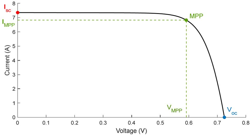
Figure 2.10: HIT cell  $I$ - $V$  curve
