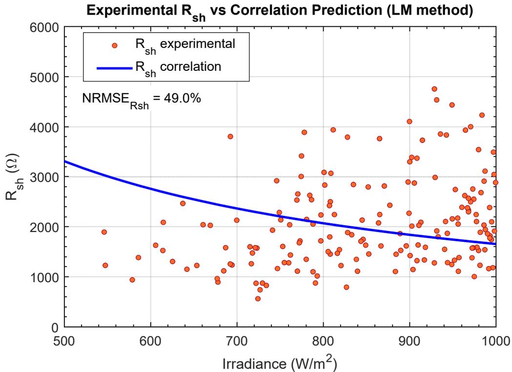
Figure 11.13:  $R_{sh}$  tendency with irradiance (LM algorithm)
