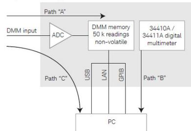
Direct I/O Measurements (Single reading – measure and I/O time)<sup>6</sup>
