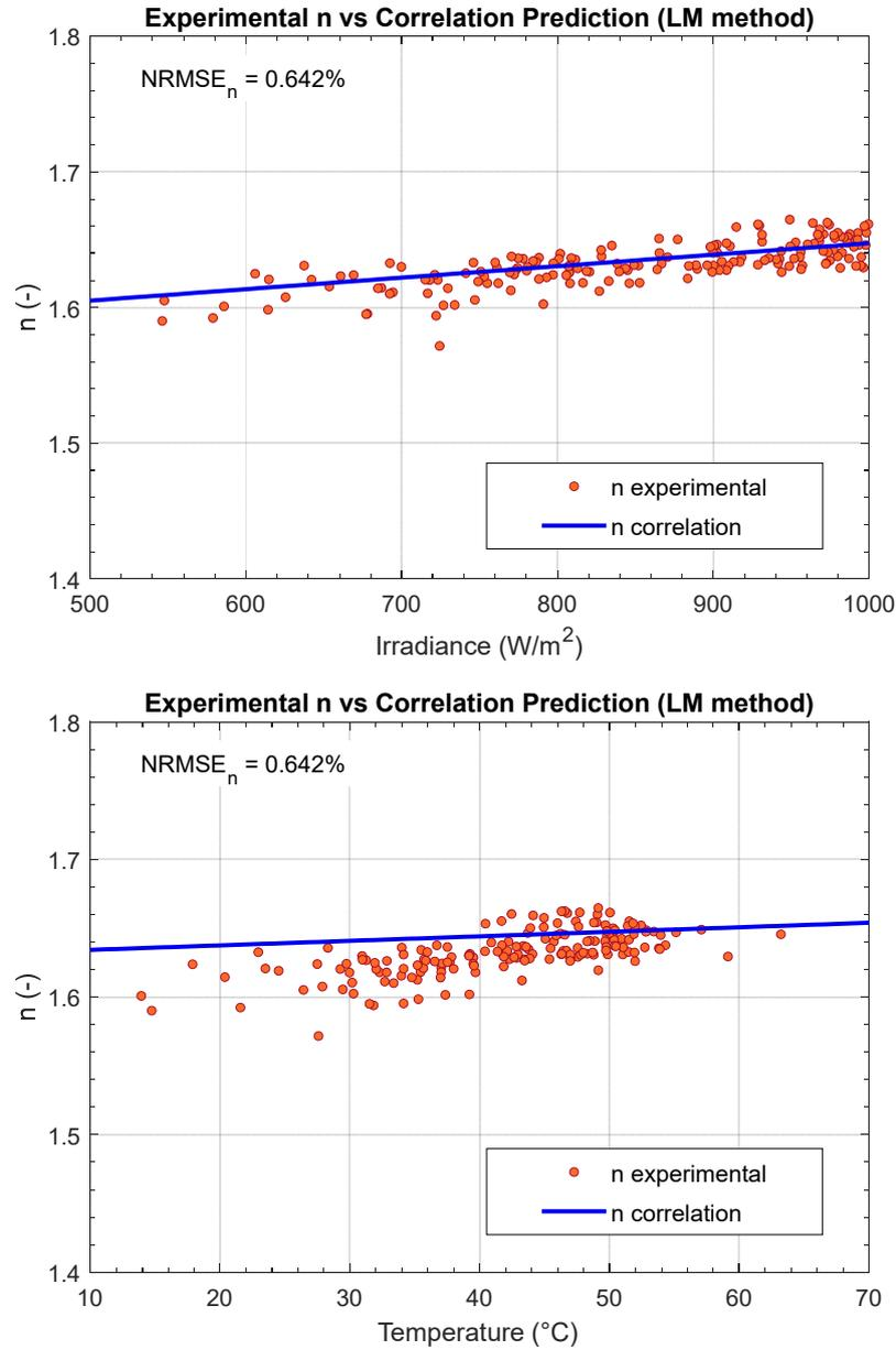
Figure 11.9:  $n$  tendency with irradiance and temperature (LM algorithm)
