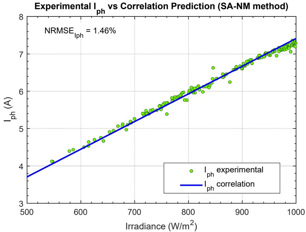
Figure 11.6:  $I_{ph}$  tendency with irradiance (SA-NM method)
