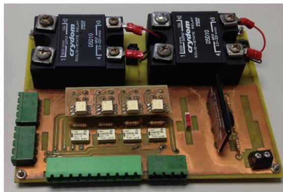
Figure 4.5: Picture of the multiplex board of each module
