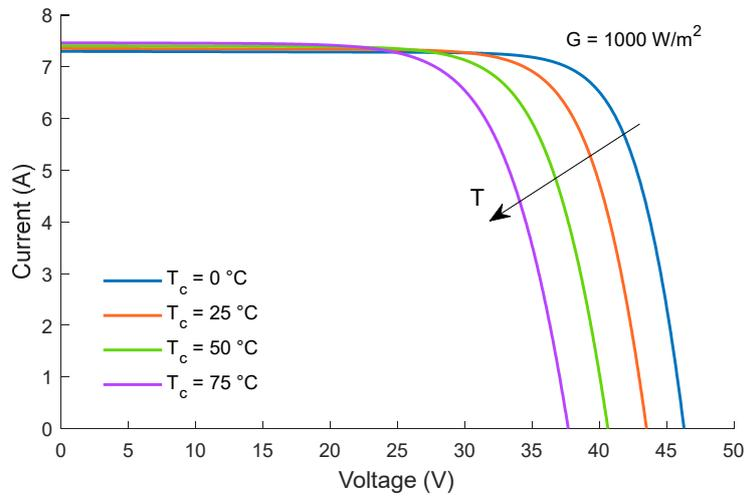
Figure 2.11: Dependence of the  $I$ - $V$  curve on temperature
