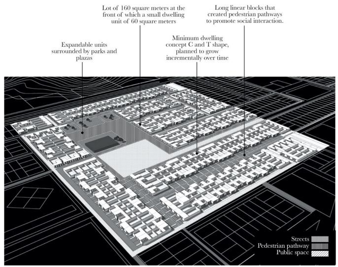
Figure 27. Digital reconstruction in axonometric view of housing cluster. Kahatt, Sh (2011). Urbanity as a project of modernization. Urban design and progressive housing strategies in Lima 1954-1984.
