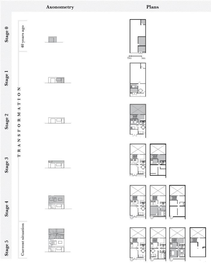
Figure 47. Different stages of development in a self-build house from Villa El Salvador. Rodriguez, C. (2015). The Transformation of Squatter Settlements into Urban Cities through the Effects of Tenure Security in Housing and Infrastructure Investments: The Evidence of Three Squatter Settlements in Lima, Peru, pp. 196.
