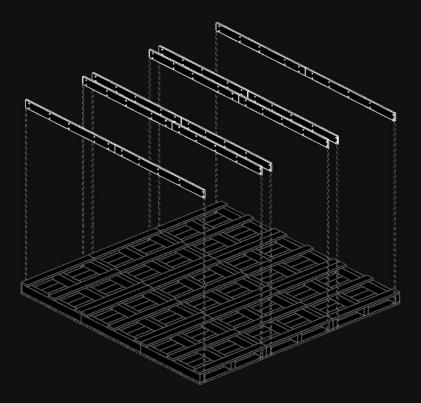
Two parallel walls need to be shorter in width in order to fit later with the other walls and not exceed the dimension of the floor
