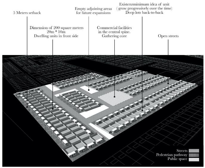
Figure 21. Digital reconstruction in axonometric view of housing cluster. Kahatt, Sh (2011). Urbanity as a project of modernization. Urban design and progressive housing strategies in Lima 1954-1984.
