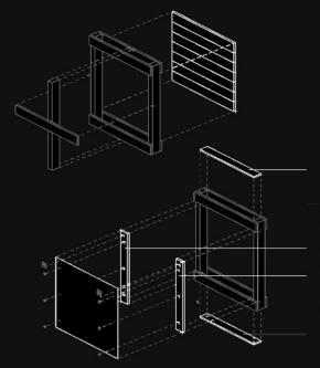
Disassembled parts will be used in order to fill the gaps and to build the frame of the polycarbonate panel. Holes will be drilled both on panel and on the frame in order to be secured later with washered wings nuts.
