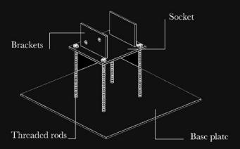
The steel socket which is holding the column is made out of three pieces of steel. The objective is to obtain a socket that correctly holds the column
