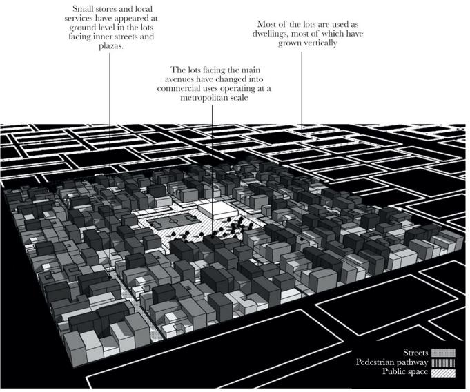
Figure 42. Reconstruction in axonometric view of housing cluster. Kahatt, Sh (2011). Urbanity as a project of modernization. Urban design and progressive housing strategies in Lima 1954-1984. *CLARA*, *No4*.
