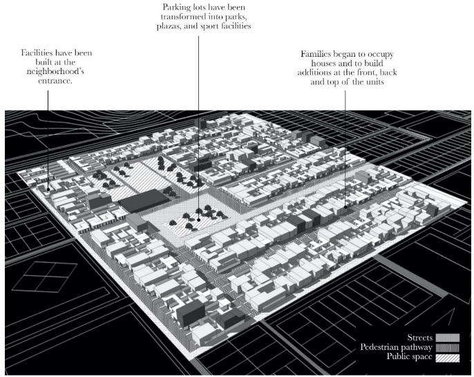
Figure 30. Digital reconstruction in axonometric view of housing cluster. Kahatt, Sh (2011). Urbanity as a project of modernization. Urban design and progressive housing strategies in Lima 1954-1984.
