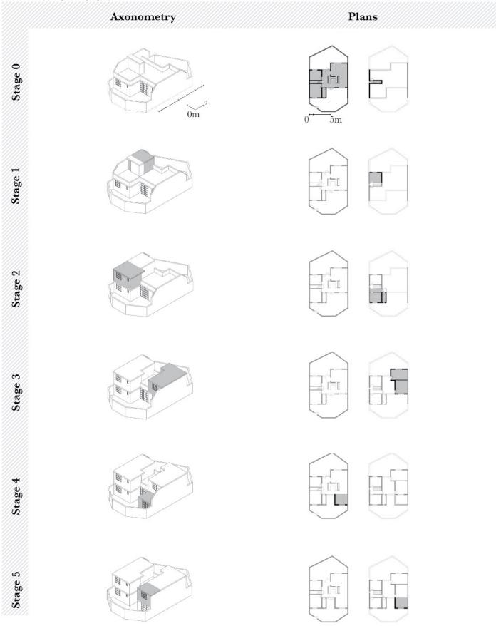
Figure 43. Different stages of development in Aldo Van Eyk project in PREVI. Source of axonometry and plans: Bas Hoevenaars 4243544, April 2014
