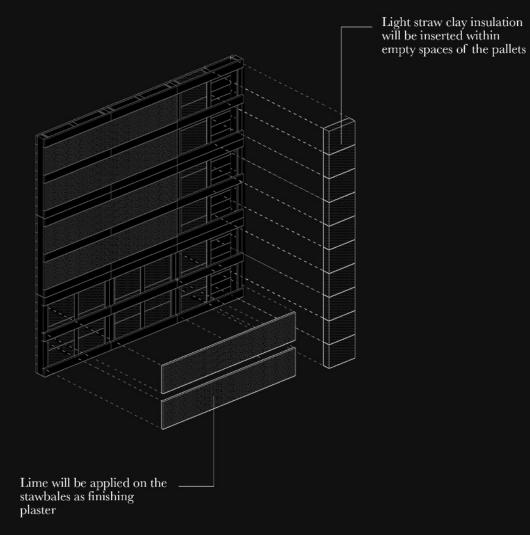
Figure 67. Insulating pallets
