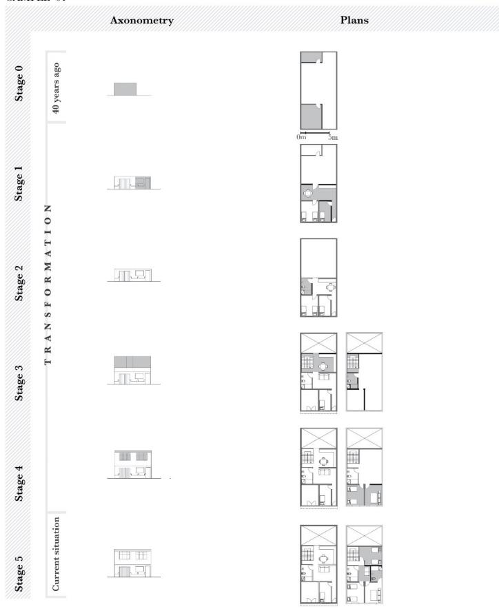
Figure 46. Different stages of development in a self-build house from Villa El Salvador. Rodriguez, C. (2015). The Transformation of Squatter Settlements into Urban Cities through the Effects of Tenure Security in Housing and Infrastructure Investments: The Evidence of Three Squatter Settlements in Lima, Peru, pp. 201.
