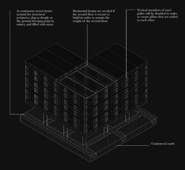
Figure 68. Rubble trench foundation
