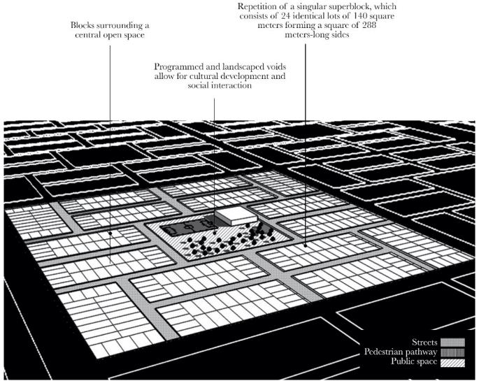
Figure 39. Reconstruction in axonometric view of housing cluster. Kahatt, Sh (2011). Urbanity as a project of modernization. Urban design and progressive housing strategies in Lima 1954-1984. *CLARA*, *No4*.
