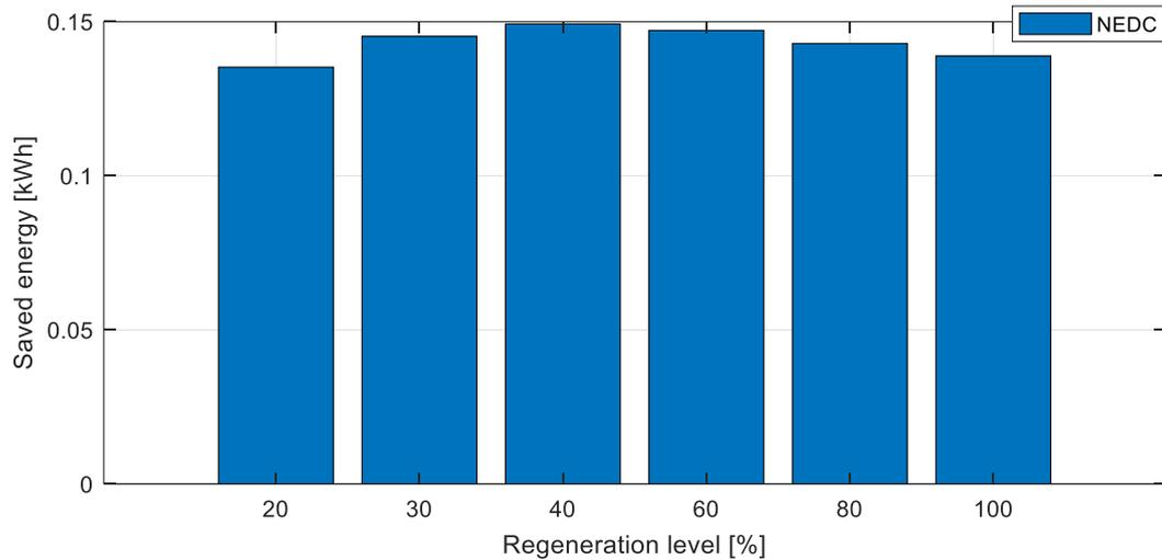
Figure 45. Saved energy with different reg. levels in NEDC
