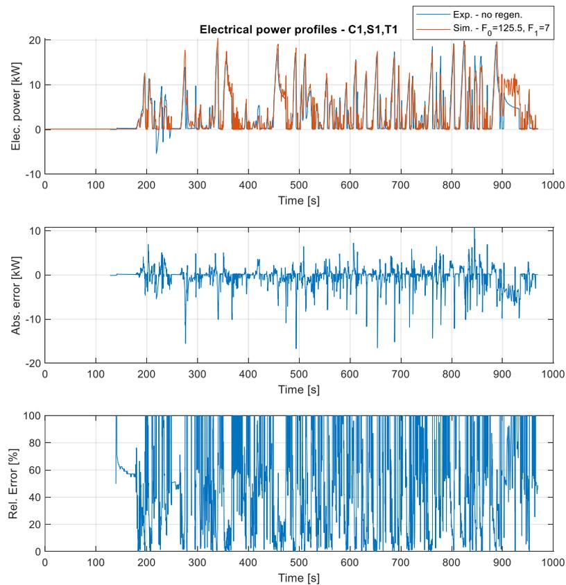
Figure 110. Electrical power profile and its error simulated with C1,S1,T1
