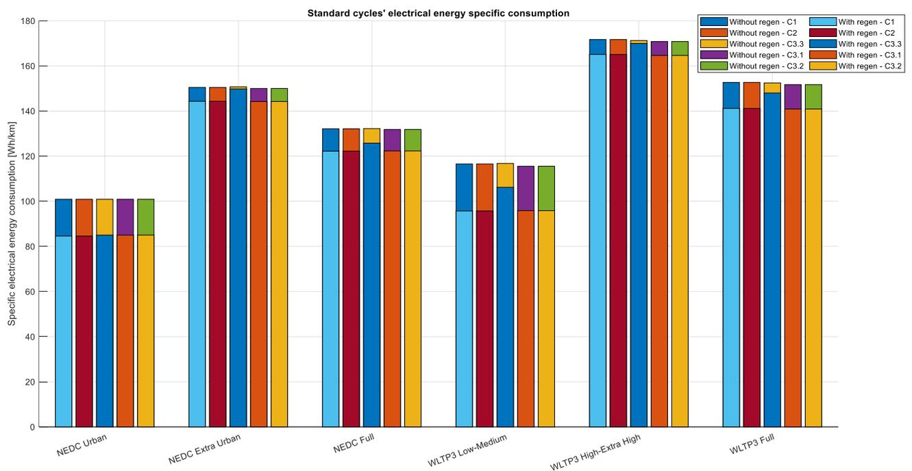
Figure 170. Specific energy consumption of C1, C2, C3.3, C3.1 and C3.2
