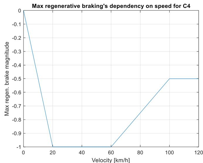
Figure 166. Maximum regenerative braking's dependency on vehicle velocity for C4 strategy
