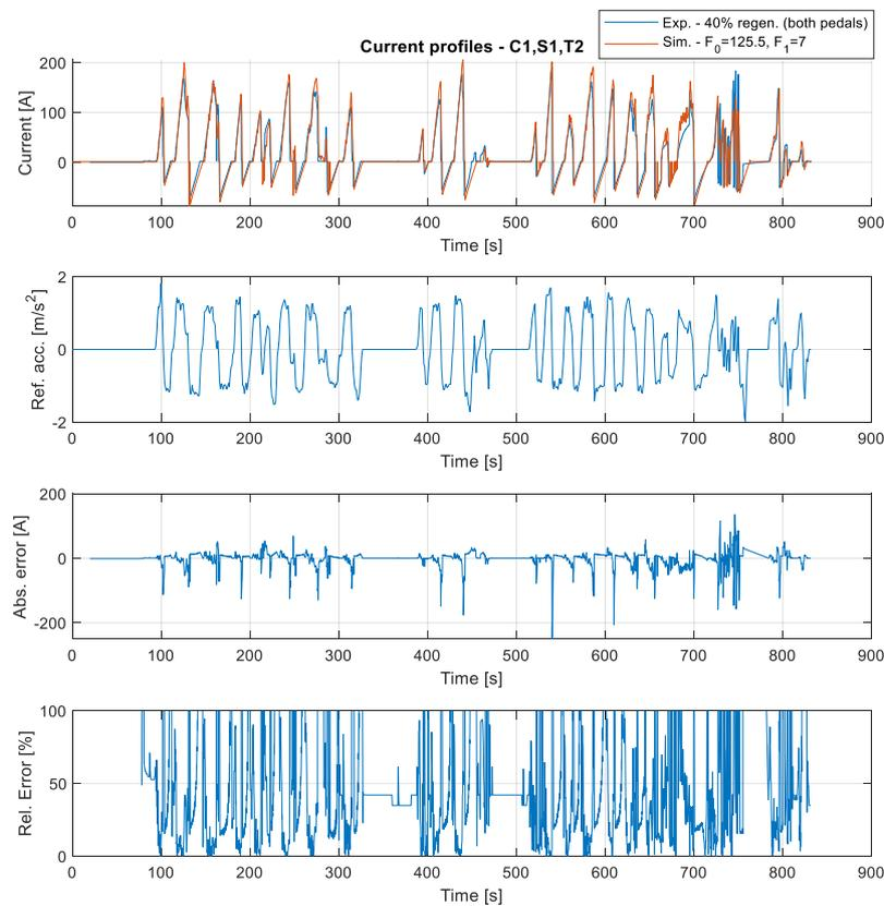
Figure 114. Current profile and its error simulated with C1,S1,T2
