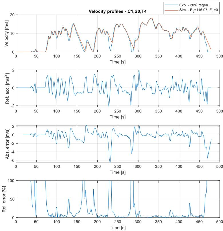
Figure 103. Velocity profile and its error simulated with C1,S0,T4
