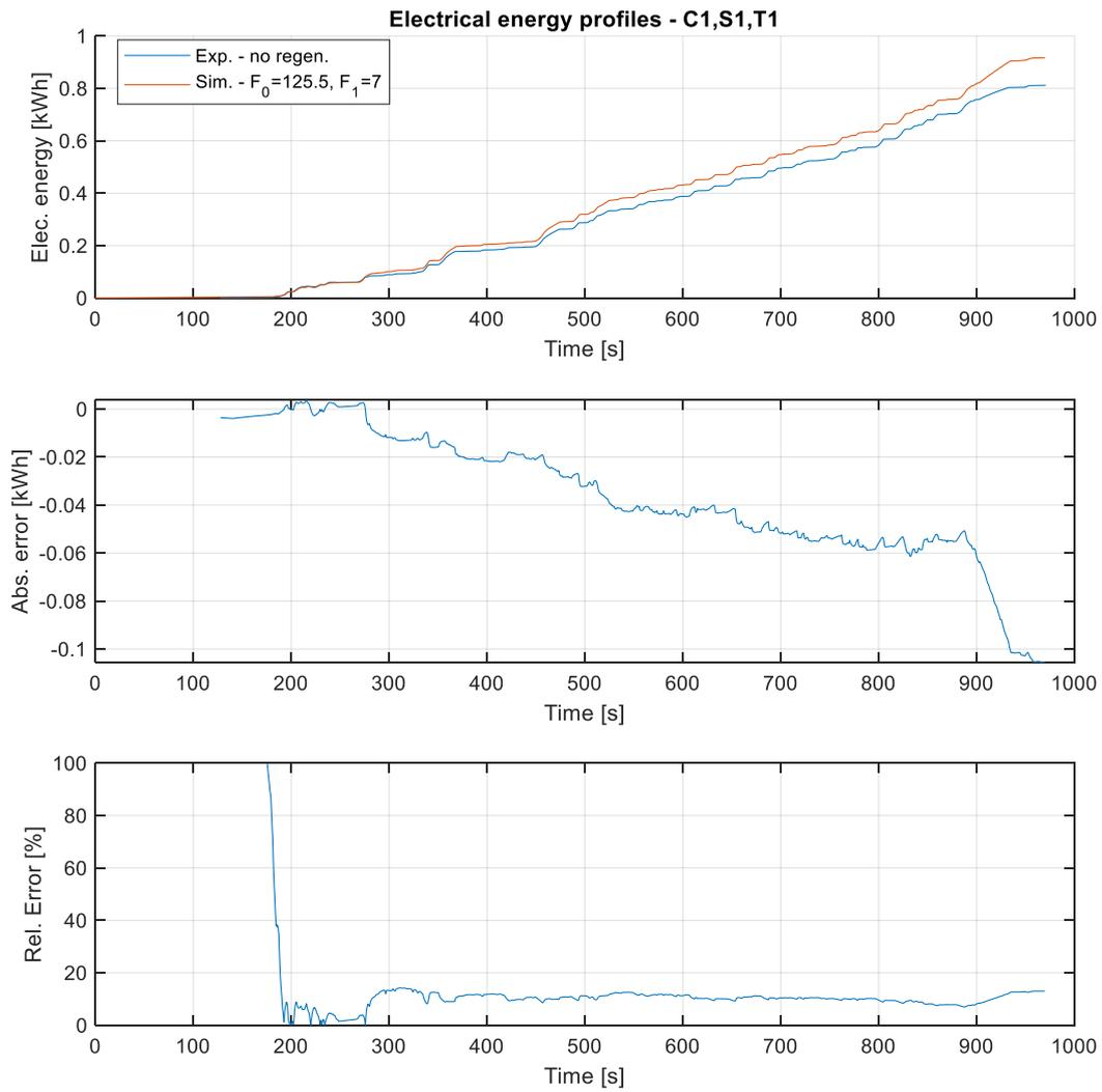
Figure 111. Electrical energy profile and its error simulated with C1,S1,T1
