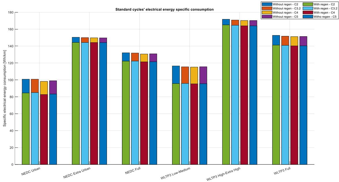
Figure 179. Specific electrical energy consumption of standard driving cycles with different one-pedal driving strategies
