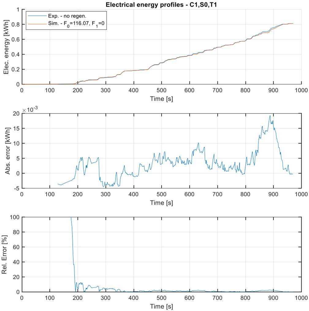
Figure 91. Electrical energy profile and its error simulated with C1,S0,T1
