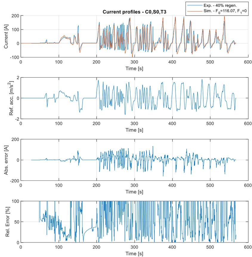
Figure 79. Current profile and its error simulated with C0,S0,T3
