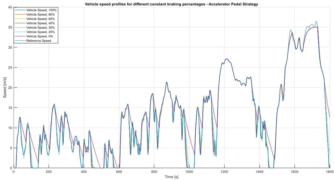
Figure 41. All the velocity profiles simulated with accelerator pedal strategy – WLTP Class 3 cycle
