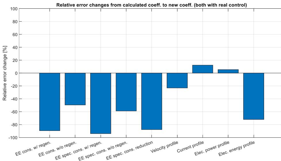
Figure 145. Relative error changes moving from calculated coast-down coeff. to the tuned ones with real control model
