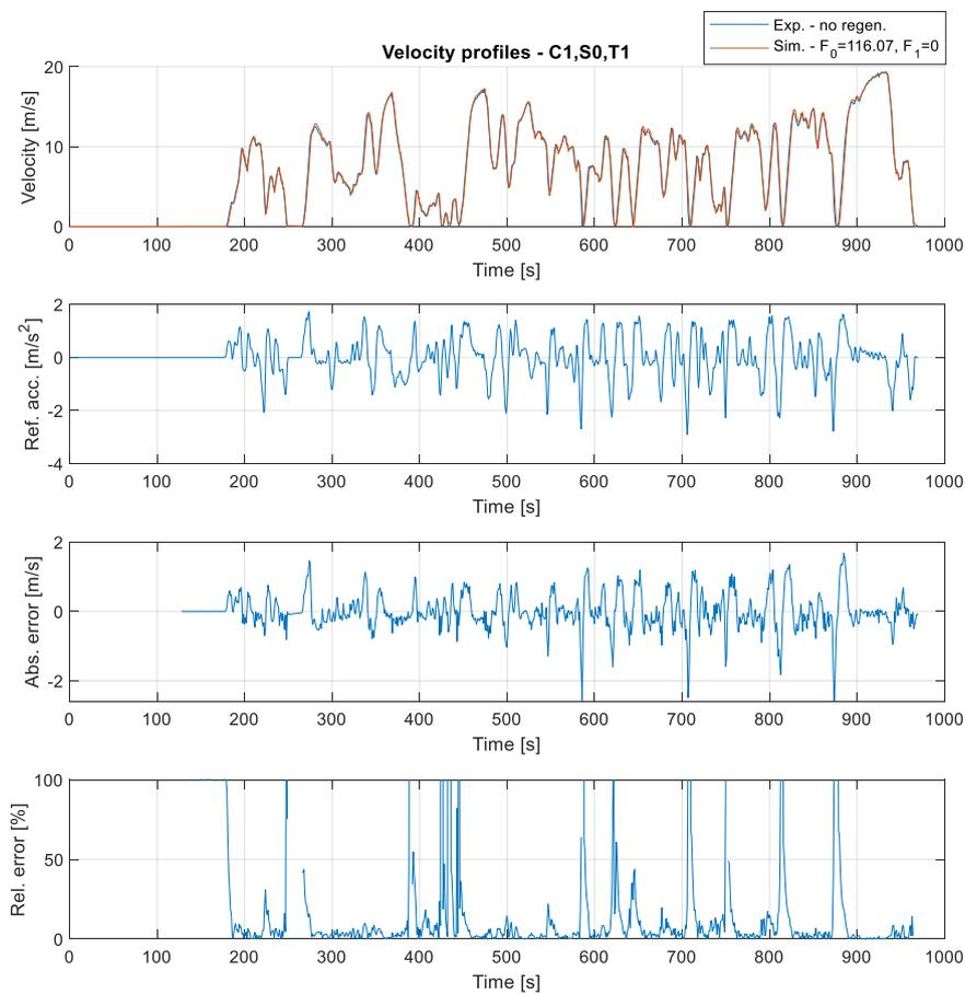
Figure 88. Velocity profile and its error simulated with C1,S0,T1
