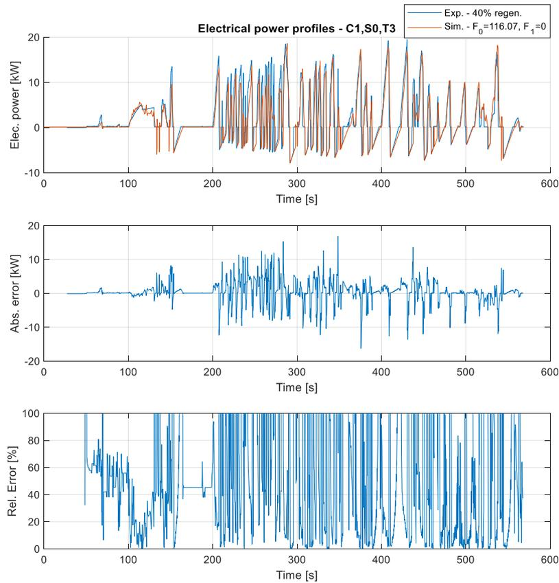
Figure 100. Electrical power profile and its error simulated with C1,S0,T3
