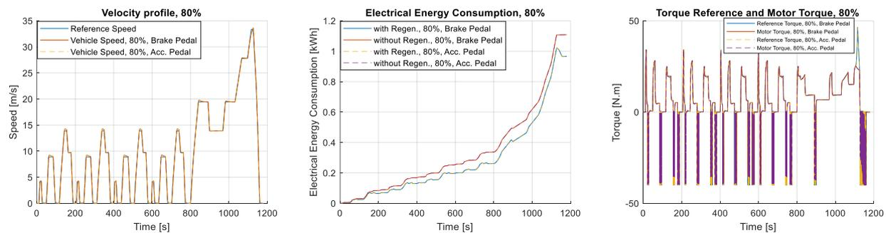
Figure 19. 80% on/off regenerative braking with both pedal strategy - NEDC cycle
