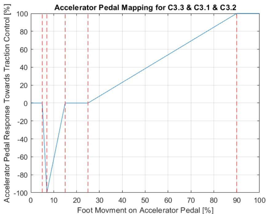
Figure 160. REDS accelerator pedal mapping used in C3.3, C3.1 and C3.2
