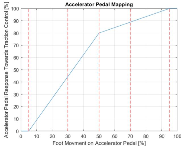
Figure 63. Accelerator pedal mapping of the vehicle during the experimental tests
