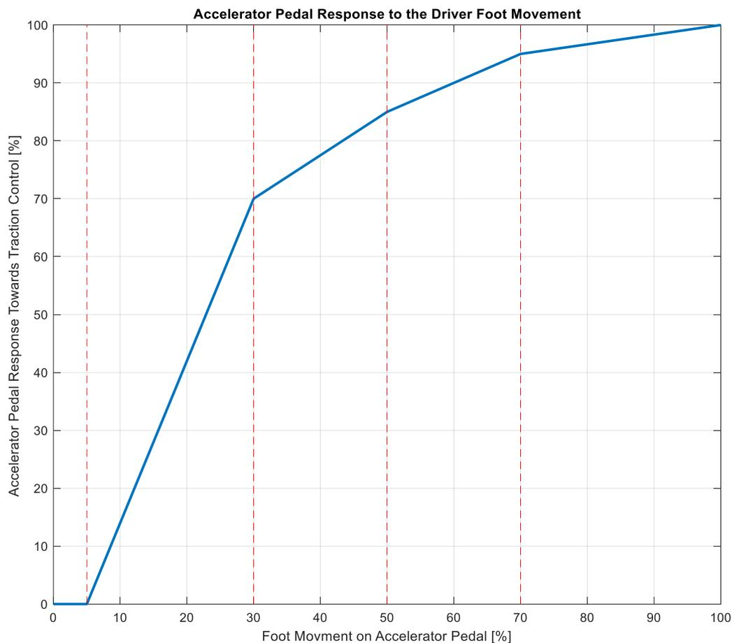
Figure 9. A simple sportive accelerator pedal mapping for an electric vehicle
