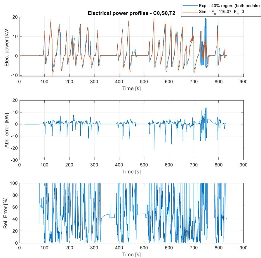
Figure 75. Electrical power profile and its error simulated with C0,S0,T2
