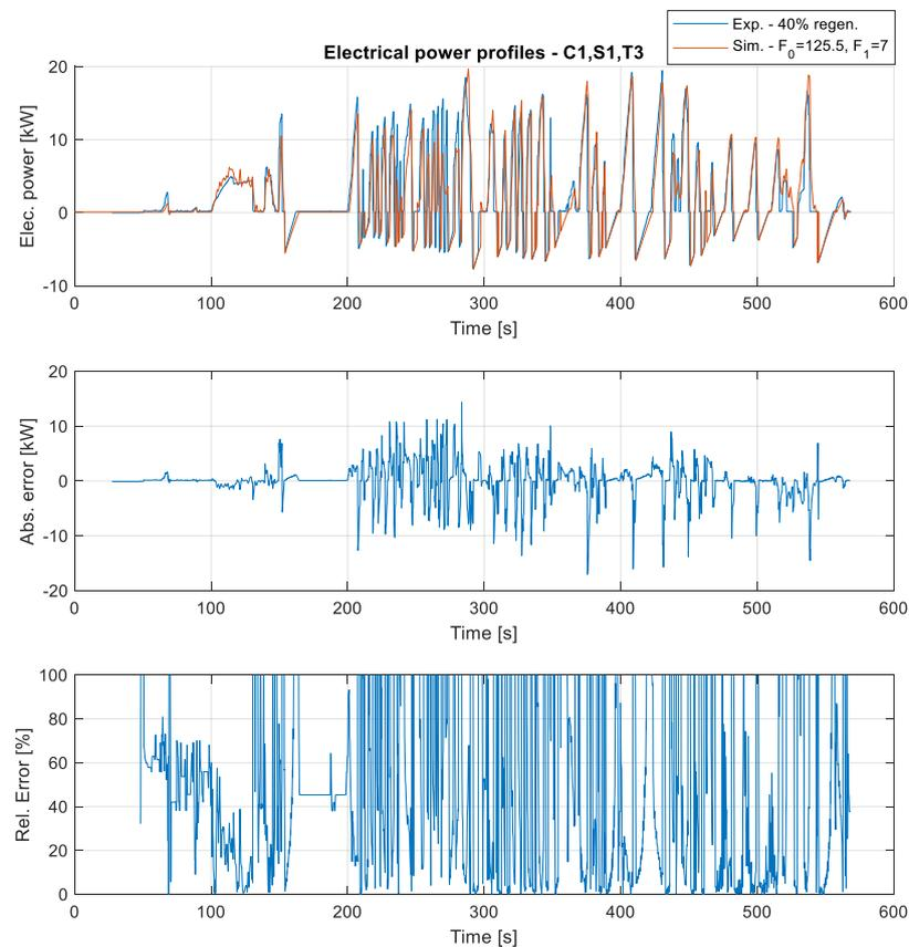
Figure 120. Electrical power profile and its error simulated with C1,S1,T3
