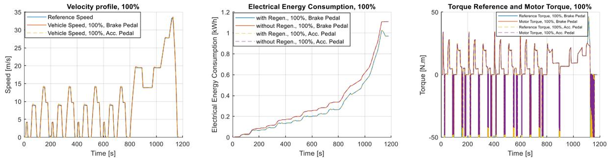
Figure 18. 100% on/off regenerative braking with both pedal strategy - NEDC cycle
