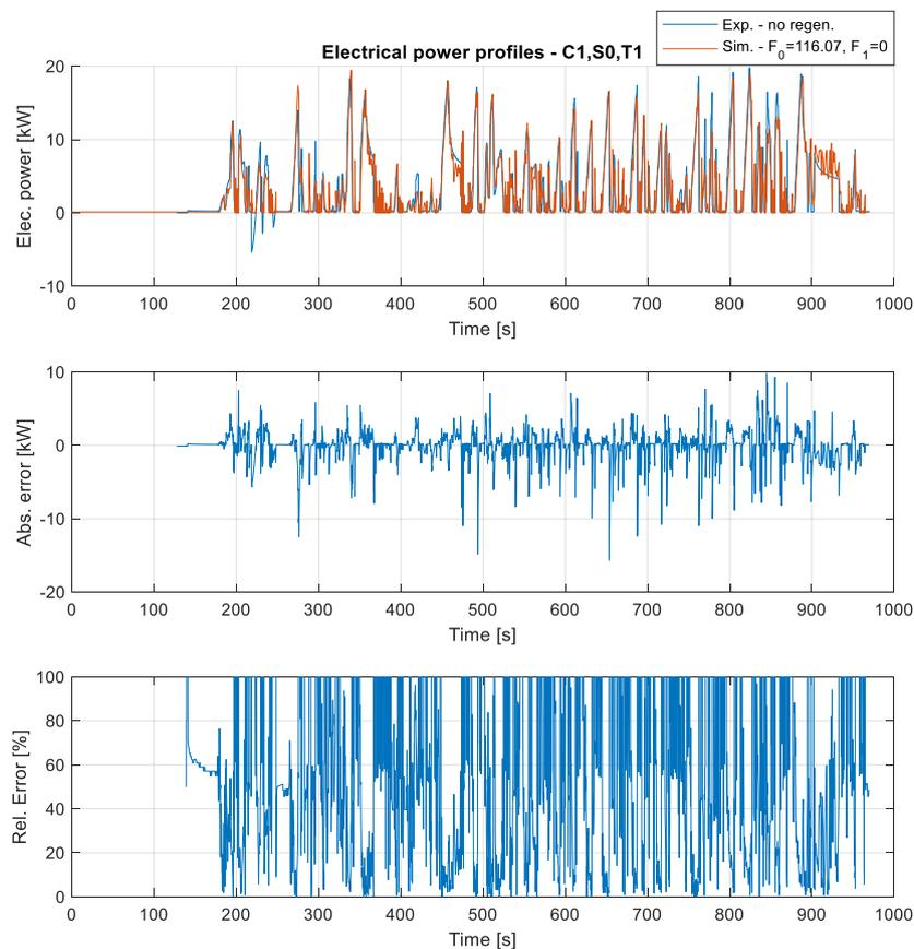
Figure 90. Electrical power profile and its error simulated with C1,S0,T1
