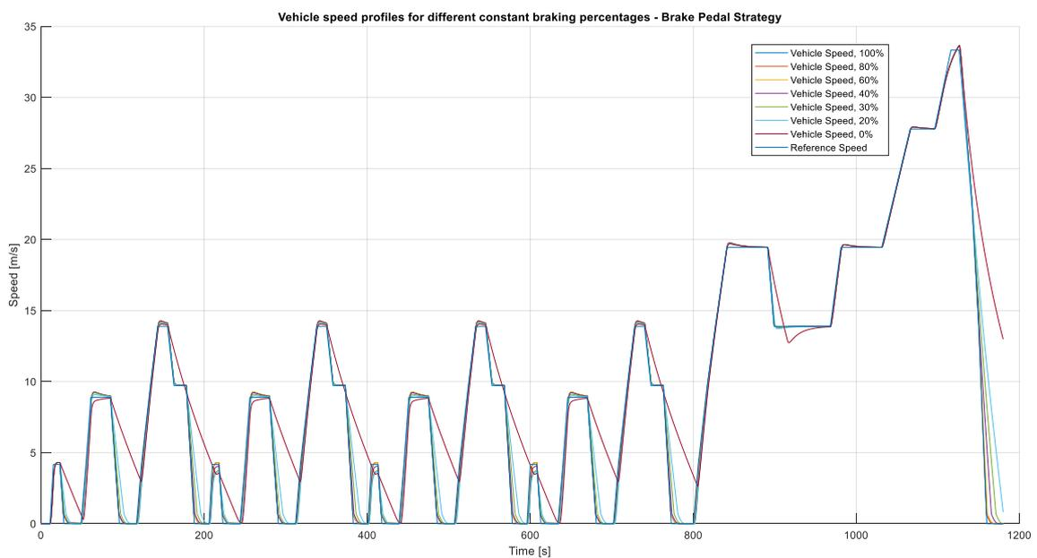
Figure 25. All the velocity profiles simulated with brake pedal strategy - NEDC cycle
