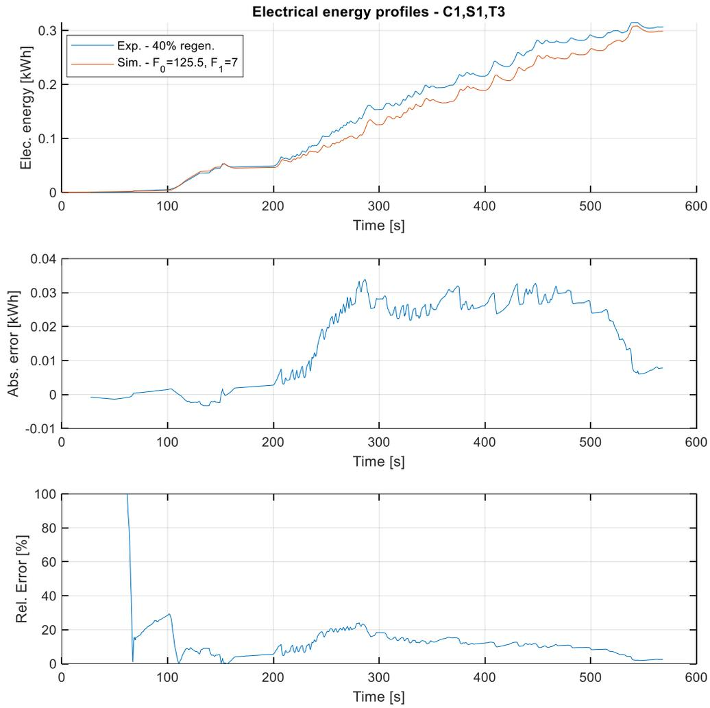
Figure 121. Electrical energy profile and its error simulated with C1,S1,T3
