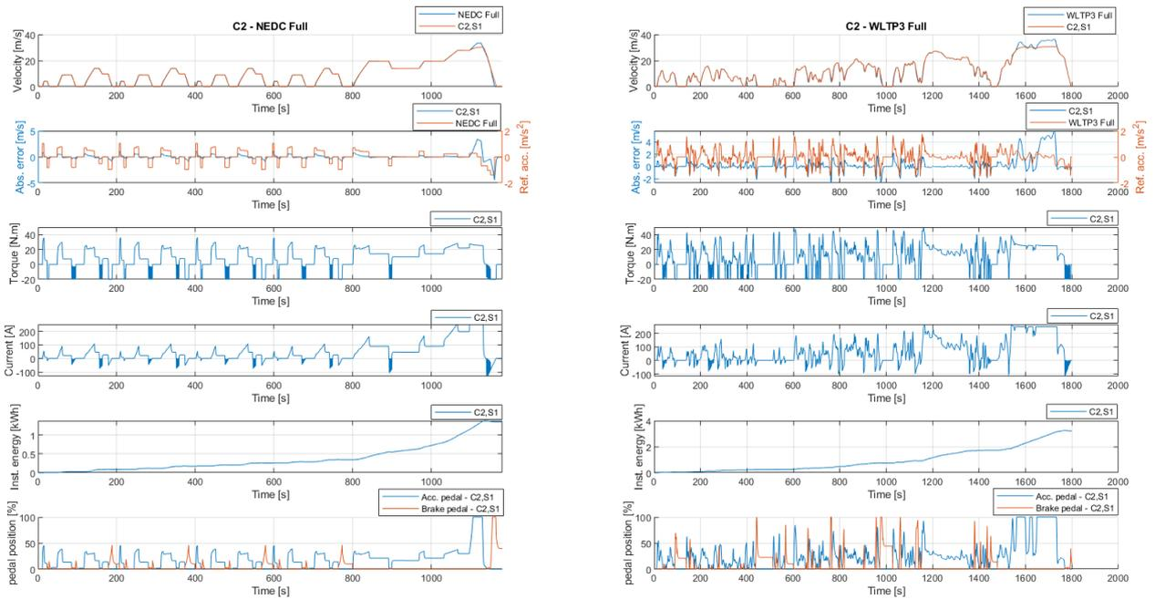
Figure 198. C2 simulation results for NEDC and WLTP Class 3 cycles
