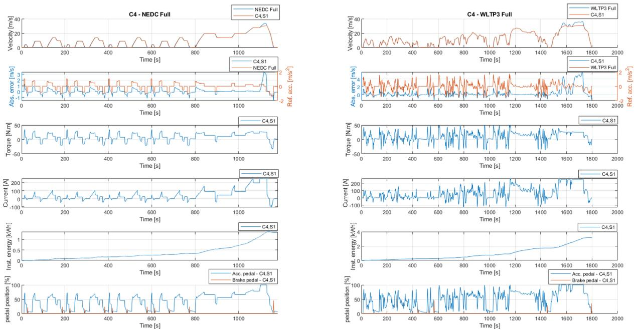
Figure 200. C4 simulation results for NEDC and WLTP Class 3 cycles
