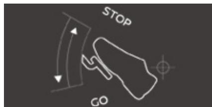
Figure 1. Accelerator pedal functioning of Nissan e-Pedal [1]
