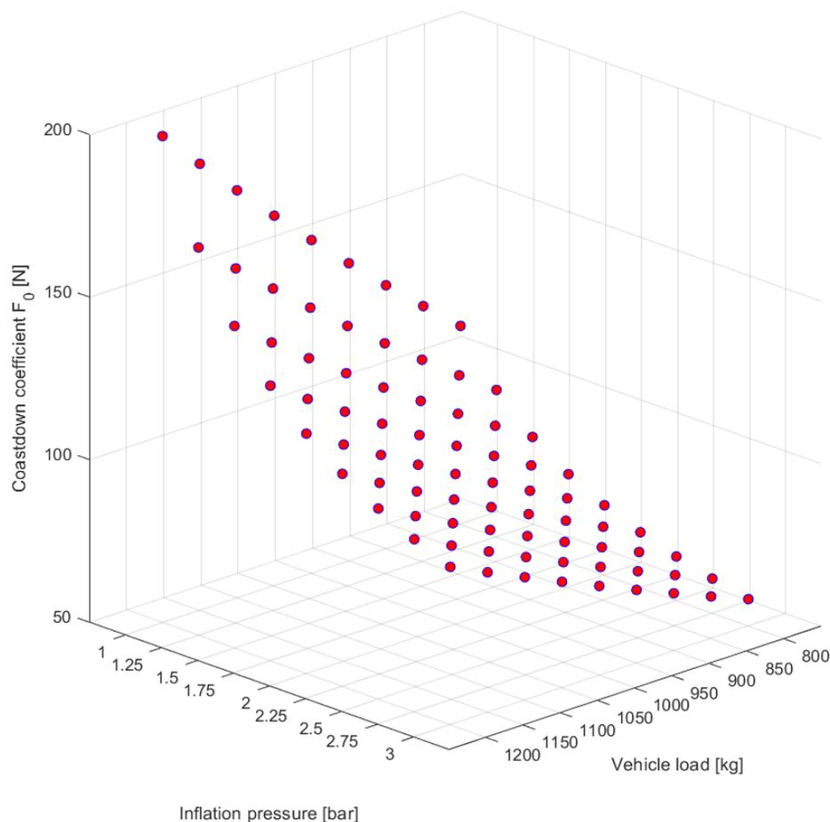
Figure 49.  $F_0$  for different combinations of vehicle load and inflation pressure
