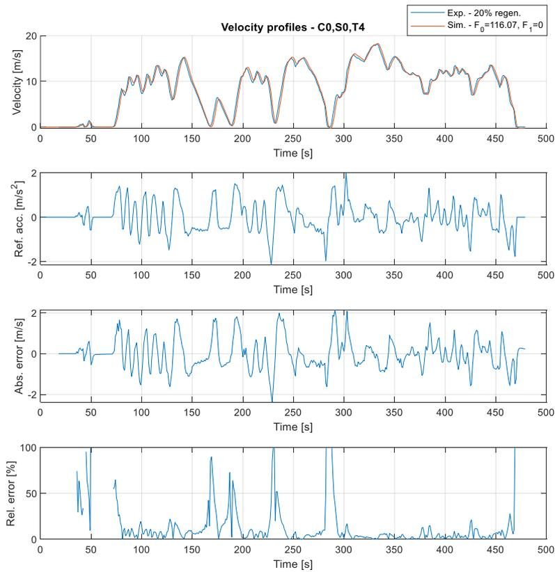
Figure 83. Velocity profile and its error simulated with C0,S0,T4
