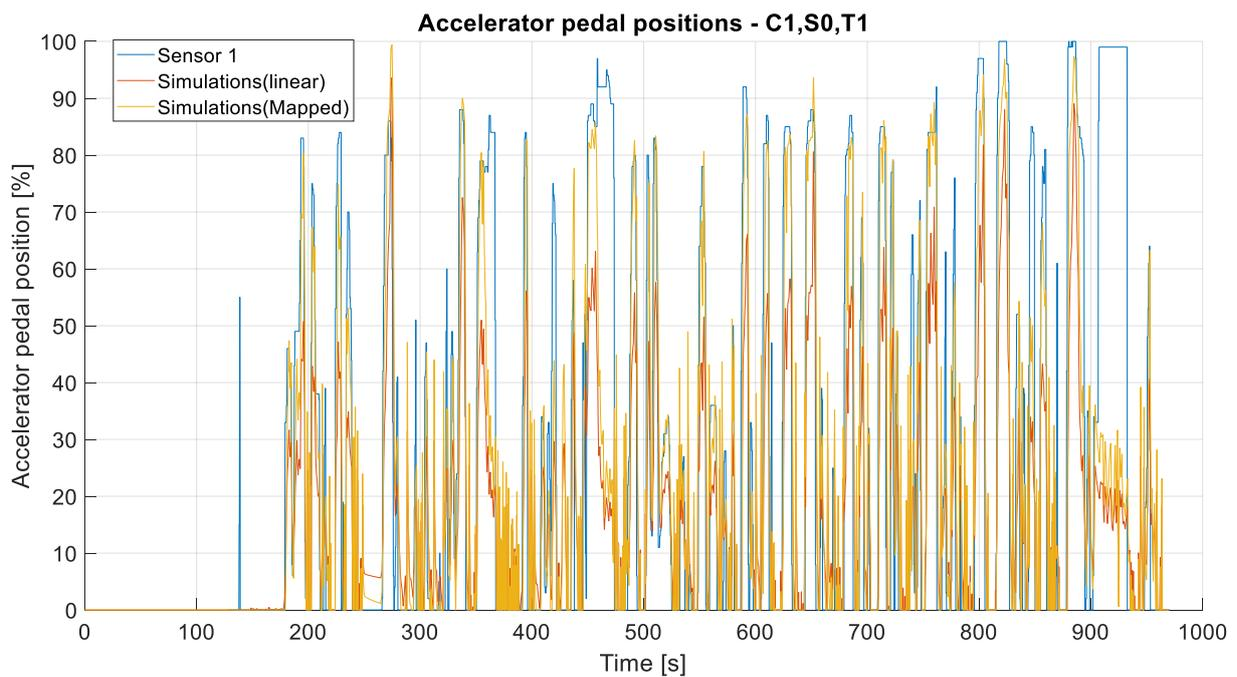
Figure 92. Accelerator pedal positions simulated with C1,S0,T1
