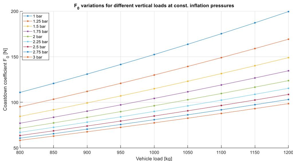
Figure 52.  $F_0$  variations for different vertical loads at constant inflation pressures
