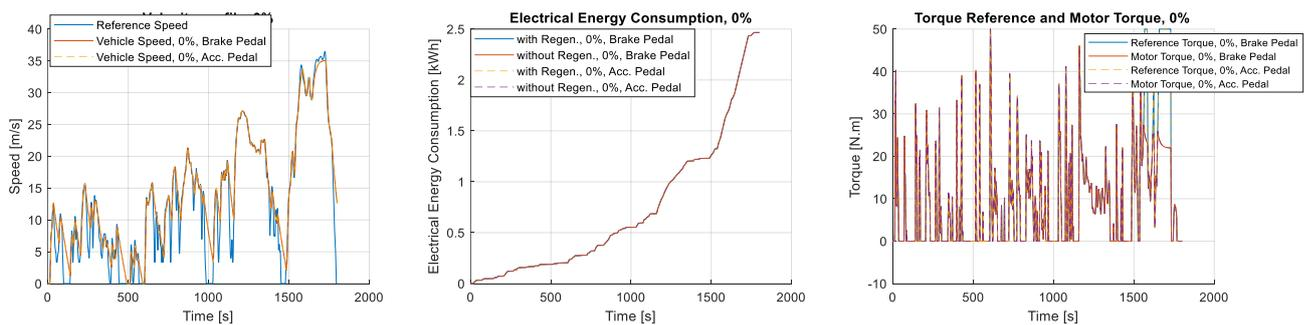
Figure 37. 0% on/off regenerative braking with both pedal strategy – WLTP Class 3 cycle
