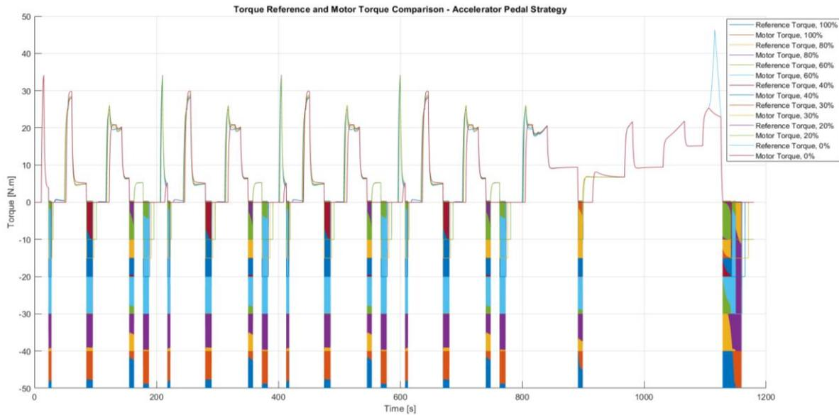
Figure 29. All the torque profiles simulated with accelerator pedal strategy – NEDC cycle
