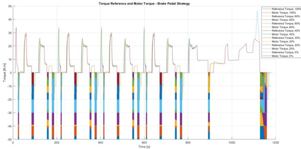
Figure 26. All the torque profiles simulated with brake pedal strategy – NEDC cycle
