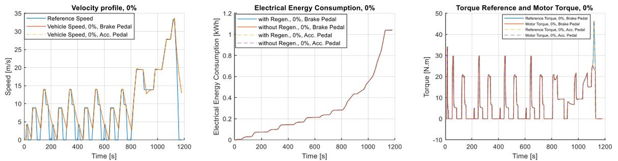
Figure 24. 0% on/off regenerative braking with both pedal strategy - NEDC cycle
