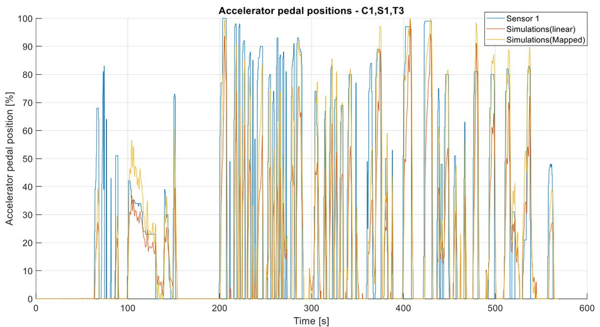
Figure 122. Accelerator pedal positions simulated with C1,S1,T3
