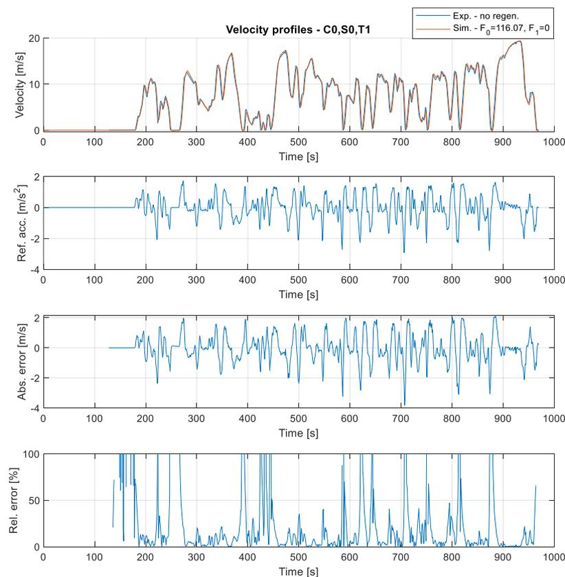
Figure 68. Velocity profile and its error simulated with C0,S0,T1
