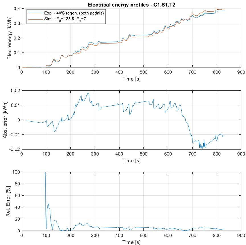
Figure 116. Electrical energy profile and its error simulated with C1,S1,T2
