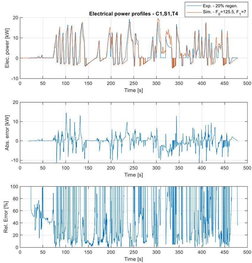
Figure 125. Electrical power profile and its error simulated with C1,S1,T4
