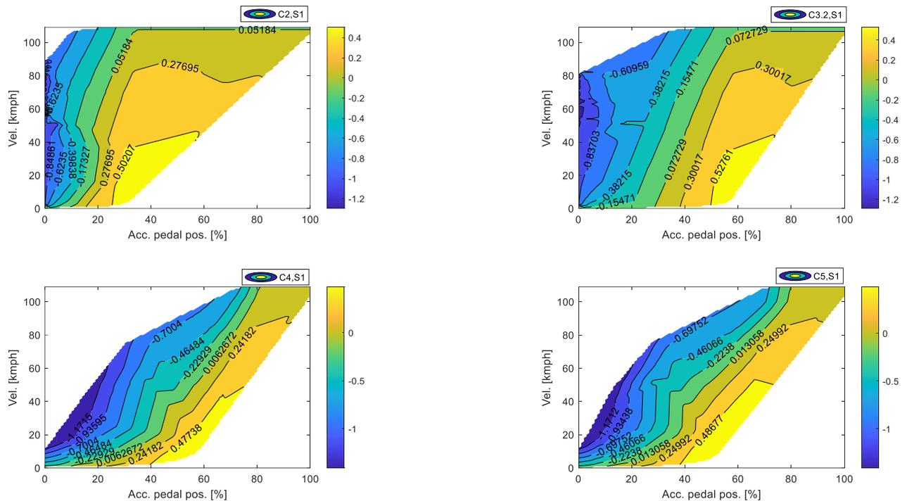
Figure 185. Acceleration contour plots – NEDC Extra Urban cycle
