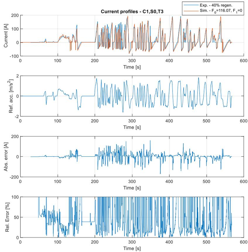
Figure 99. Current profile and its error simulated with C1,S0,T3
