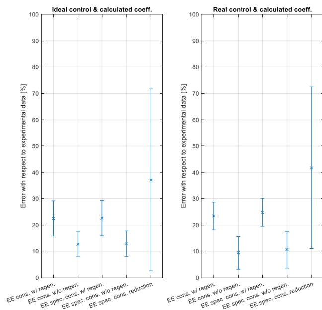
Figure 133. Average and corresponding standard deviation of consumption errors – C0,S0 vs. C1,S0
