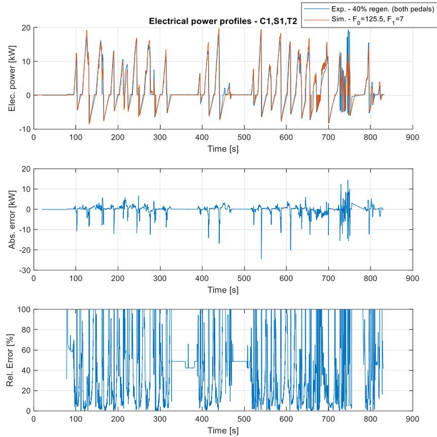
Figure 115. Electrical power profile and its error simulated with C1,S1,T2
