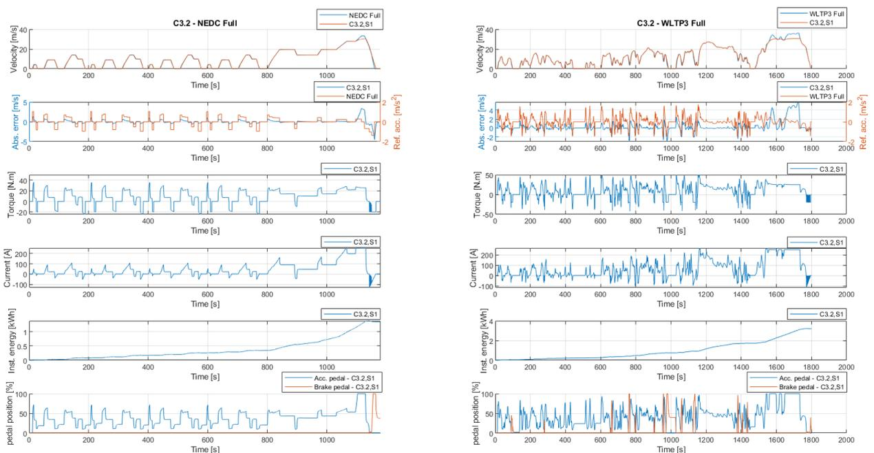
Figure 199. C3.2 simulation results for NEDC and WLTP Class 3 cycles
