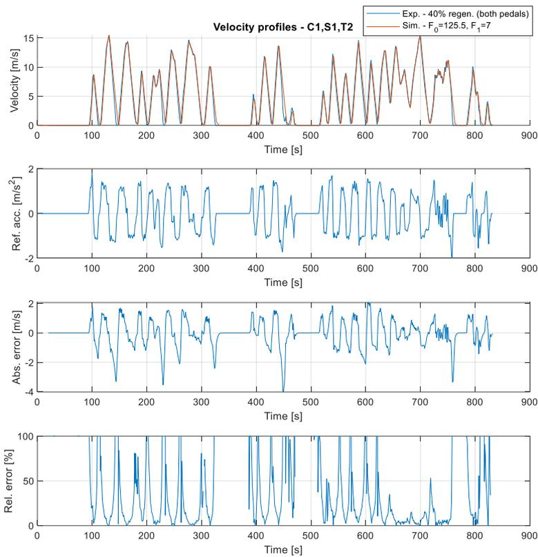
Figure 113. Velocity profile and its error simulated with C1,S1,T2
