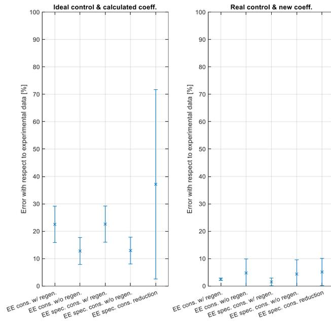
Figure 149. Average and corresponding standard deviation of consumption errors – C0,S0 vs. C1,S1
