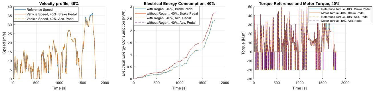
Figure 34. 40% on/off regenerative braking with both pedal strategy – WLTP Class 3 cycle
