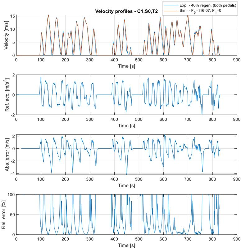
Figure 93. Velocity profile and its error simulated with C1,S0,T2
