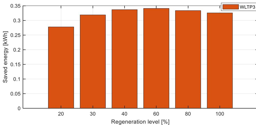
Figure 46. Saved energy with different reg. levels in WLTP Class 3
