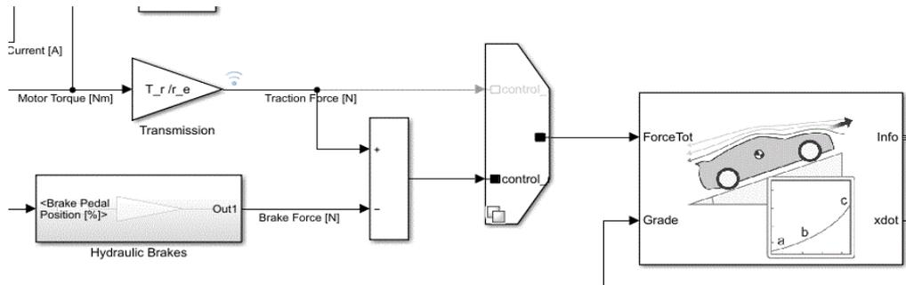
Figure 158. Implementation of hydraulic braking in the Simulink model
