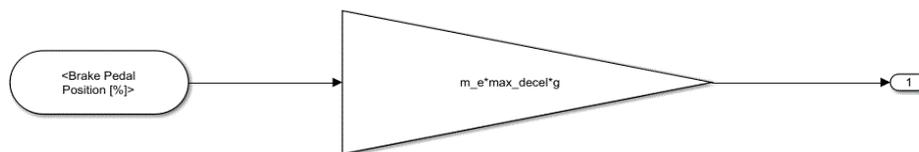
Figure 159. Linear relation between brake pedal position and maximum hydraulic braking force for the considered maximum deceleration value
