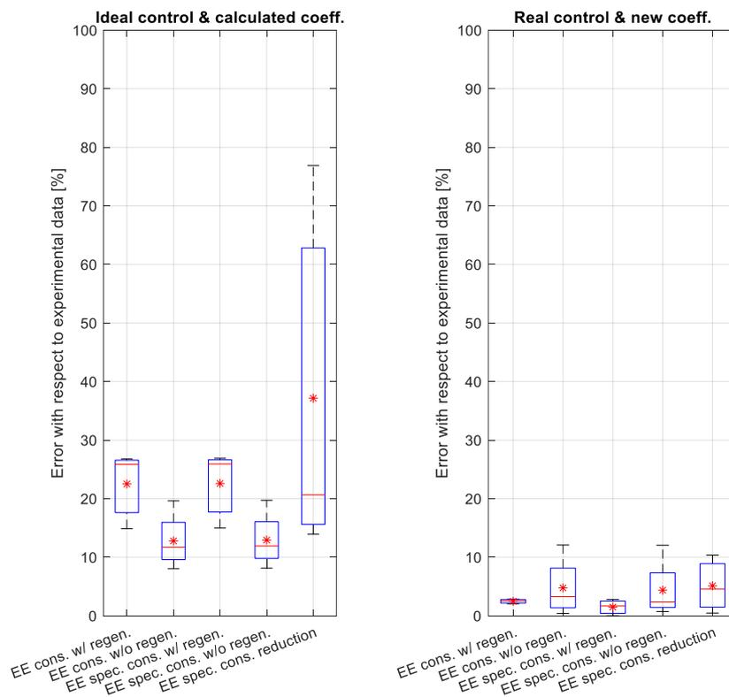
Figure 148. Distribution of consumption errors reported in box plots – C0,S0 vs. C1,S1
