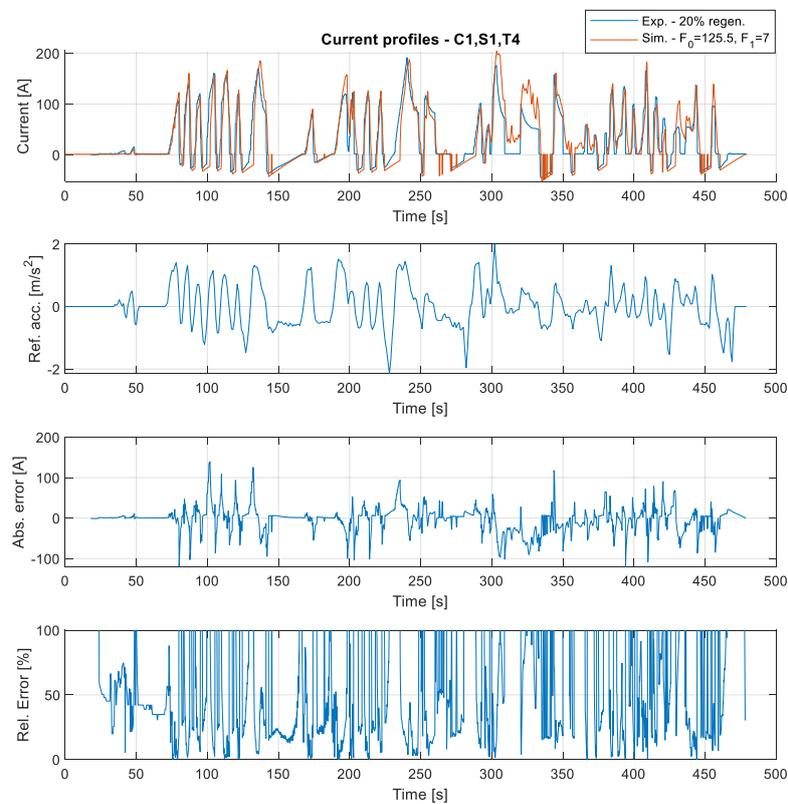
Figure 124. Current profile and its error simulated with C1,S1,T4
