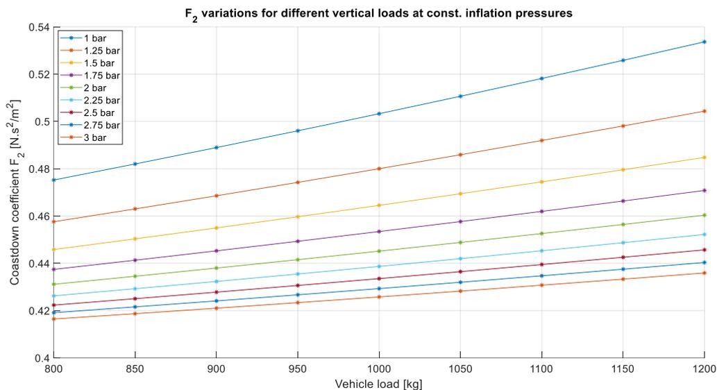
Figure 54.  $F_2$  variations for different vertical loads at constant inflation pressures
