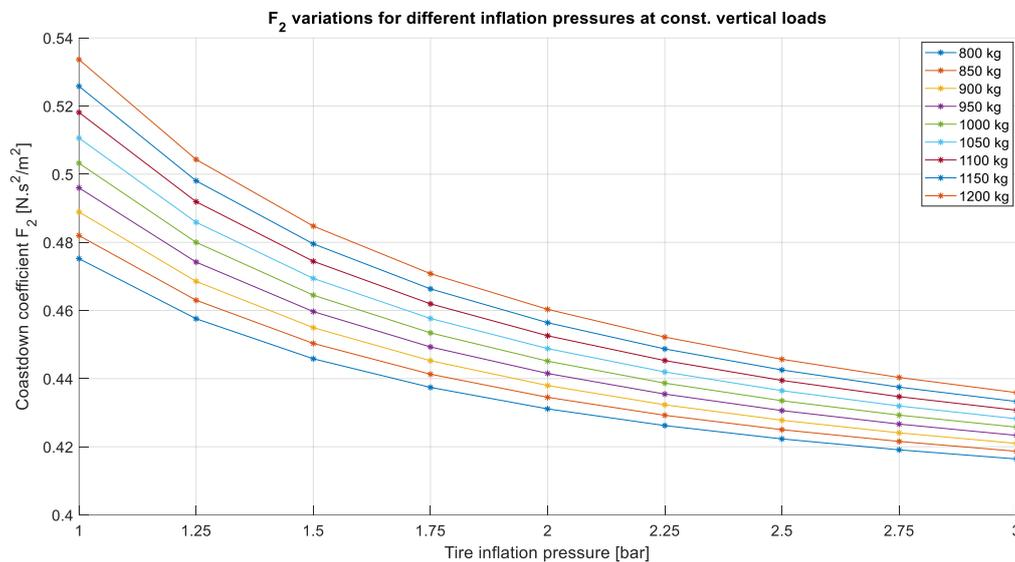
Figure 53.  $F_2$  variations for different inflation pressures at constant vertical loads
