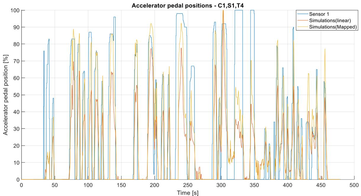
Figure 127. Accelerator pedal positions simulated with C1,S1,T4
