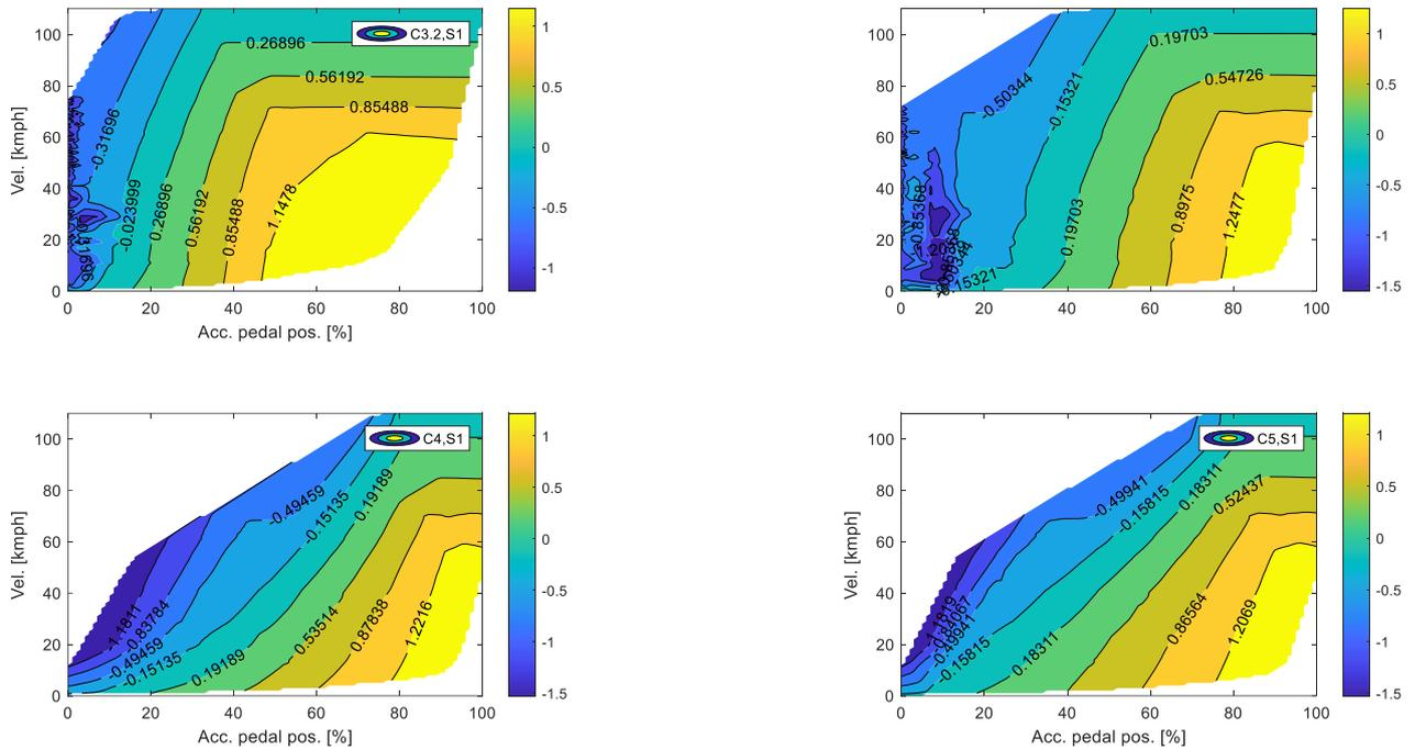
Figure 194. Acceleration contour plots – WLTP Class 3 High-Extra High
