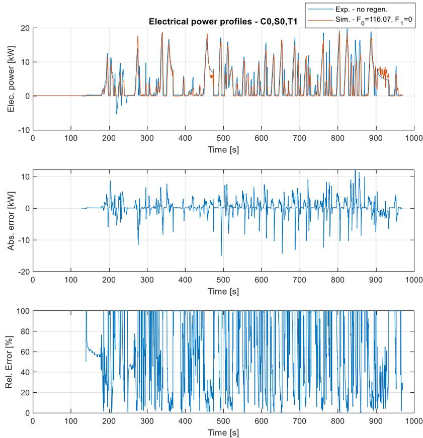
Figure 70. Electrical power profile and its error simulated with C0,S0,T1
