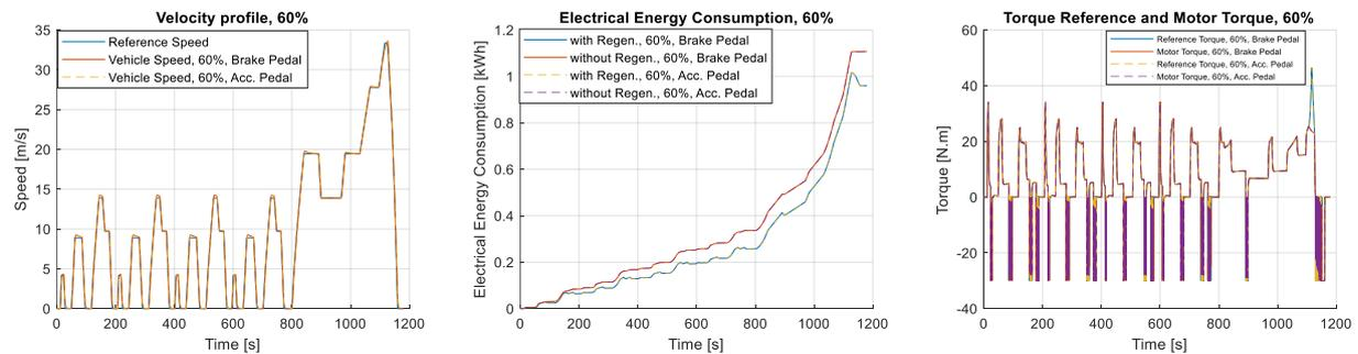
Figure 20. 60% on/off regenerative braking with both pedal strategy - NEDC cycle
