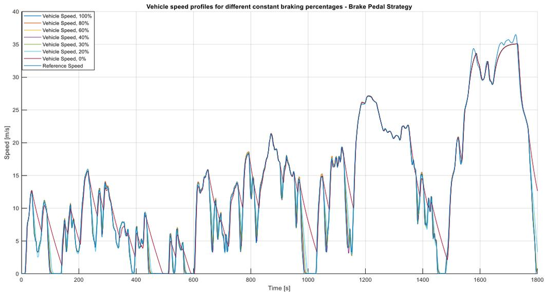
Figure 38. All the velocity profiles simulated with brake pedal strategy – WLTP Class 3 cycle
