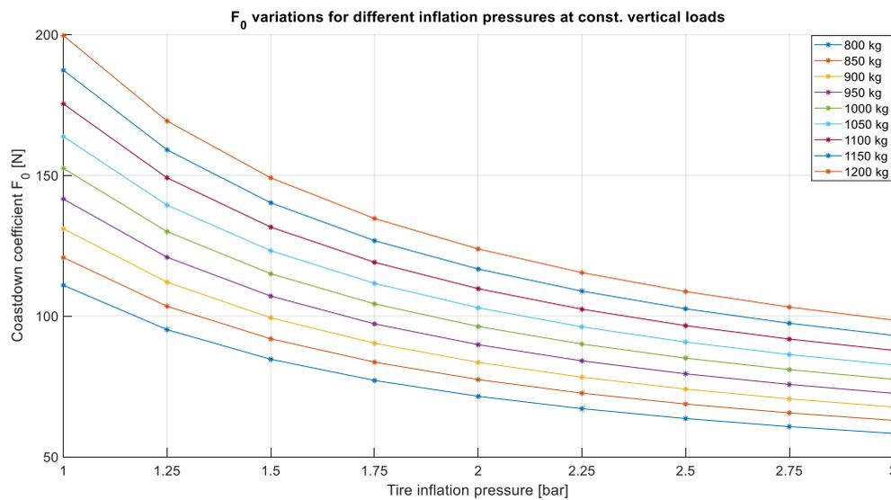
Figure 51.  $F_0$  variations for different inflation pressures at constant vertical loads
