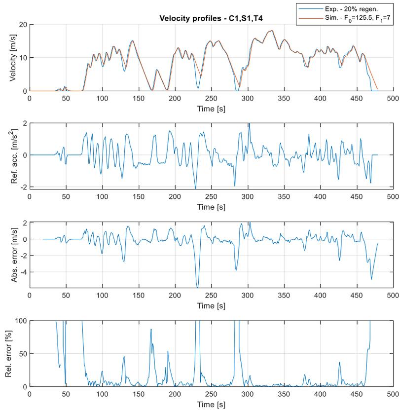
Figure 123. Velocity profile and its error simulated with C1,S1,T4
