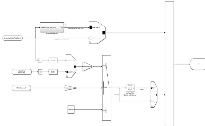
Figure 154. Simulink implementation of C1
