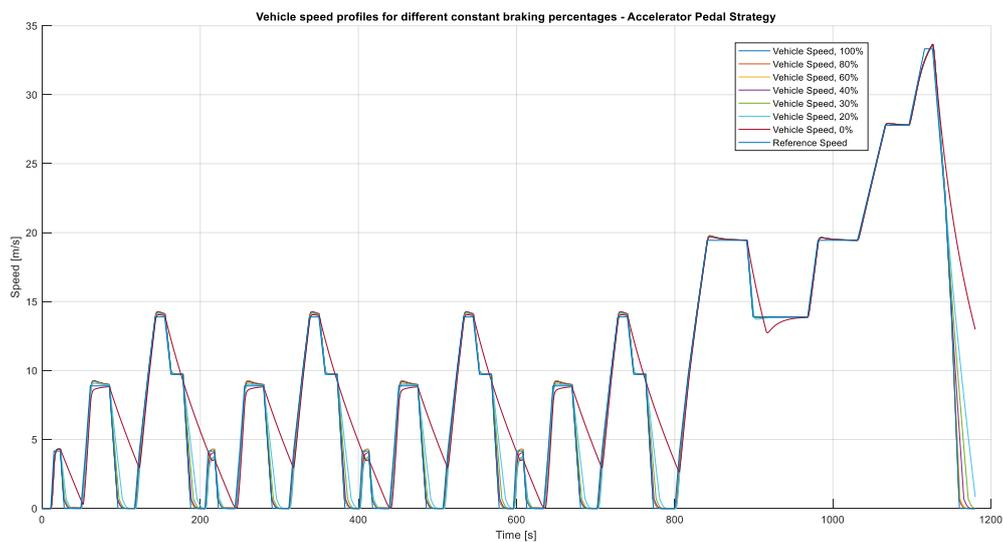
Figure 28. All the velocity profiles simulated with accelerator pedal strategy - NEDC cycle
