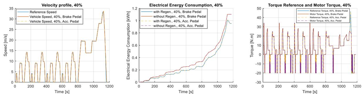
Figure 21. 40% on/off regenerative braking with both pedal strategy - NEDC cycle
