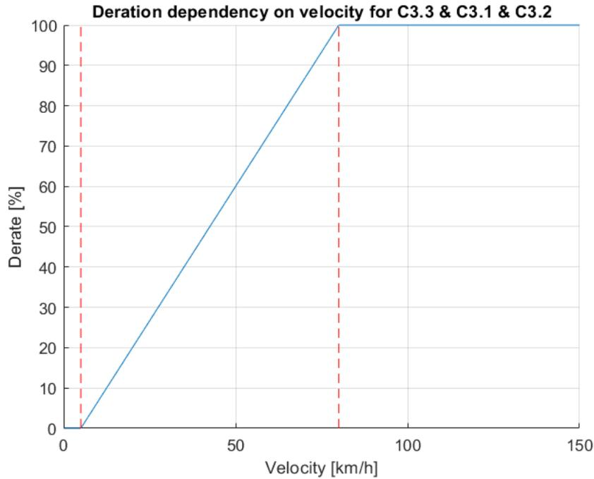
Figure 161. Degradation of maximum regenerative braking in REDS strategy
