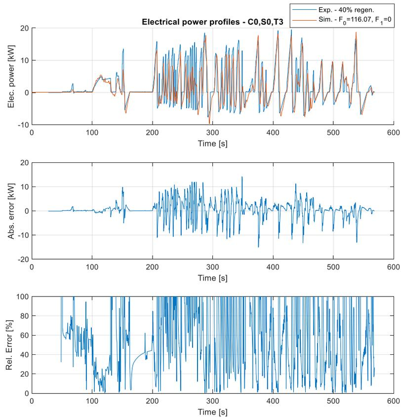
Figure 80. Electrical power profile and its error simulated with C0,S0,T3
