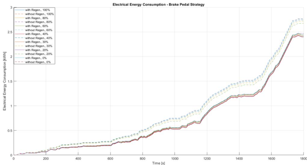
Figure 40. All the electrical energy consumption profiles simulated with brake pedal strategy – WLTP Class 3 cycle
