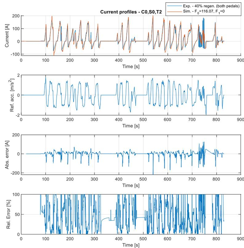
Figure 74. Current profile and its error simulated with C0,S0,T2
