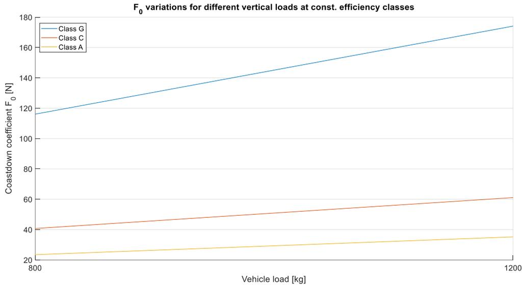
Figure 55.  $F_0$  variations for different vertical loads at constant efficiency classes
