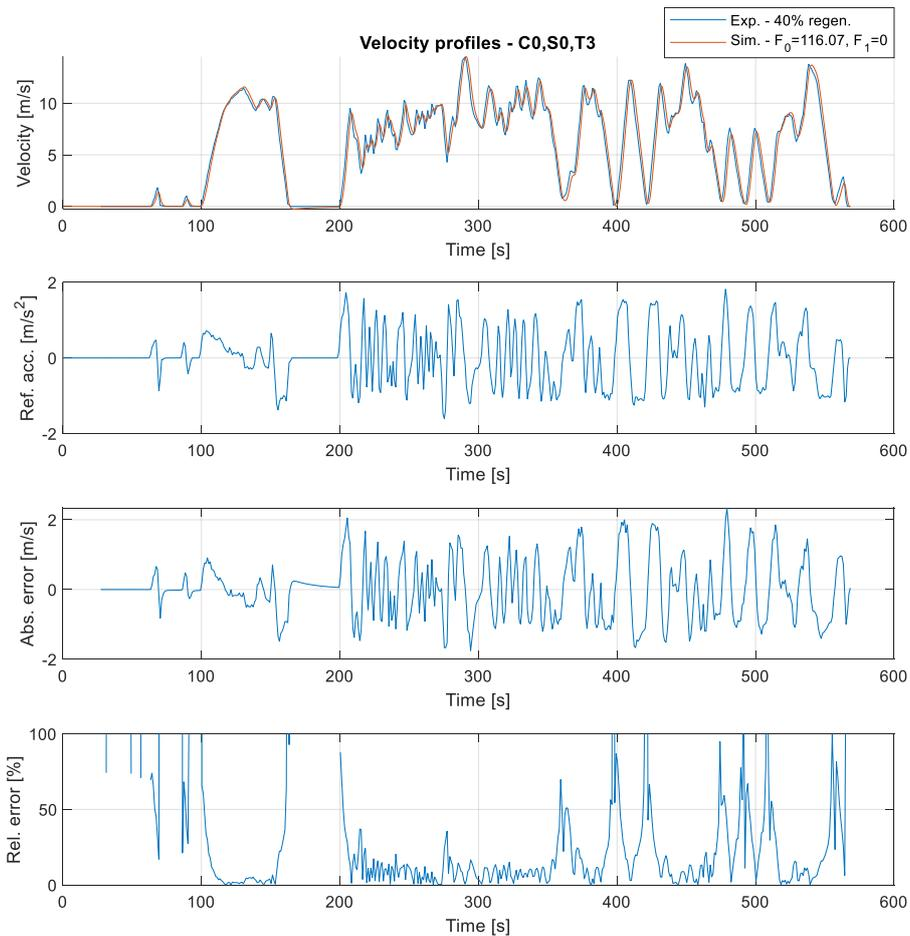
Figure 78. Velocity profile and its error simulated with C0,S0,T3
