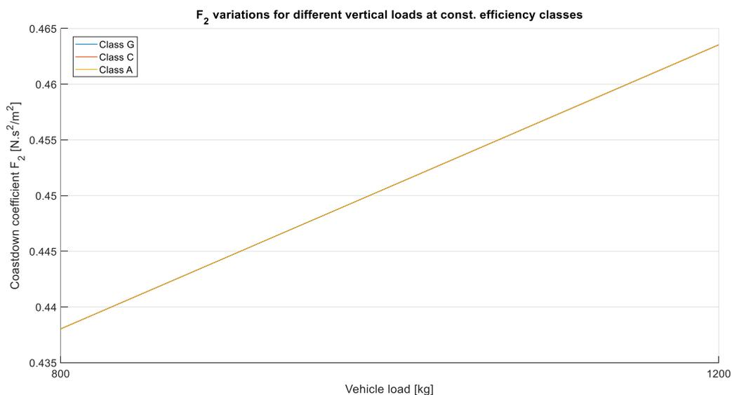
Figure 56.  $F_2$  variations for different vertical loads at constant energy efficiency classes
