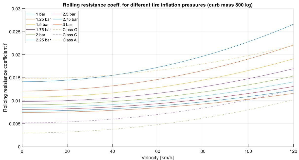
Figure 48. Rolling resistance coefficient for different tire inflation pressures at fixed vertical load (800kg)
