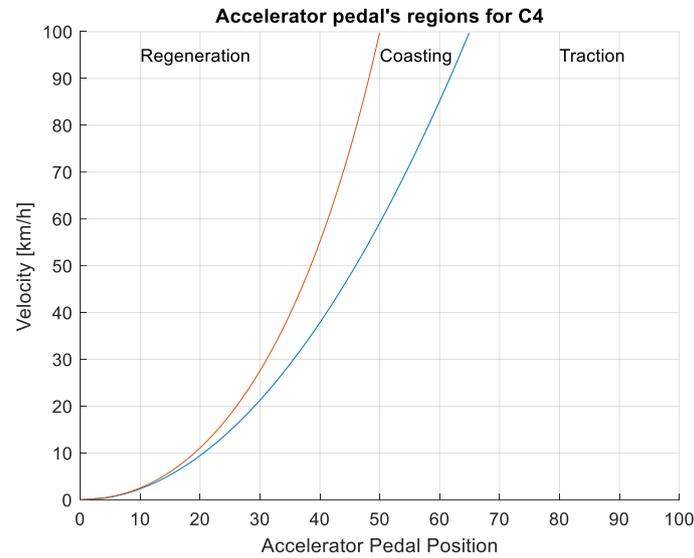
Figure 164. Variation of regeneration, coasting and traction regions over the velocity range of the vehicle with C4 strategy
