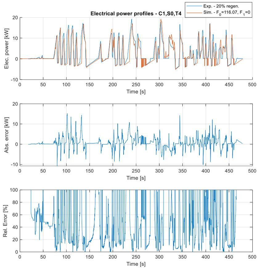
Figure 105. Electrical power profile and its error simulated with C1,S0,T4
