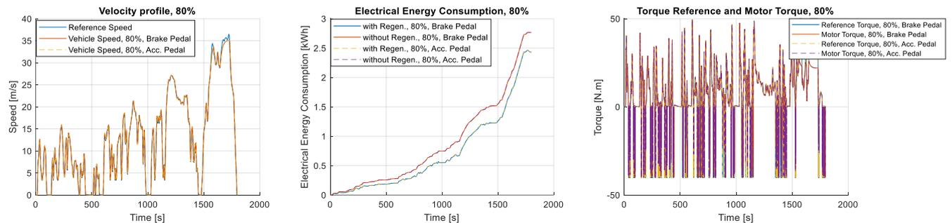
Figure 32. 80% on/off regenerative braking with both pedal strategy – WLTP Class 3 cycle
