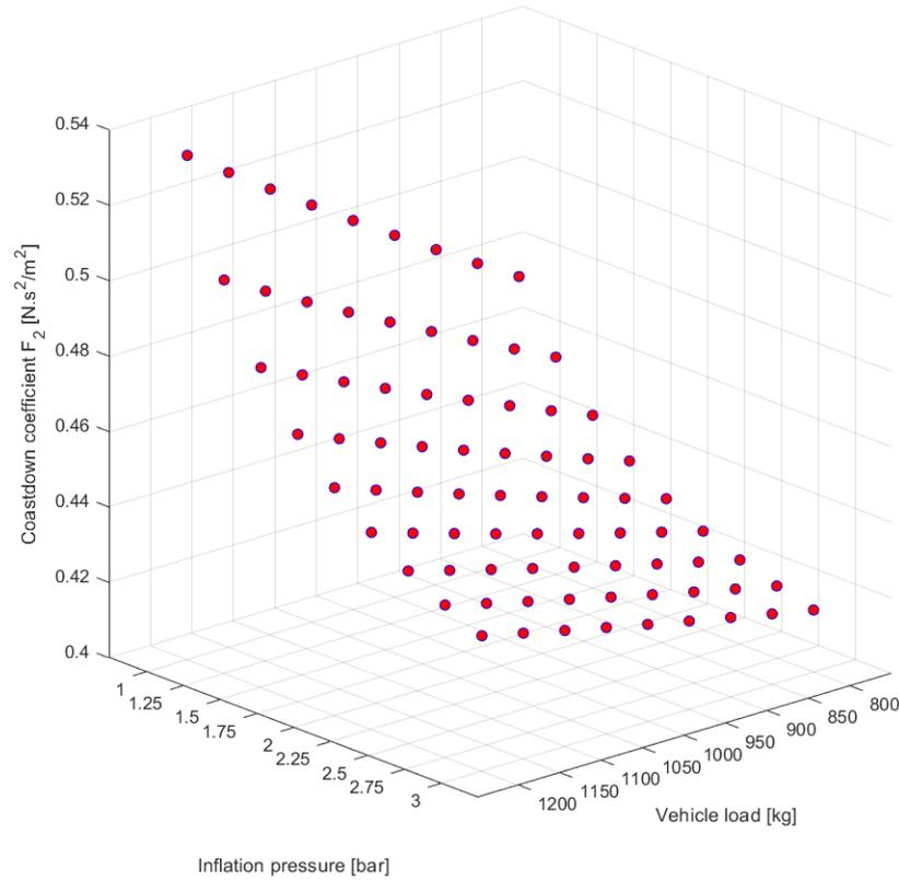
Figure 50.  $F_2$  for different combinations of vehicle load and inflation pressure
