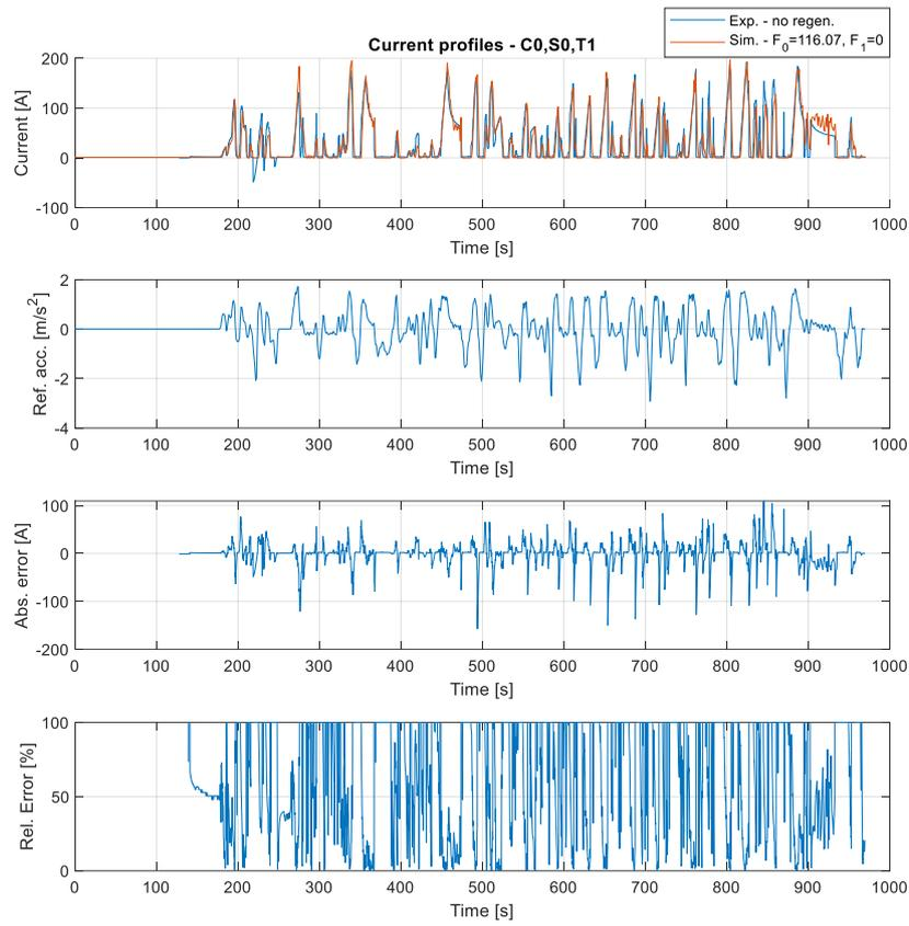
Figure 69. Current profile and its error simulated with C0,S0,T1
