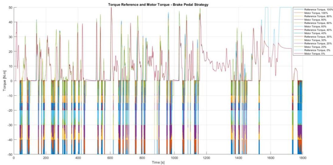
Figure 39. All the torque profiles simulated with brake pedal strategy – WLTP Class 3 cycle
