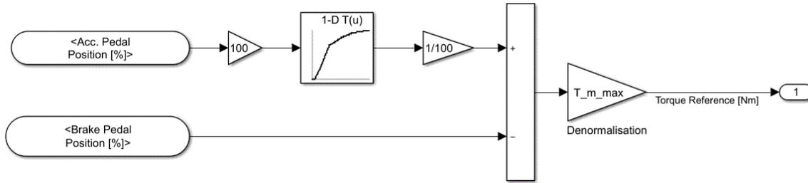
Figure 10. Simulink implementation of the accelerator pedal map
