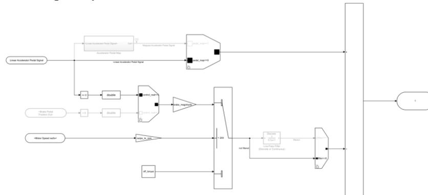
Figure 17. Simulink implementation of on/off regenerative braking with accelerator pedal strategy
