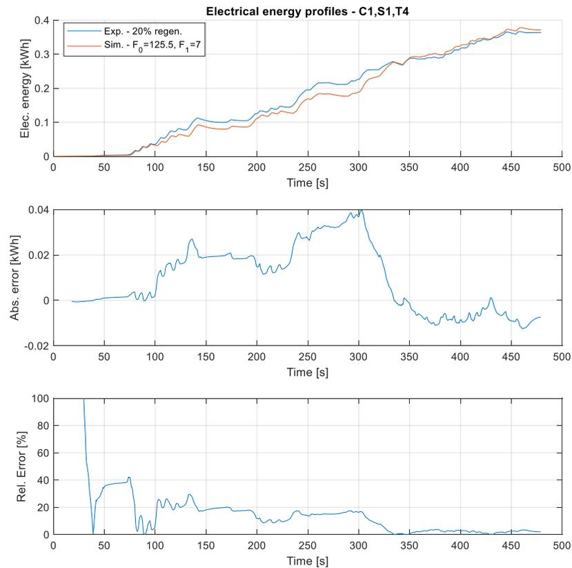
Figure 126. Electrical energy profile and its error simulated with C1,S1,T4
