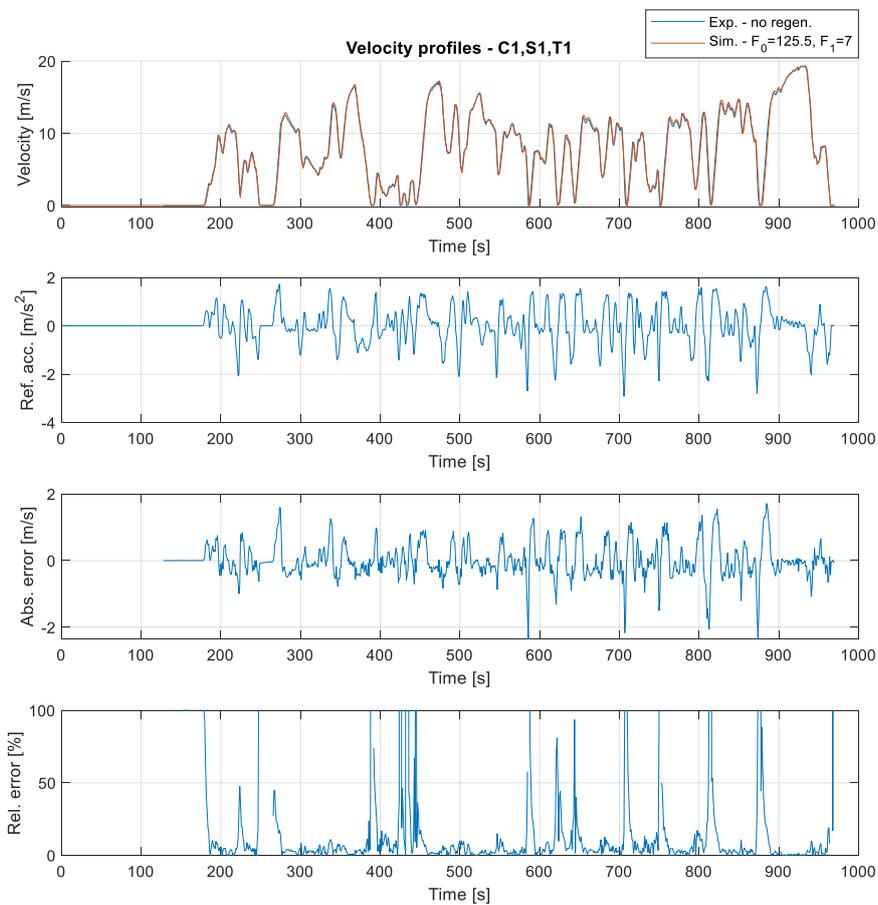
Figure 108. Velocity profile and its error simulated with C1,S1,T1
