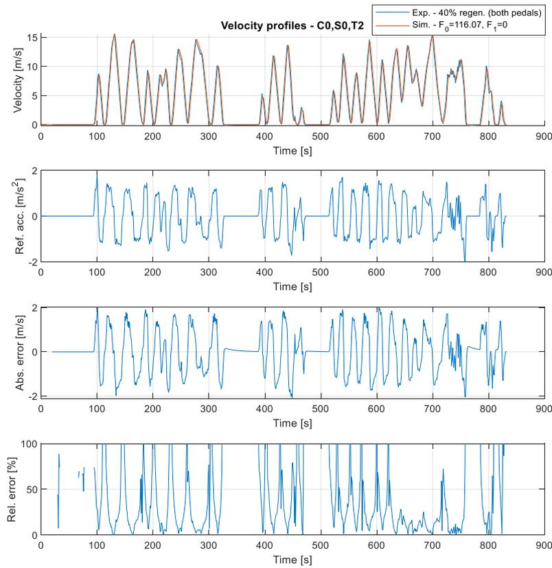
Figure 73. Velocity profile and its error simulated with C0,S0,T2
