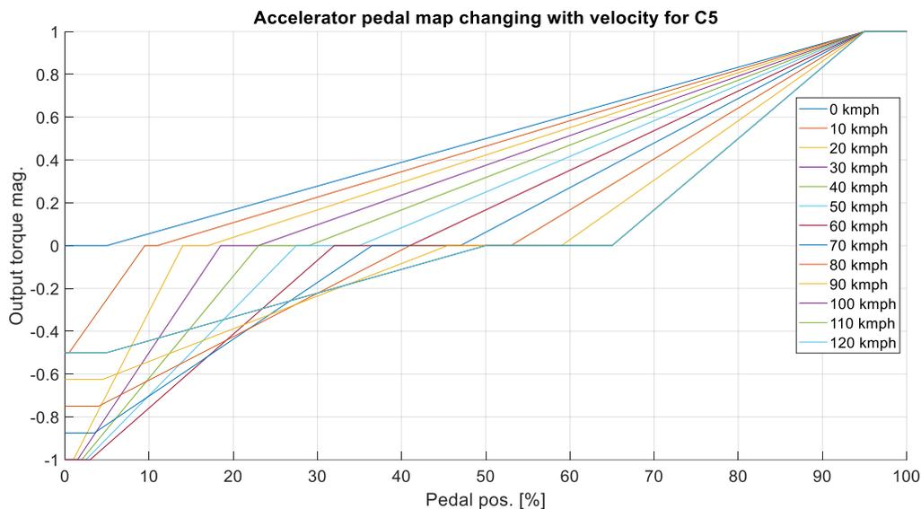
Figure 168. Accelerator pedal map changing with velocity in C5
