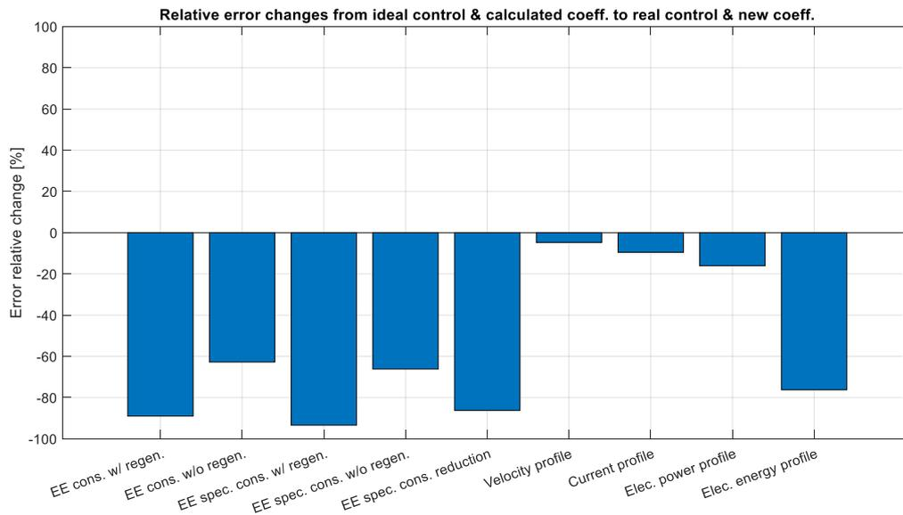
Figure 152. Overall relative error changes moving from original model to the new one with tuned coeff. and real control
