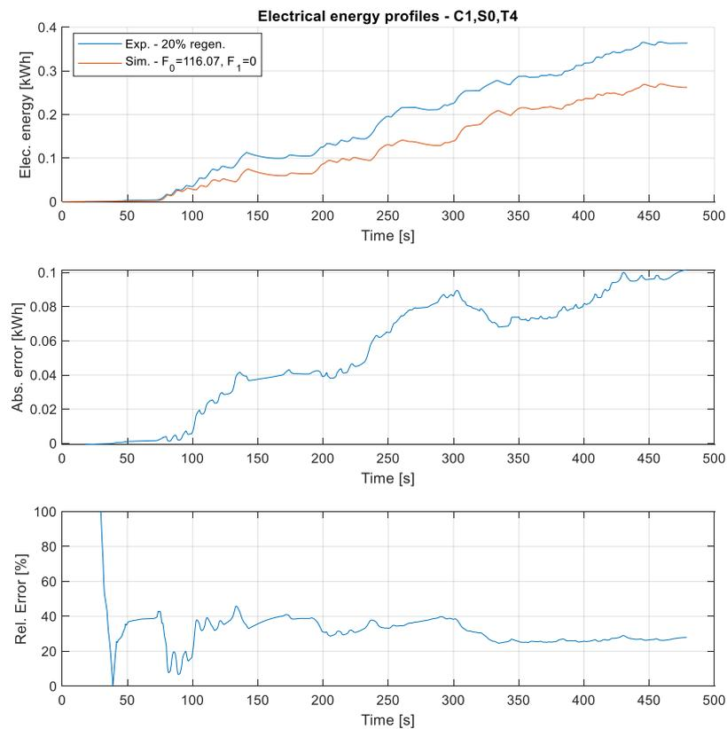
Figure 106. Electrical energy profile and its error simulated with C1,S0,T4
