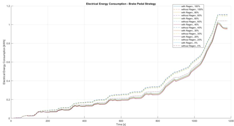
Figure 27. All the electrical energy consumption profiles simulated with brake pedal strategy – NEDC cycle
