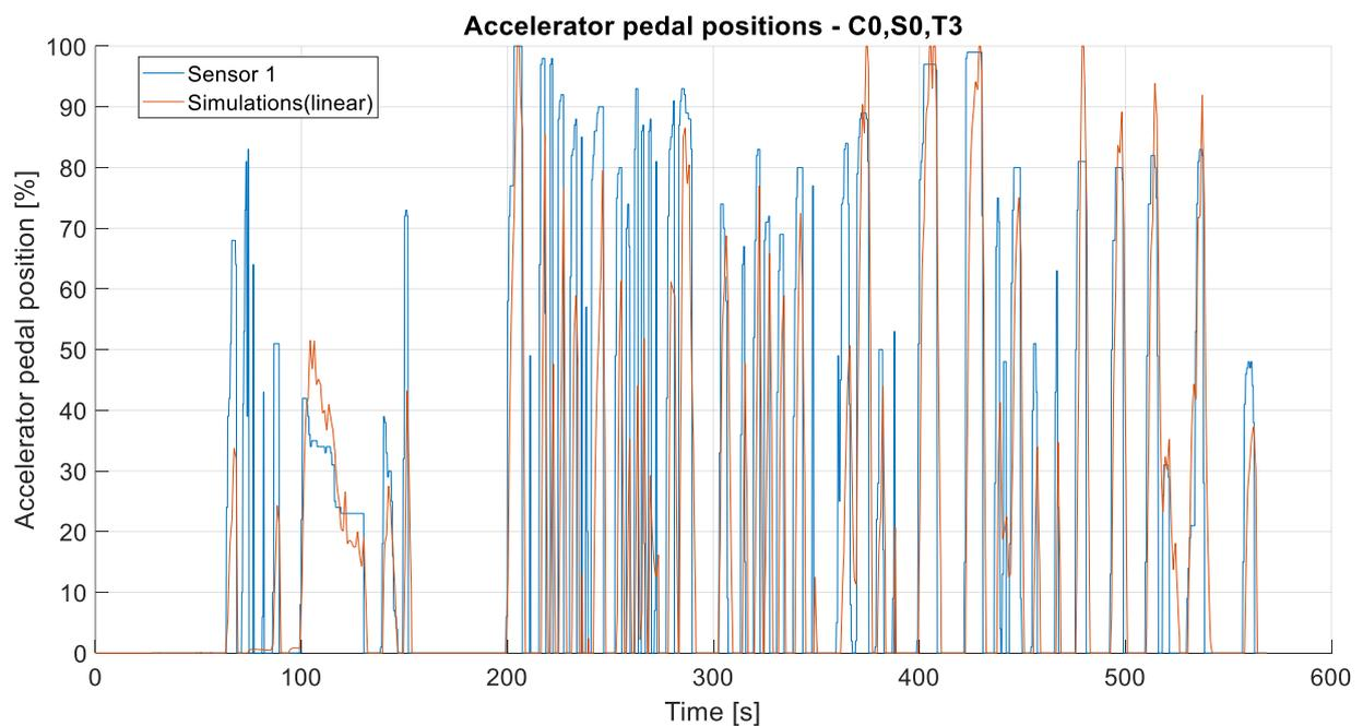
Figure 82. Accelerator pedal positions simulated with C0,S0,T3
