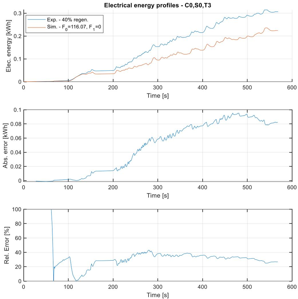
Figure 81. Electrical energy profile and its error simulated with C0,S0,T3
