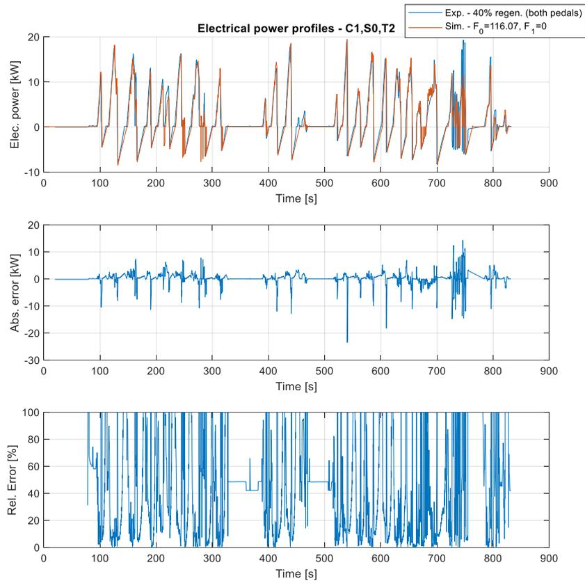
Figure 95. Electrical power profile and its error simulated with C1,S0,T2
