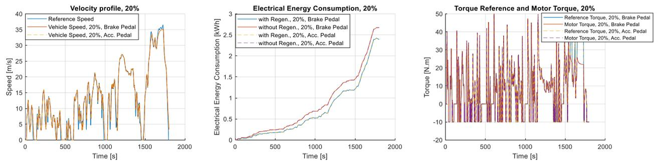
Figure 36. 20% on/off regenerative braking with both pedal strategy – WLTP Class 3 cycle
