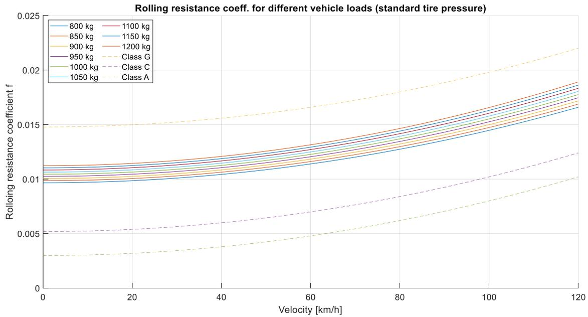
Figure 47. Rolling resistance coefficient for different vertical loads at fixed 1.8 [bar] tire inflation pressure
