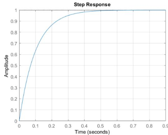
Figure 64. Step response of the low pass filter implemented in Simulink model of the real control system C1
