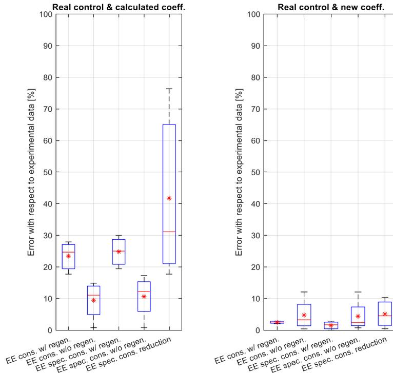
Figure 141. Distribution of consumption errors reported in box plots – C1,S0 vs. C1,S1
