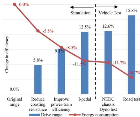
Figure 7. Road map of energy consumption and drive range changes obtained in [4]
