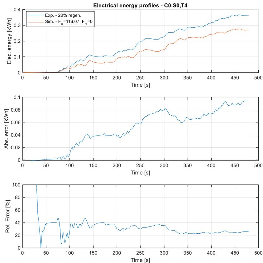
Figure 86. Electrical energy profile and its error simulated with C0,S0,T4
