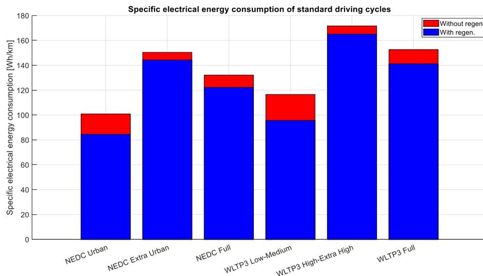
Figure 153. Specific electrical energy consumption of standard driving cycle
