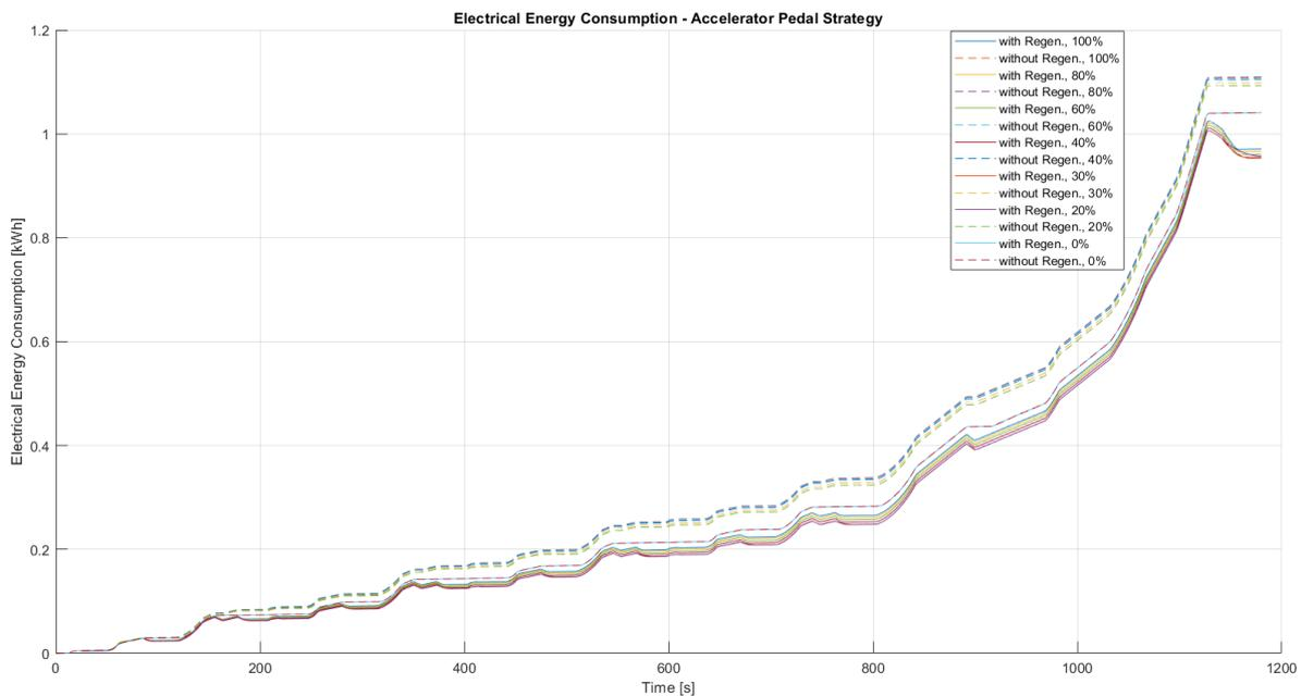
Figure 30. All the electrical energy consumption profiles simulated with accelerator pedal strategy – NEDC cycle
