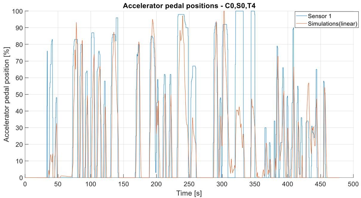
Figure 87. Accelerator pedal positions simulated with C0,S0,T4
