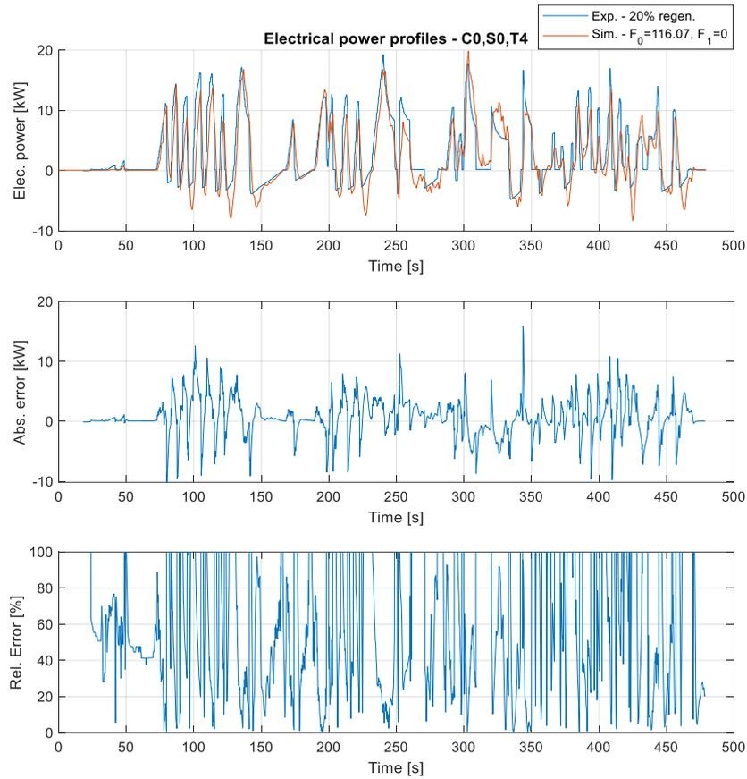
Figure 85. Electrical power profile and its error simulated with C0,S0,T4
