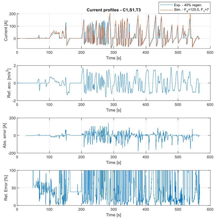
Figure 119. Current profile and its error simulated with C1,S1,T3
