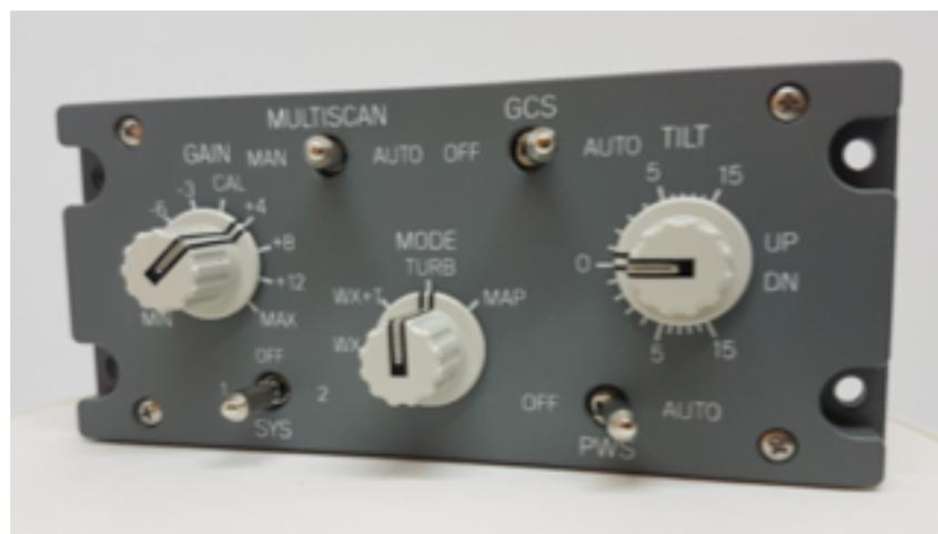
**Figura 54 - Weather Radar Control Panel.<sup>77</sup>**
