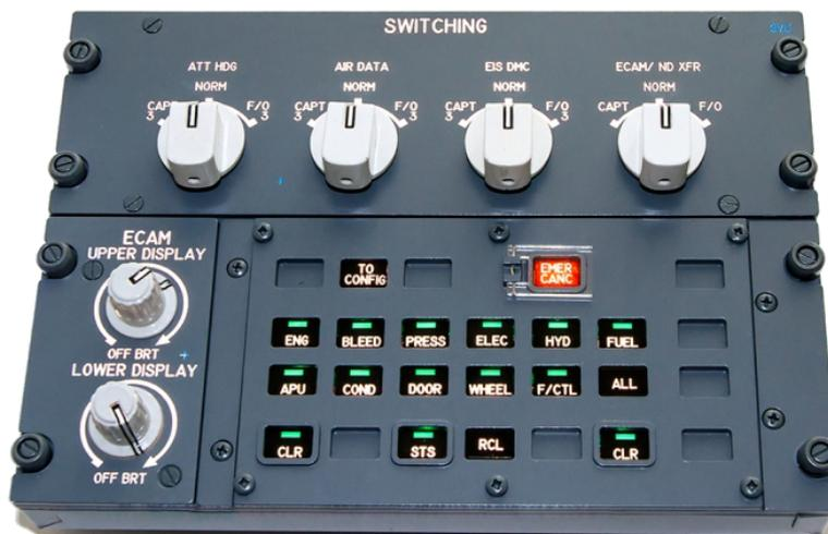
**Figura 51 – ECAM Panel e Multipurpose Switching Panel del velivolo A320.<sup>73</sup>**
