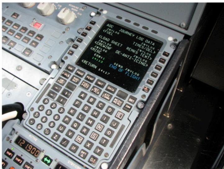
**Figura 50 - Multipurpose Control Display Unit del velivolo A320.<sup>71</sup>**
