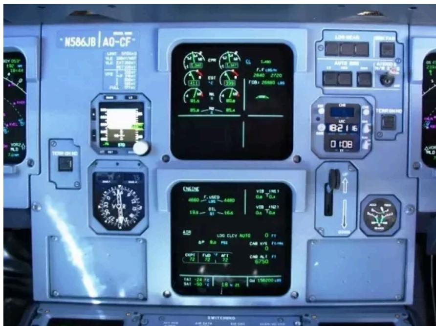
**Figura 43 - Electronic Centralized Aircraft Monitoring Displays.<sup>61</sup>**
