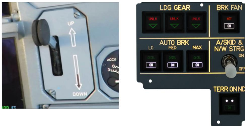
**Figura 44 - Landing Gear Lever (a sinistra)<sup>62</sup>
