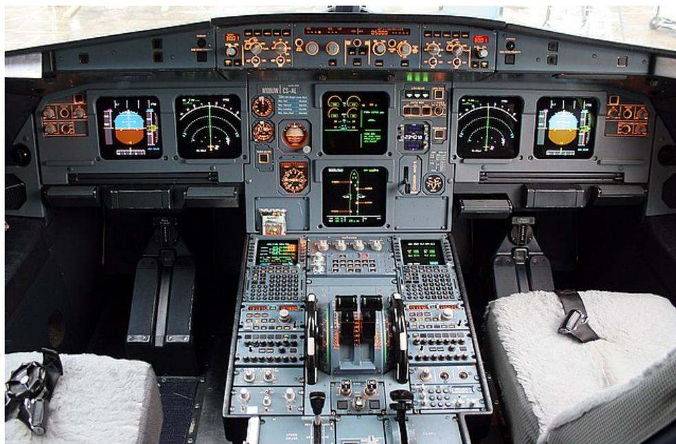
Figura 40 - *Glass Cockpit* del velivolo Airbus A320.<sup>54</sup>
