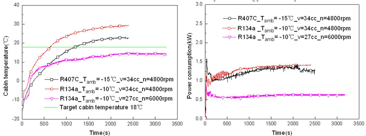
Fig: (a) Variation of the cabin temperature under different heating conditions; (b) Variation of the compressor power consumption [38]
