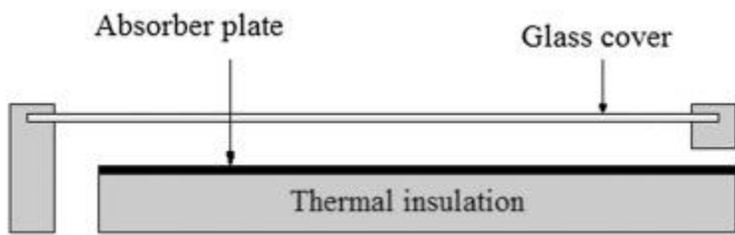
Figure 2 Solar chimney
