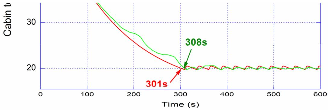
Fig. 5 Validation of cabin temperature variation with reference (33)
