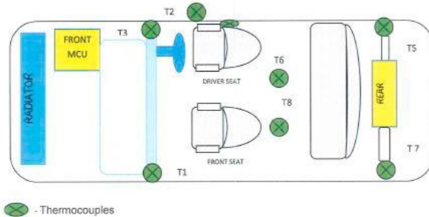
Figure 3 Thermocouples representation [35]
