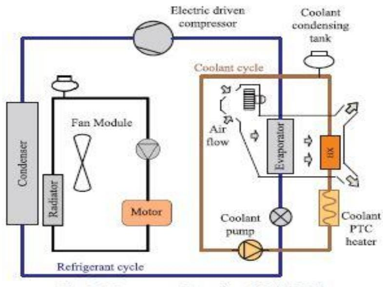
Figure 1 AC system configuration of i-MiEV
