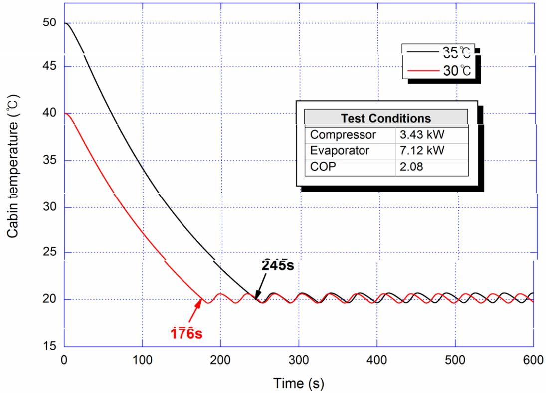
The above figure shows the experimental results of simulation of the ambient temperature of 40 and 50 °C since there were no comparable experimental results for 35 and 30 °C. It takes 176 and 245 seconds from 40 and 50 °C respectively to reach the targeted temperature. Once the target temperature is achieved, the cabin temperature is maintained.
