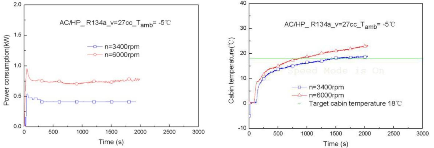
Fig (a) Variation of the cabin temperature under different compressor speeds;(b) Variation of the compressor power consumption [38]
