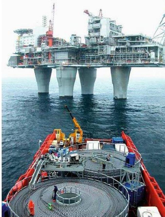
*Figure 3 Submarine power cables supplying gas platform [1]*
