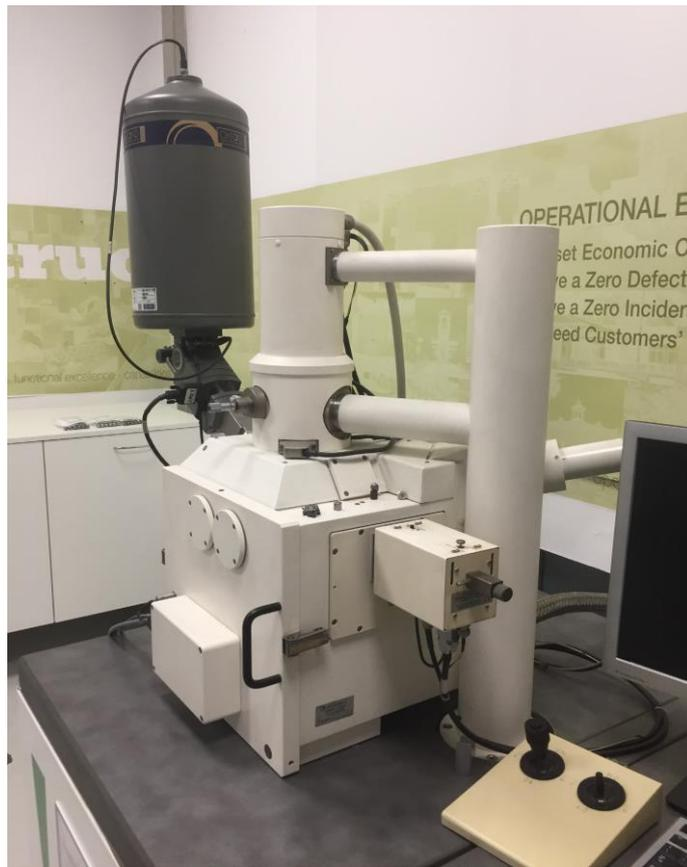
Figure 4.13 – Scanning electron microscope
