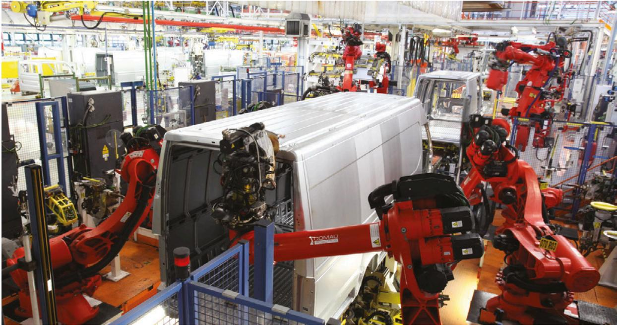
Figure 10: A digital twin of the Iveco manufacturing line helps drive better automated welding capabilities. Source: AnyLogic
