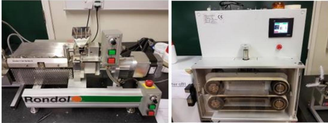
Figure 27: Left: Rondol 10mm Twin Screw Mini Extruder. Right: Rondol Haul-Off.
