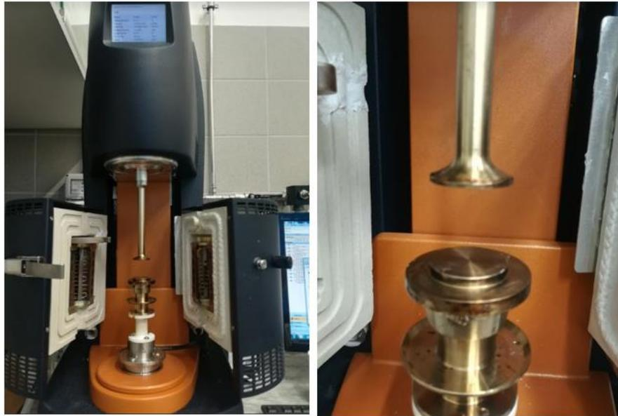
Figure 38: Left: DHR-2 rotational rheometer. Right: Detail of the 25 mm parallel plate geometry.
