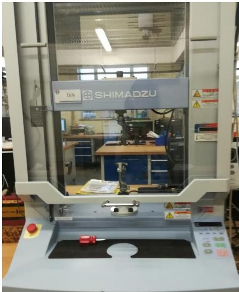
Figure 33: Shimadzu 1kN testing machine in G15 laboratory.
