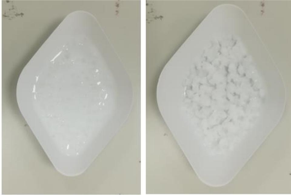
Figure 25: Pellets production. Left: PLLA mixed with HA suspension. Right: dried pellets.
