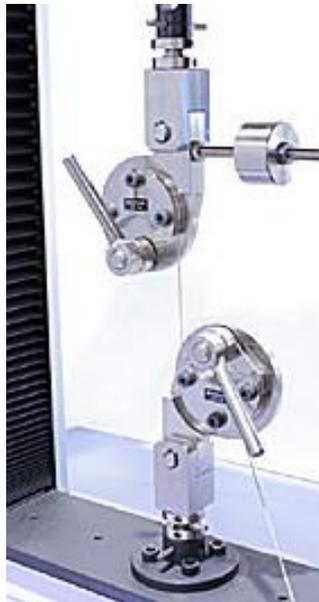
*Figure 35: Example of the grip used to hold the filaments.<sup>121</sup>*
