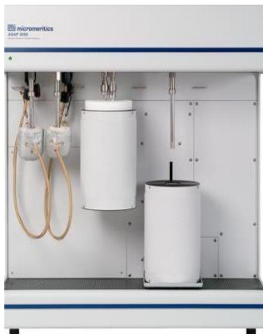
Figure 29: ASAP2020 from Micromeritics for  $N_2$  adsorption-desorption analysis.
