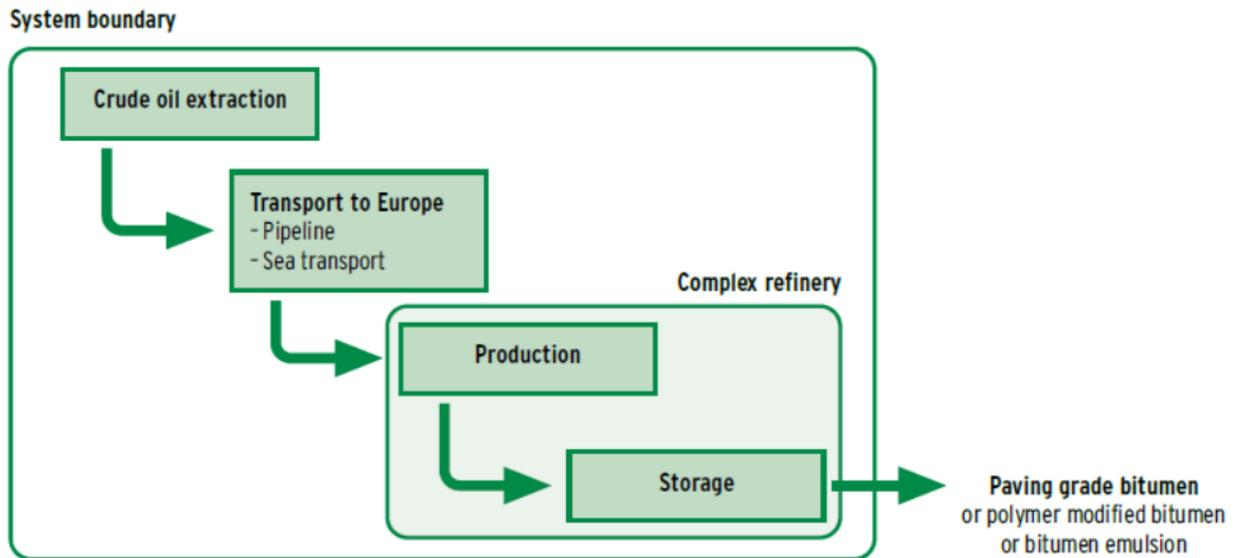
Figure 31. System boundaries for the bitumen eco-profile (cradle-to-gate approach).
