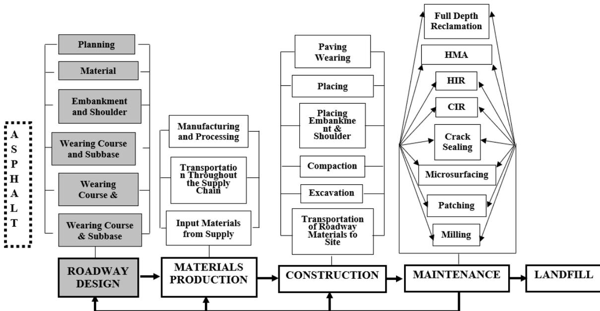
Figure 19. Example of asphalt construction life-cycle.
