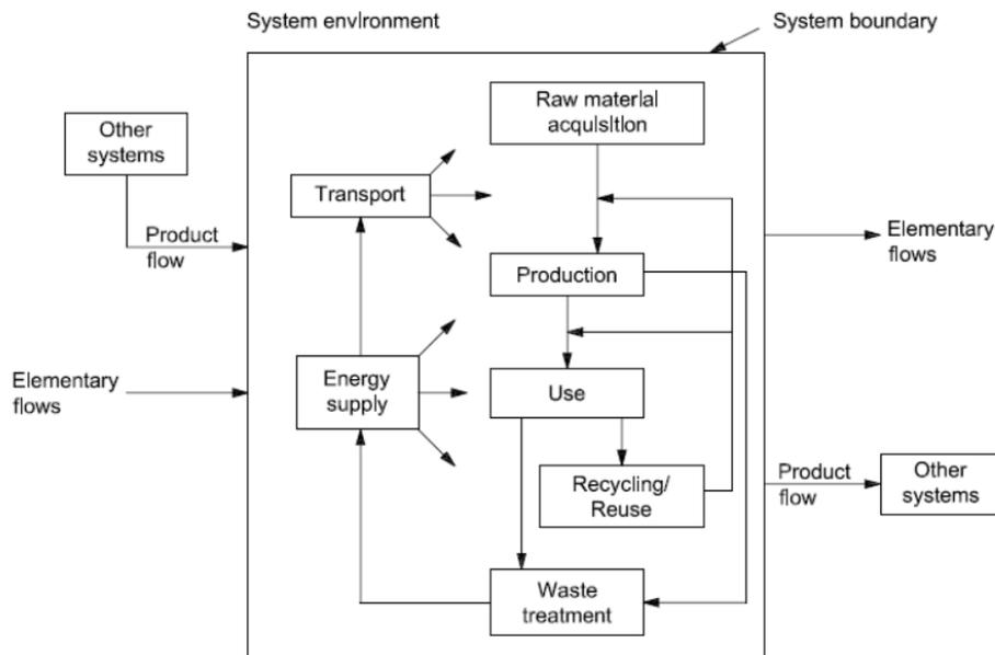
Figure 5. Example of a product system for LCA (Iso, 2004).
