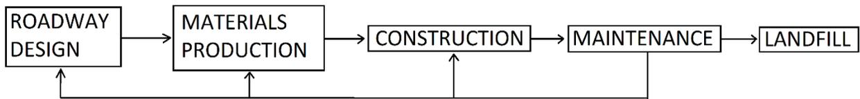
Figure 7. Life cycle of a pavement considered by PaLATE.
