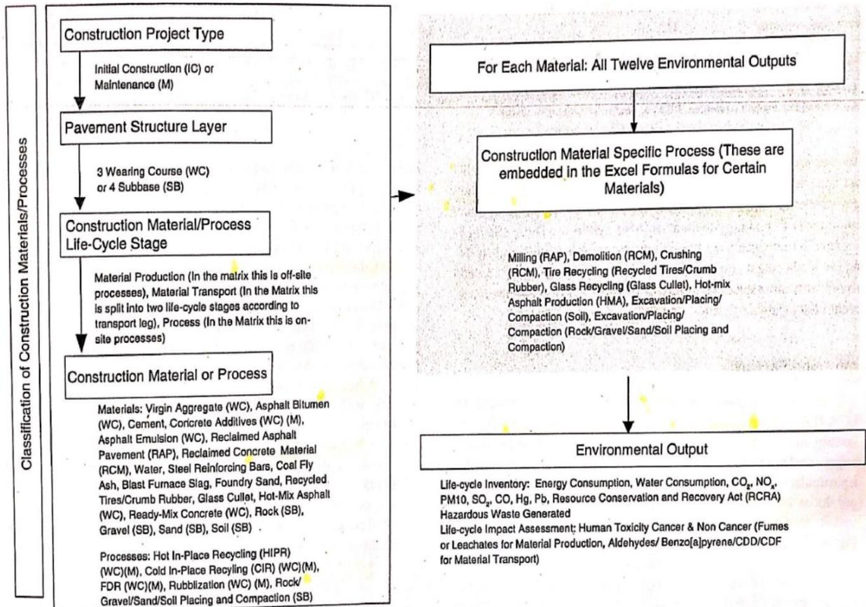
Figure 23. How PaLATE arrives to environmental calculations (Nathman et al., 2009).
