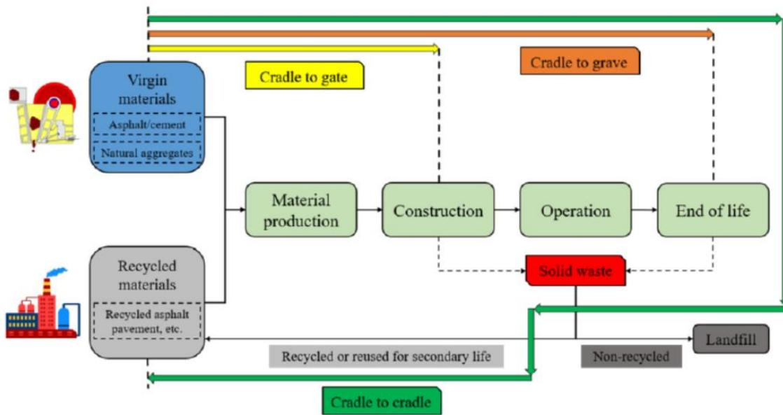
Figure 2. Diagram of three pavement LCAs (Li et al., 2019).
