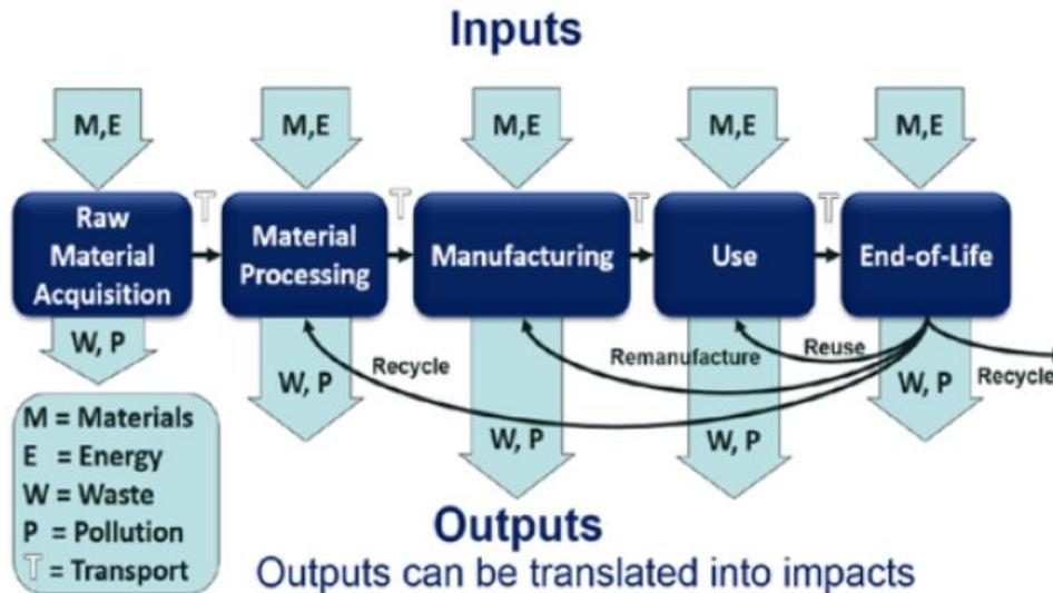
Figure 1. Generic life cycle of a production system for LCA (Federal Highway Administration (FHWA), 2014).
