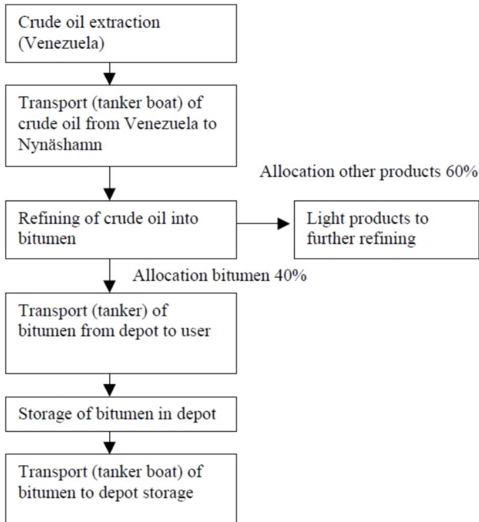
Figure 32. Overview of a model structure for production of bitumen (Stripple, 2001).
