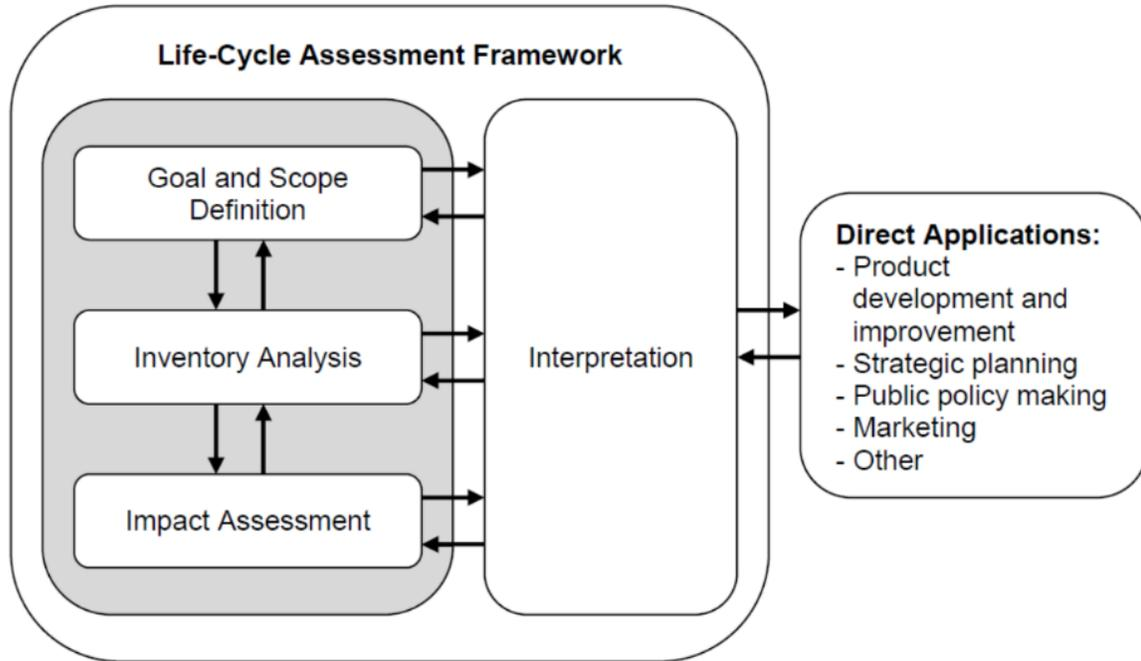
Figure 3. Basic LCA framework (Santero et al., 2010).
