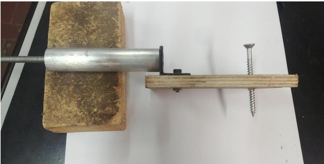
*Figure 6.1: Simple tool used to simulate and measure the force required to tear the cloth*
