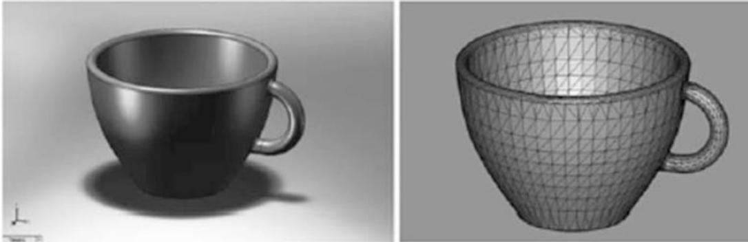
Figure 11) CAD model converted into STL format [2]
