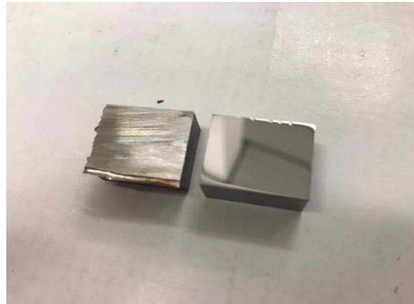
Figure 71) sample after cutting on the left and after polishing on the right
