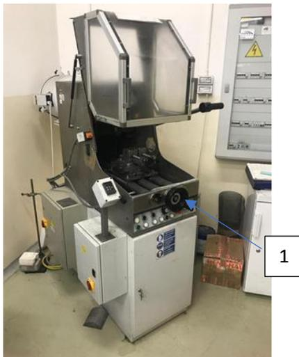
Figure 60) cutting machine with positioning system (1)
