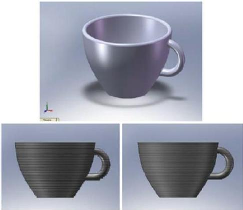
Figure 3) example of a model divided into layers [2]
