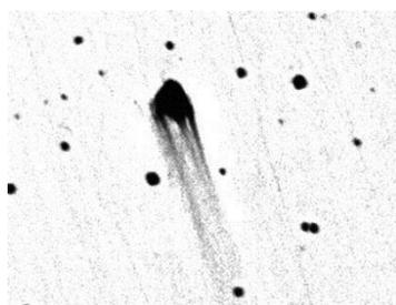
*Figure 74) pore's wake created by polishing*
